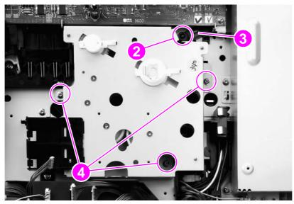
Figure 89. Feed-drive assembly
