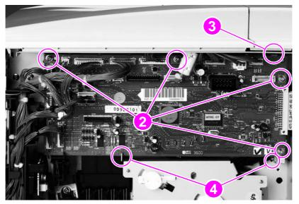
Figure 85.DC controller (2 of 2)
