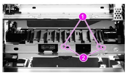
Figure 73. Transfer-guide assembly
