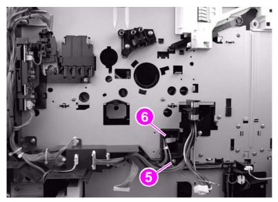
Figure 97. Fuser-connector holder assembly (3 of 3)
