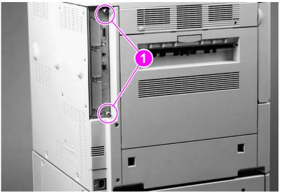
Figure 79. Formatter (HP LaserJet 9000 shown)
