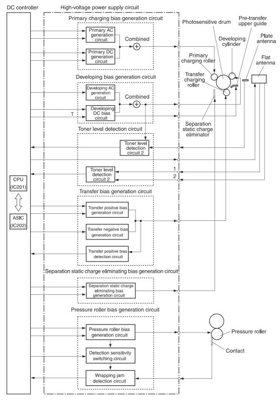
Figure 26. High-voltage power supply block diagram
