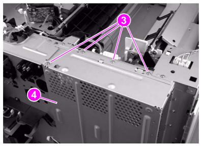
Figure 96. Fuser-connector holder assembly (2 of 3)
