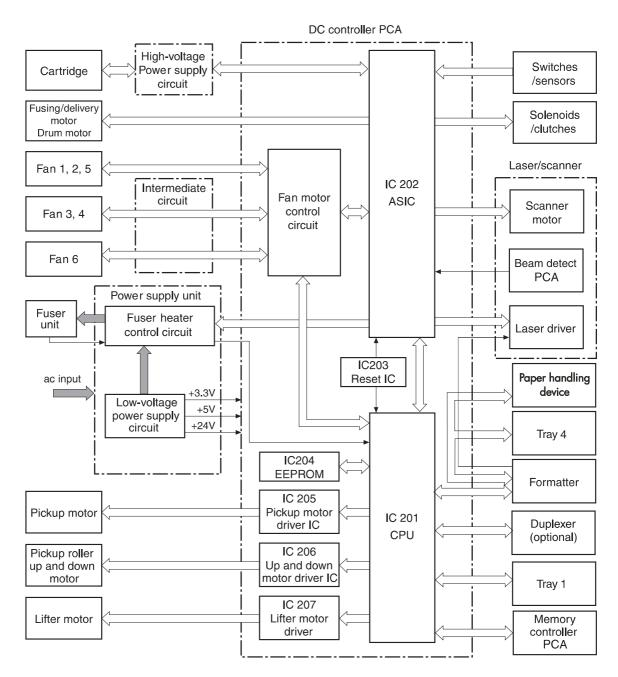
Figure 25. DC controller PCA block diagram
