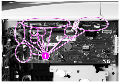
Figure 84. DC controller (1 of 2)
