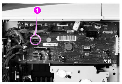
Figure 71. Registration assembly (1 of 2)
