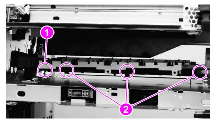
Figure 74. Reinstalling the transfer-guide assembly
