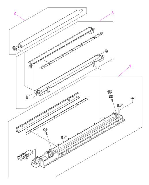
Figure 147. Transfer roller assembly
