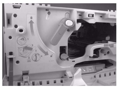
Figure 58. Cartridge release lever (3 of 3)
