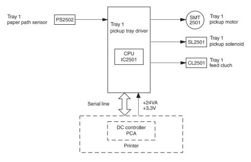
Figure 33. Tray 1 block diagram
