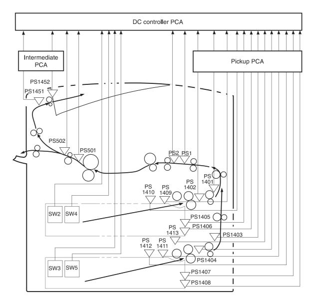
Figure 31. Pickup-and-feed system sensors and switches
