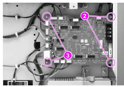
Figure 111. Controller board (2 of 2)
