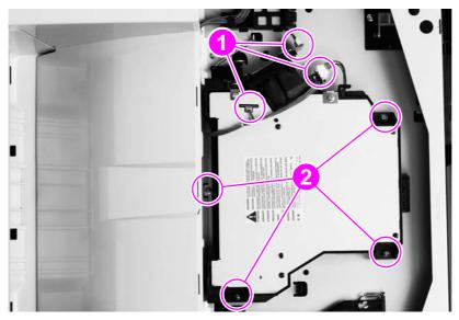
Figure 50. Laser/scanner assembly
