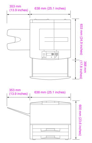
Figure 6. Space requirements for the base model
