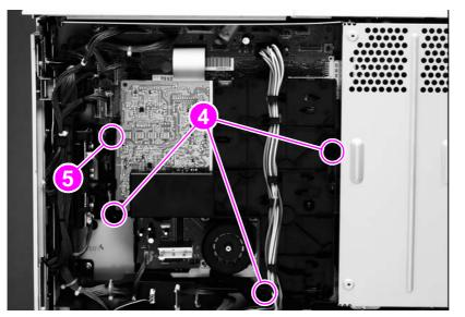
Figure 83.High-voltage power supply (2 of 2)
