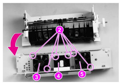
Figure 54. Delivery-assembly fans and face-down-bin fan (2 of 2)
