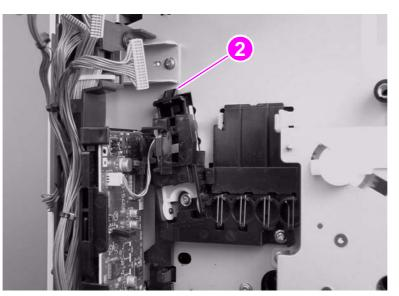
Figure 87.Reinstalling the toner-sensor contact assembly
