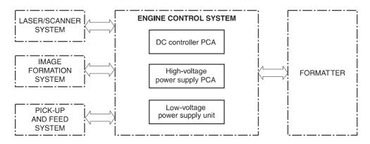
Figure 24. Engine-control-system block diagram
