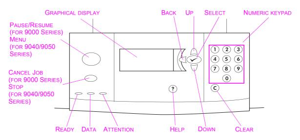
Figure 11. Control-panel layout
