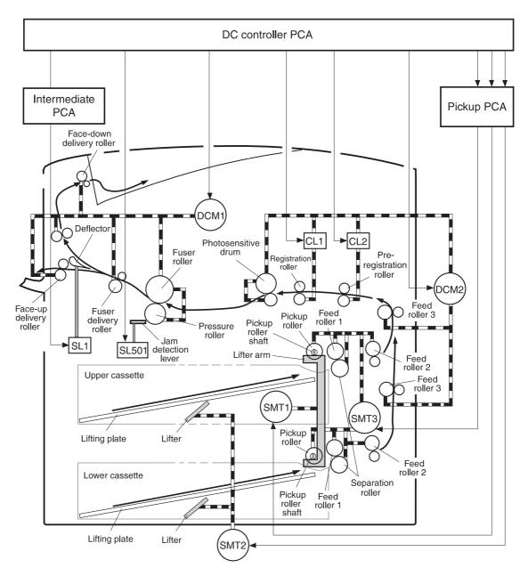
Figure 32. Pickup-and-feed system motors and solenoids
