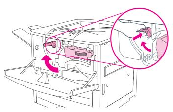
Figure 18.Lock the print cartridge
