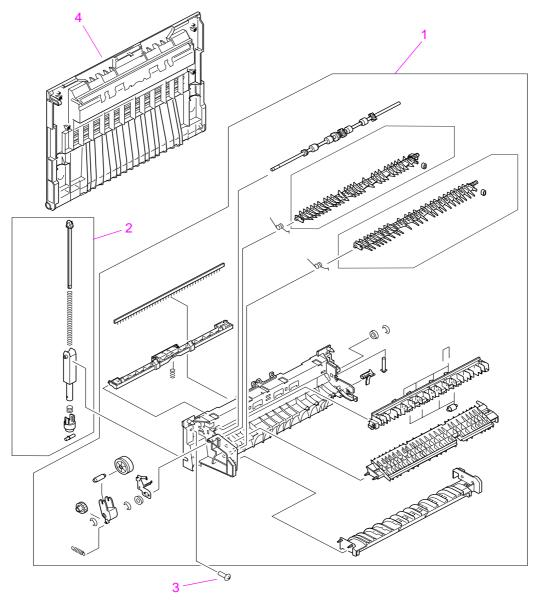
Figure 135. Left door and diverter
