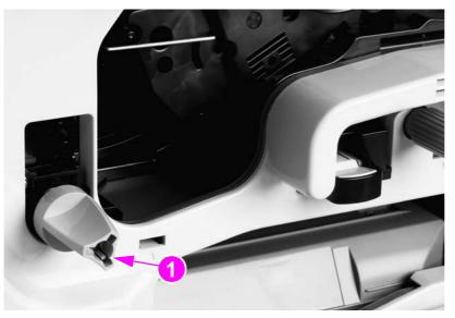
Figure 63. Fuser-jam-removal knob
