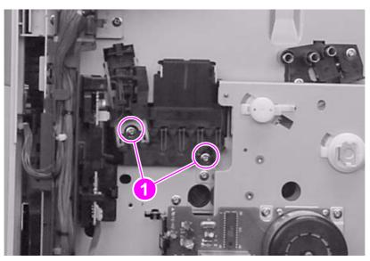
Figure 86. Toner-sensor contact assembly
