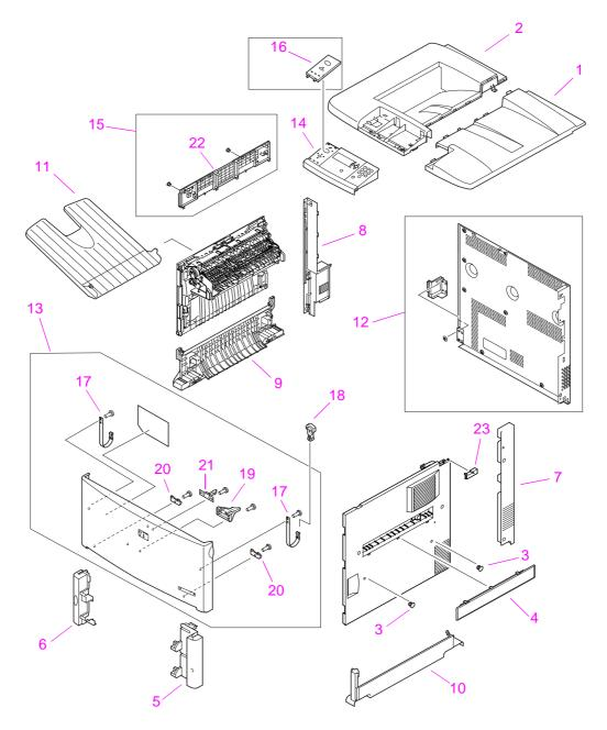
Figure 134. Printer external covers and panels
