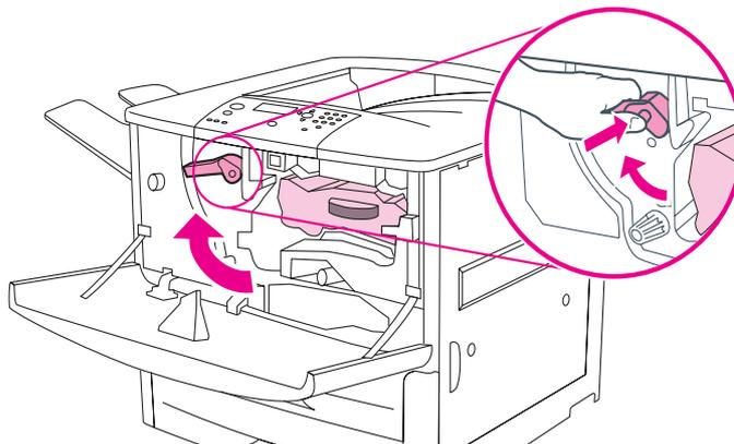
**Figure 18.** Lock the print cartridge
