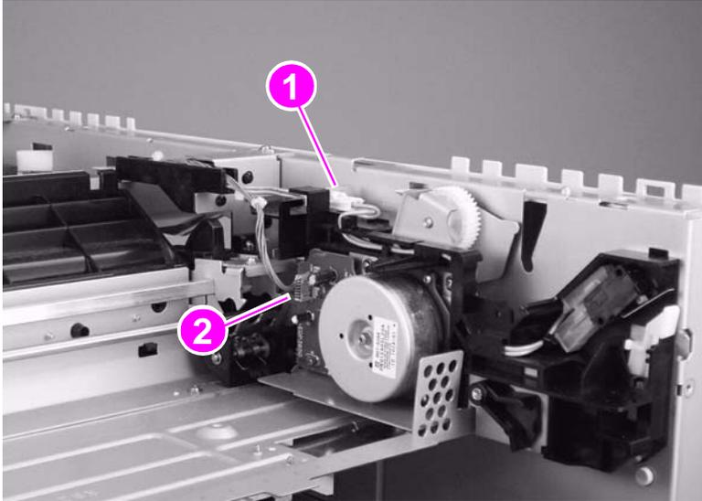
**Figure 98.** Fuser delivery-drive assembly (1 of 3)
