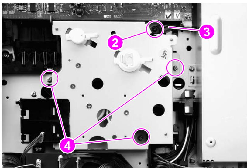
**Figure 89.** Feed-drive assembly
