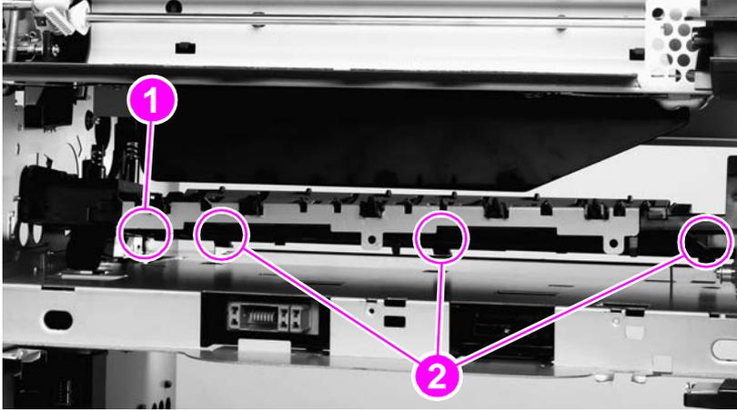
**Figure 74.** Reinstalling the transfer-guide assembly
