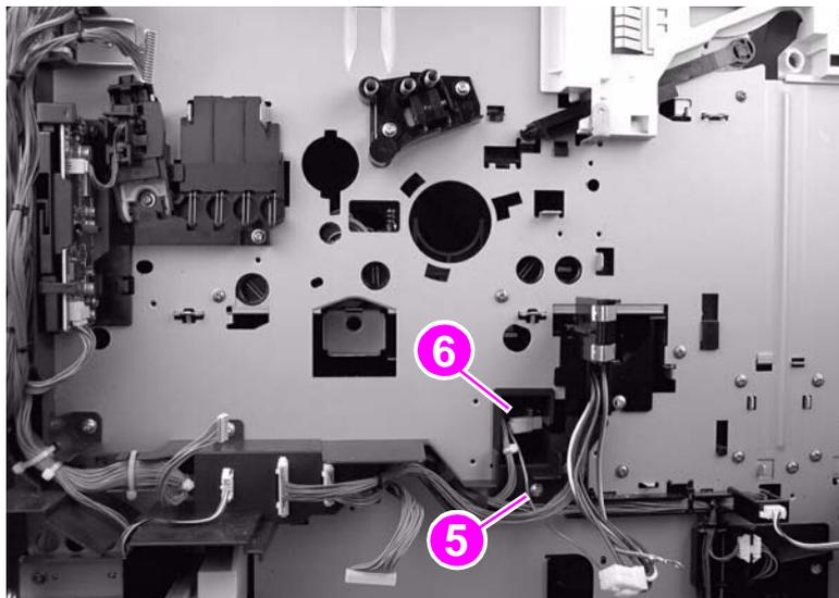
**Figure 97.** Fuser-contractor holder assembly (3 of 3)
