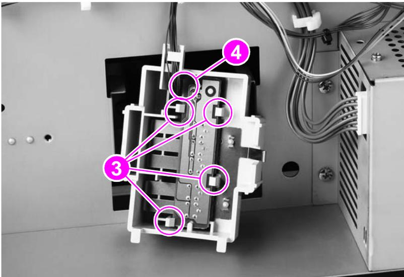
Figure 113. Paper-size switch PCA (2 of 2)
