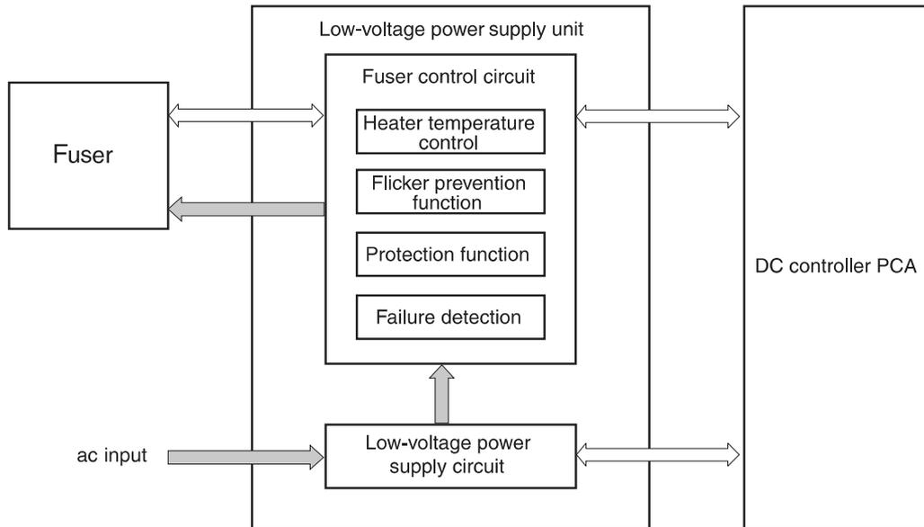
**Figure 27.** Power-supply-block diagram
