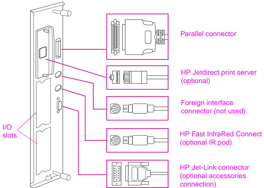
**Figure 4.** Interface connections (HP LaserJet 9000 Series printer)
