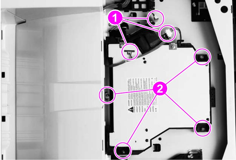
**Figure 50.** Laser/scanner assembly
