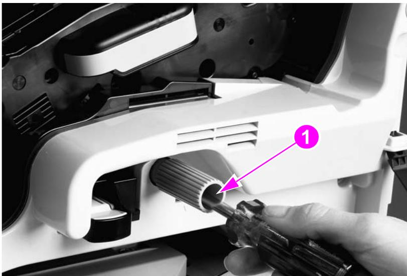
**Figure 64.** Registration-jam-removal knob
