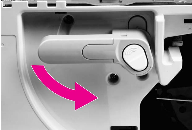
**Figure 56.** Cartridge release lever (1 of 3)
