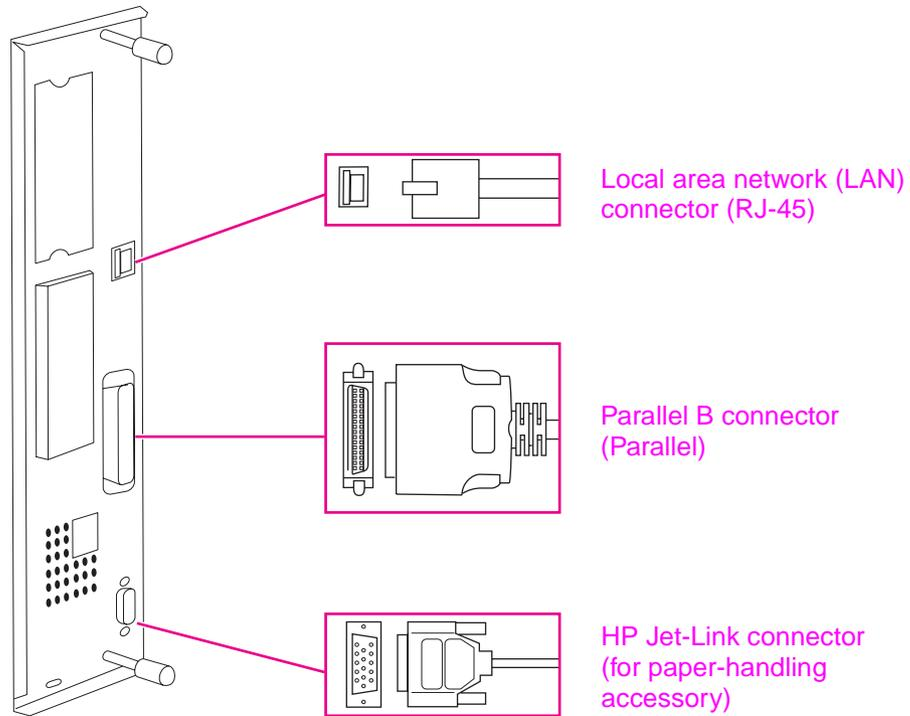
**Figure 3.** Interface connections (HP LaserJet 9040/9050 Series printer)
