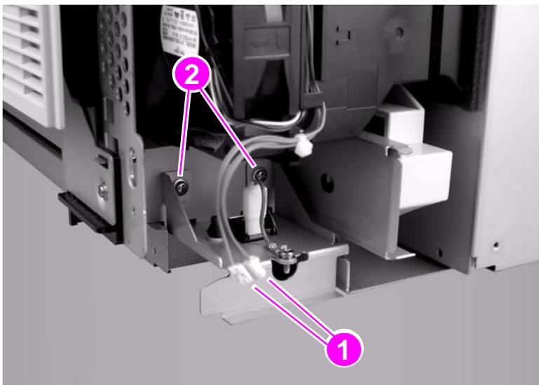
**Figure 94.** Jetlink connector
