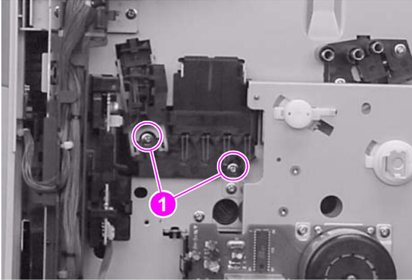
**Figure 86.** Toner-sensor contact assembly
