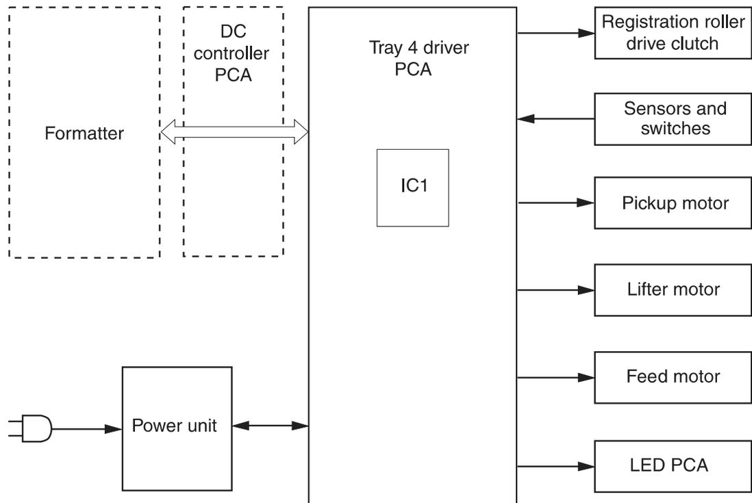
Figure 34. Tray 4 block diagram
