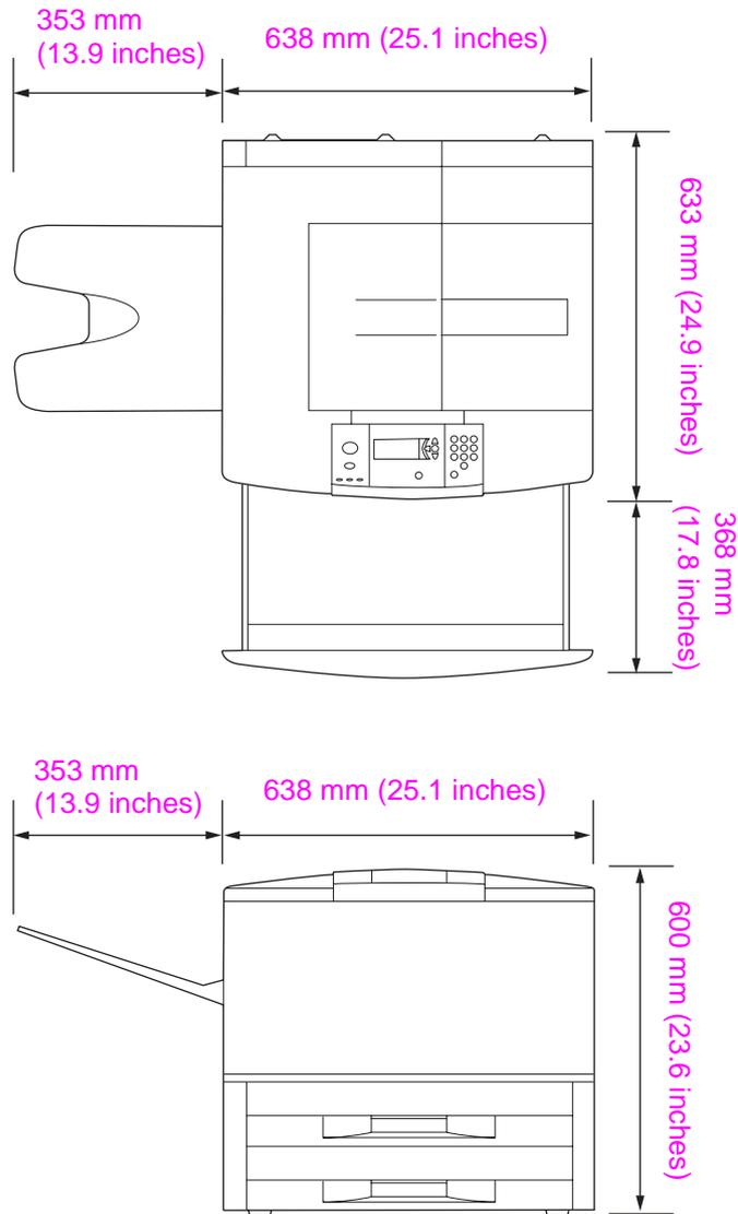
**Figure 6.** Space requirements for the base model
