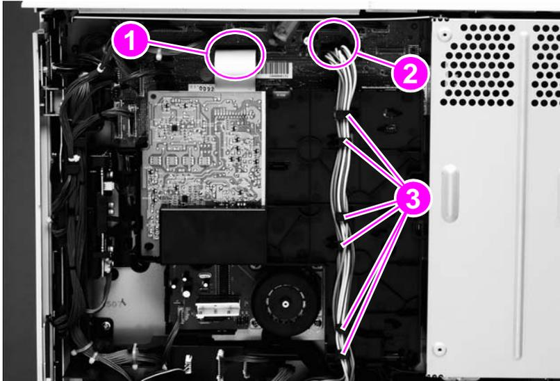
**Figure 82.** High-voltage power supply (1 of 2)
