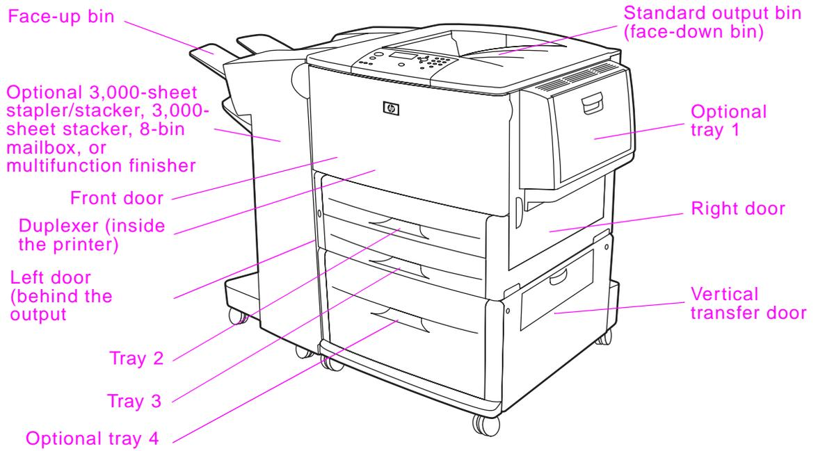
**Figure 2.** External view of the printer and accessories
