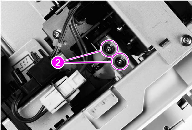
**Figure 57.** Cartridge release lever (2 of 3)
