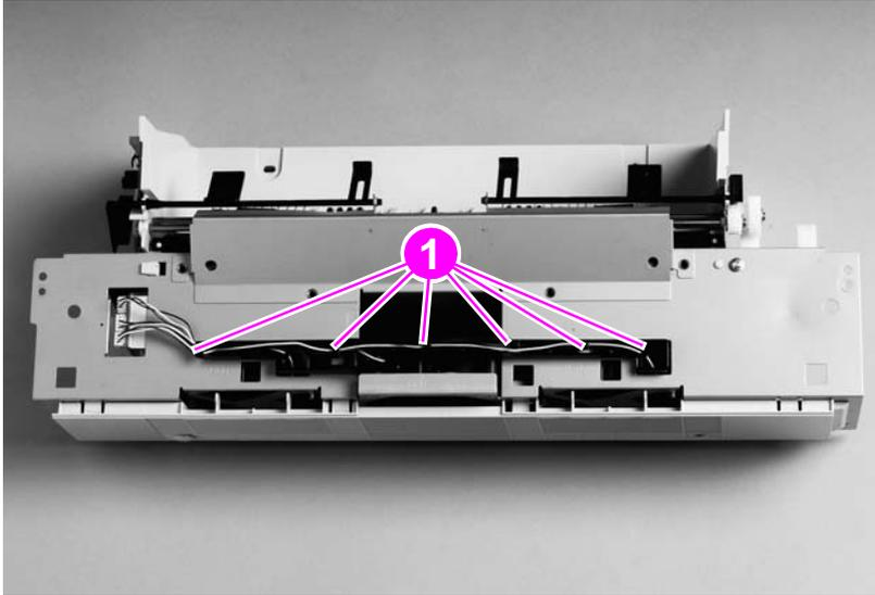
**Figure 53.** Delivery-assembly fans and face-down-bin fan (1 of 2)
