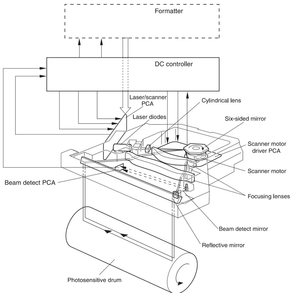
**Figure 28.** Laser/scanner system
