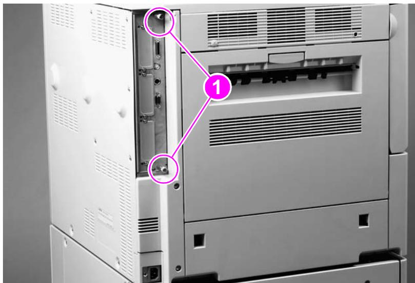
**Figure 79.** Formatter (HP LaserJet 9000 shown)
