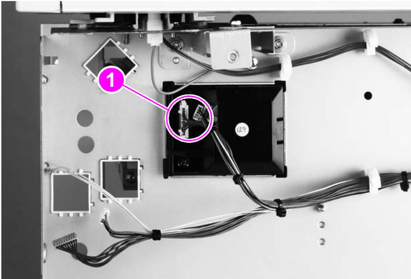
**Figure 115.** Pickup assembly (1 of 2)
