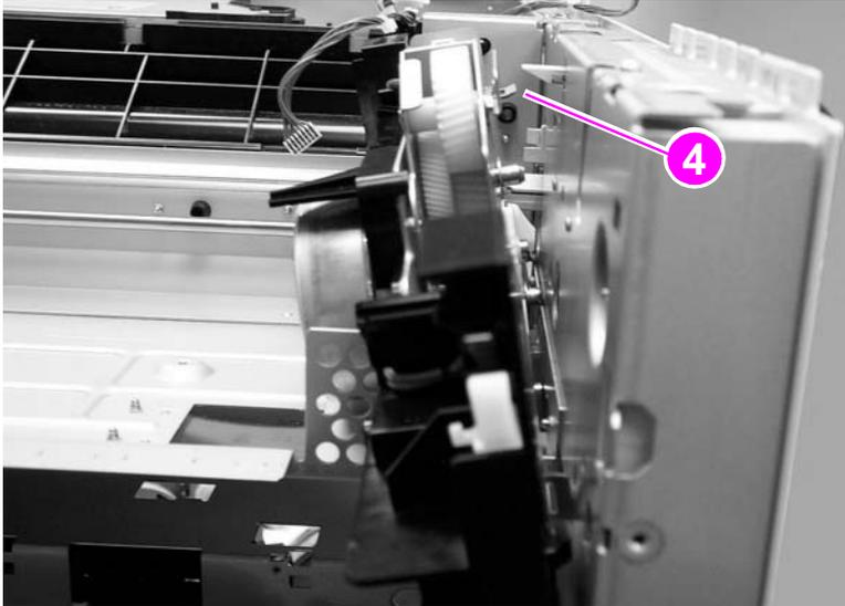
**Figure 100.** Fuser delivery-drive assembly (3 of 3)
