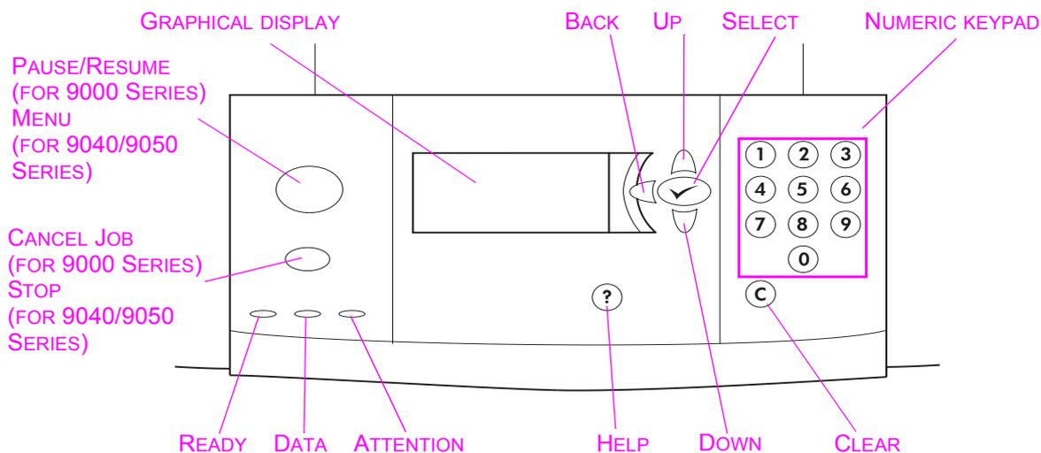
**Figure 11.** Control-panel layout
