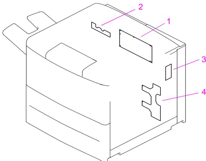
**Figure 149.** PCA assembly location
