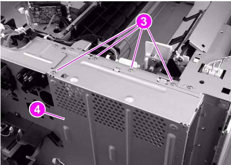
**Figure 96.** Fuser-connector holder assembly (2 of 3)
