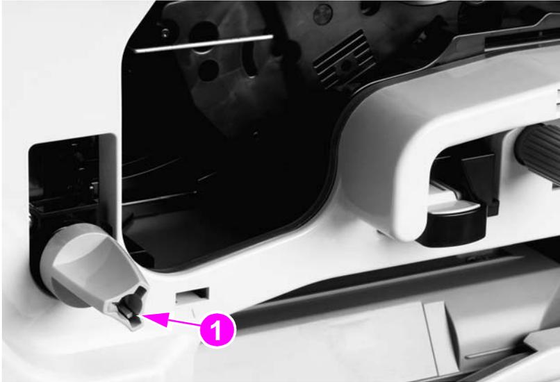
**Figure 63.** Fuser-jam-removal knob
