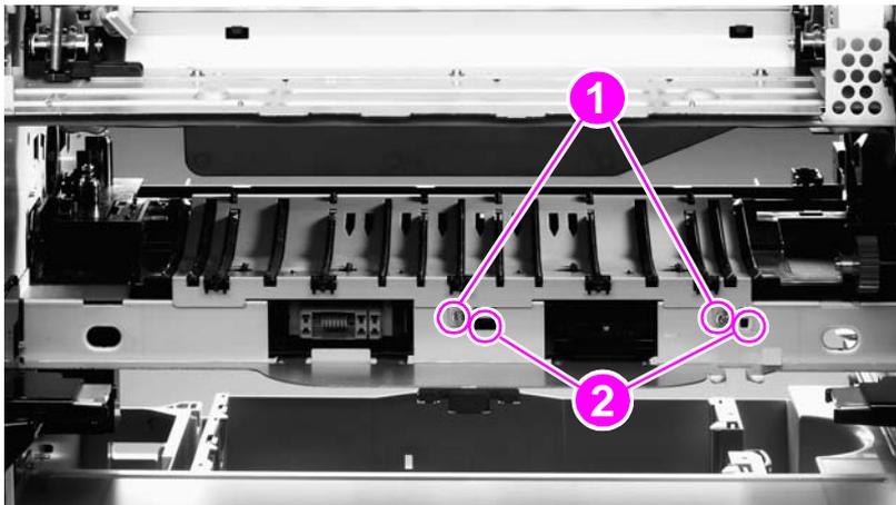
Figure 73. Transfer-guide assembly
