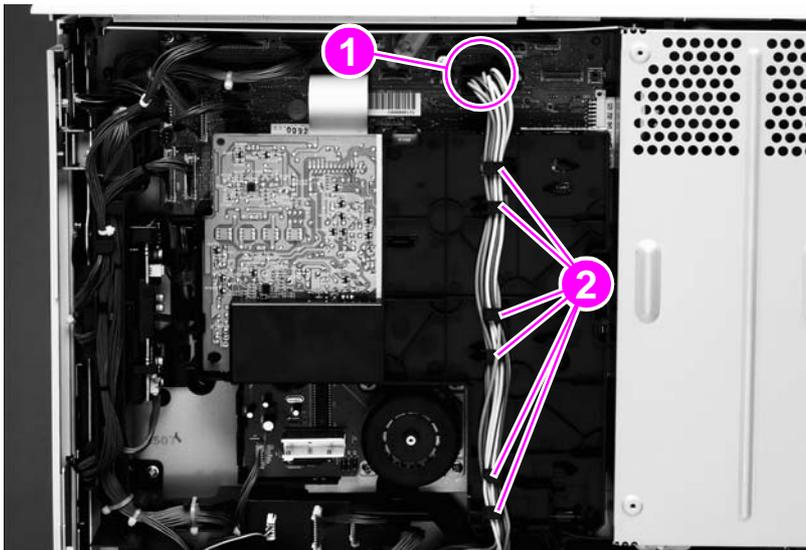
**Figure 80.** Low-voltage power supply (1 of 2)
