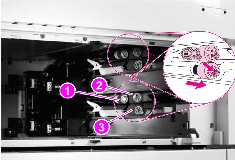
**Figure 62.** Rollers (pickup, feed, or separation)
