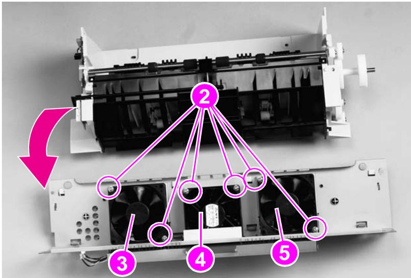
**Figure 54.** Delivery-assembly fans and face-down-bin fan (2 of 2)
