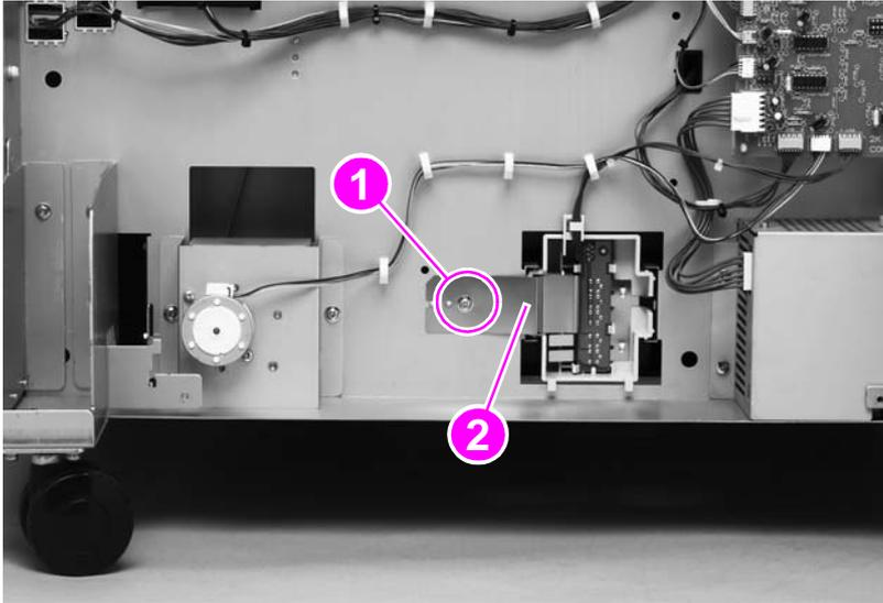
Figure 112. Paper-size switch PCA (1 of 2)
