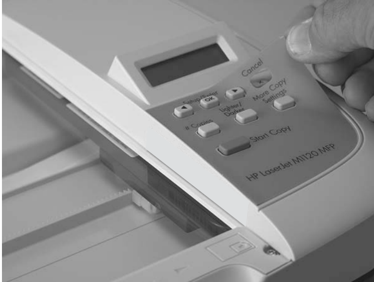
Figure 5-9 Remove the control-panel overlay
