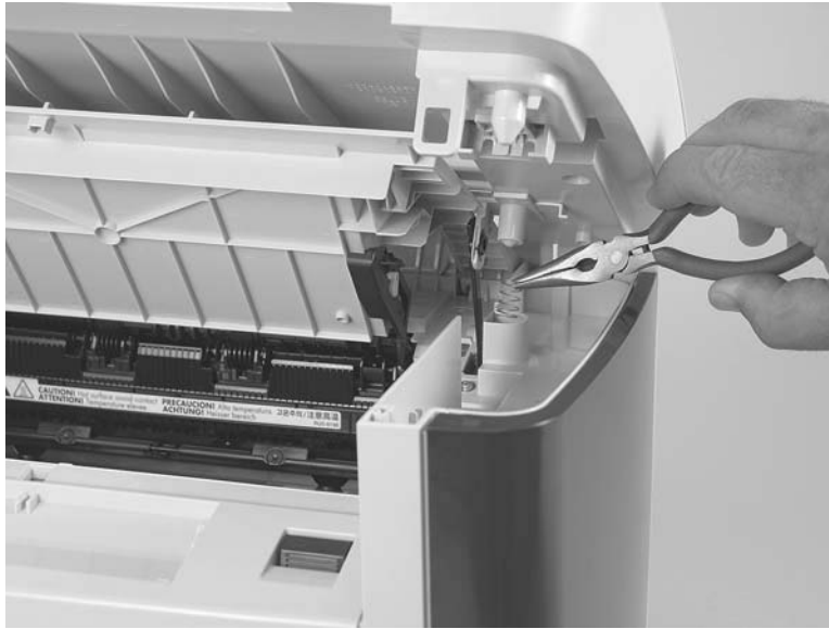
Figure 5-6 Remove the link assemblies and scanner support-frame spring (4 of 4)
