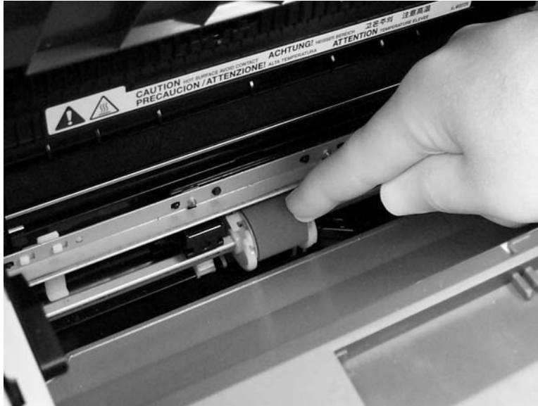
Figure 5-31 Remove the pickup roller (5 of 5)
