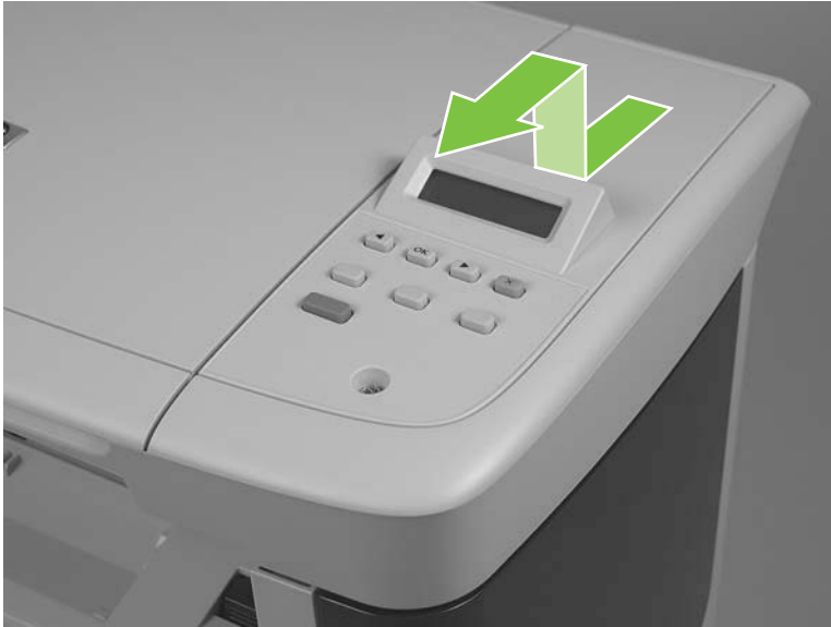
Figure 5-11 Remove the control-panel assembly (2 of 3)
