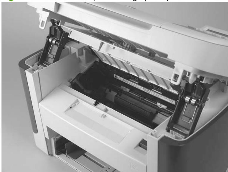
Figure 5-23 Remove the print cartridge (1 of 2)
