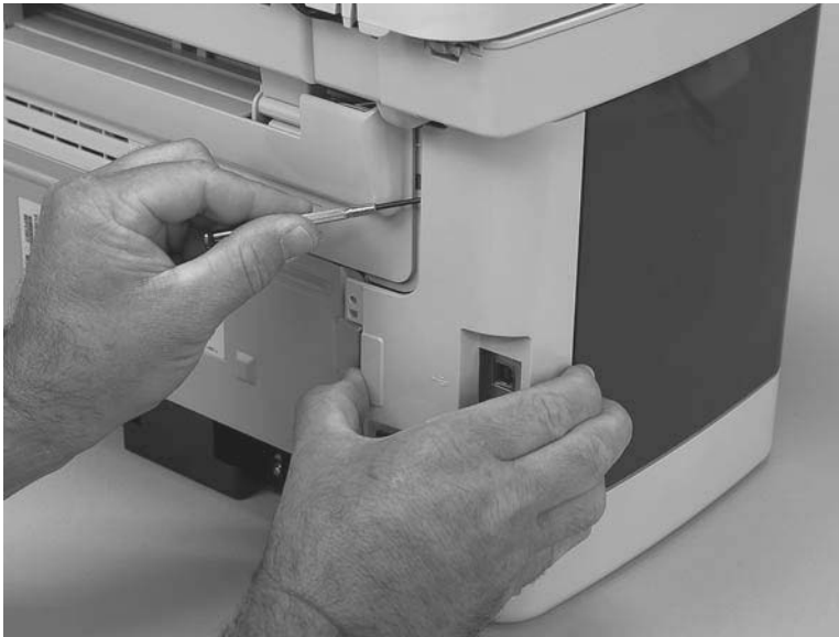
Figure 5-14 Remove the scanner assembly (2 of 10)
