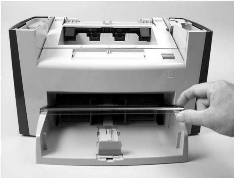
Figure 5-33 Remove the media input tray (1 of 3)
