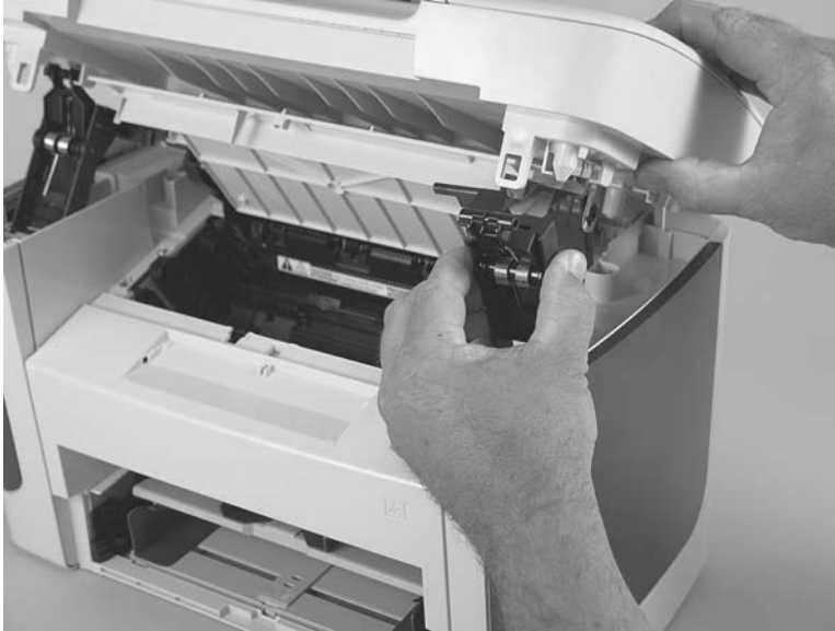
Figure 5-4 Remove the link assemblies and scanner support-frame spring (2 of 4)
