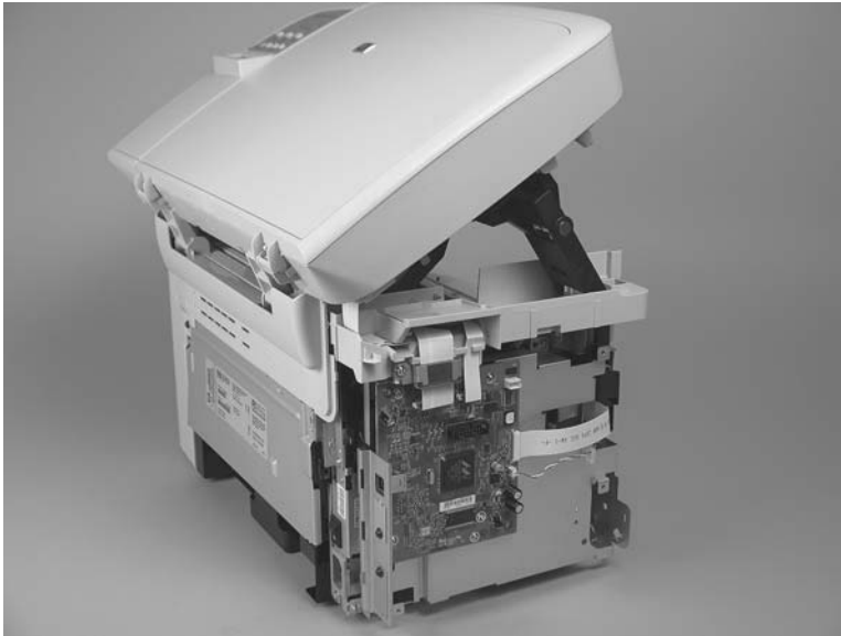
Figure 5-17 Remove the scanner assembly (5 of 10)
