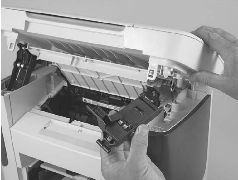
Figure 5-5 Remove the link assemblies and scanner support-frame spring (3 of 4)
