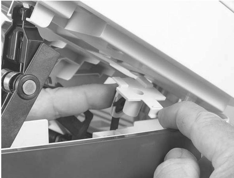
Figure 5-20 Remove the scanner assembly (8 of 10)
