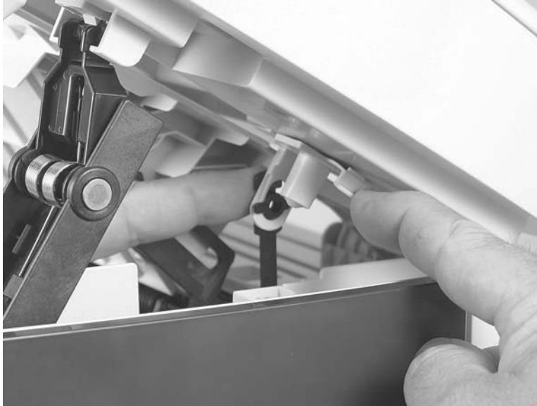
Figure 5-19 Remove the scanner assembly (7 of 10)
