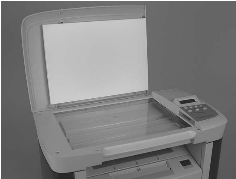
Figure 5-7 Remove the scanner lid (1 of 2)
