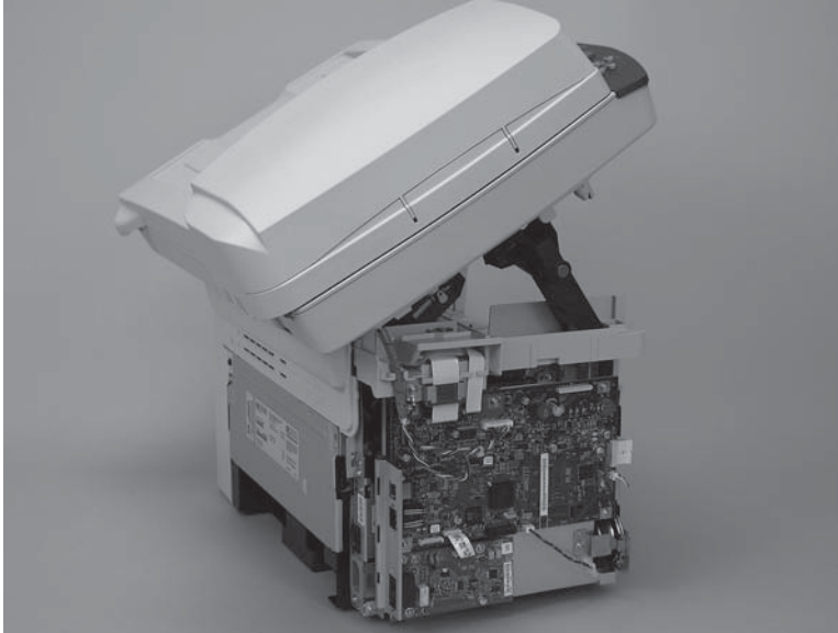
Figure 5-33 Remove the scanner assembly (5 of 10)
