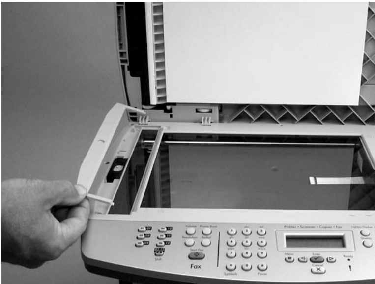
Figure 5-27 Remove the ADF scanner glass (2 of 3)
