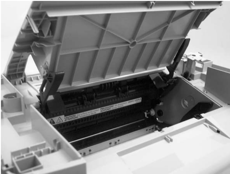
Figure 5-57 Remove the print-cartridge door (1 of 2)
