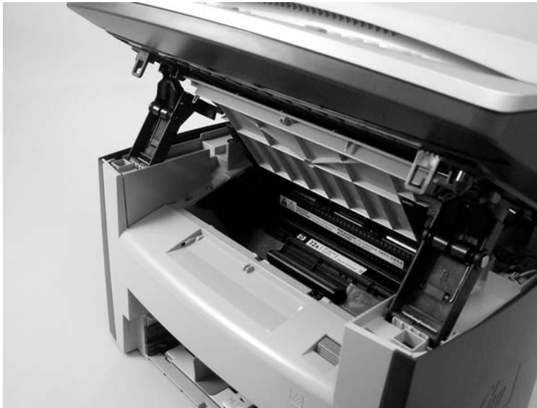
Figure 5-39 Remove the print cartridge (1 of 2)
