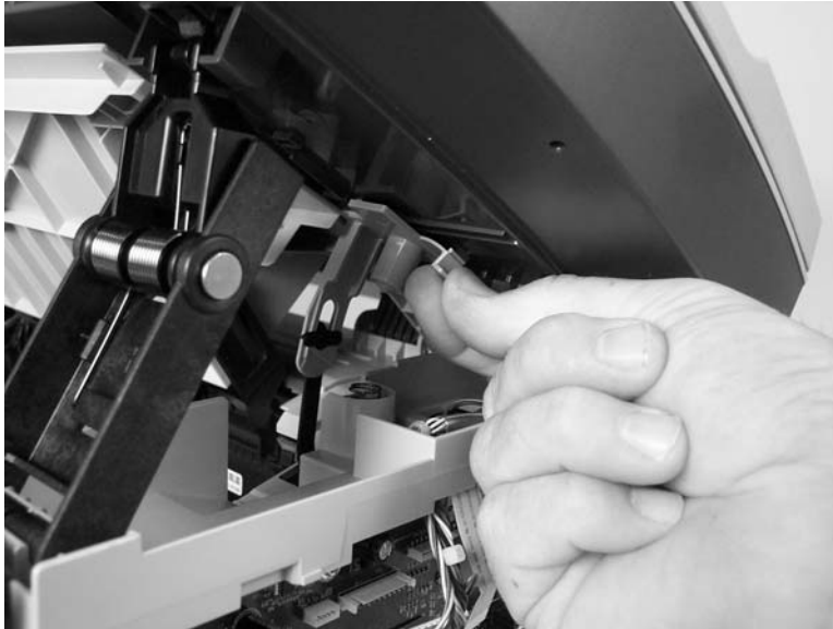
Figure 5-35 Remove the scanner assembly (7 of 10)
