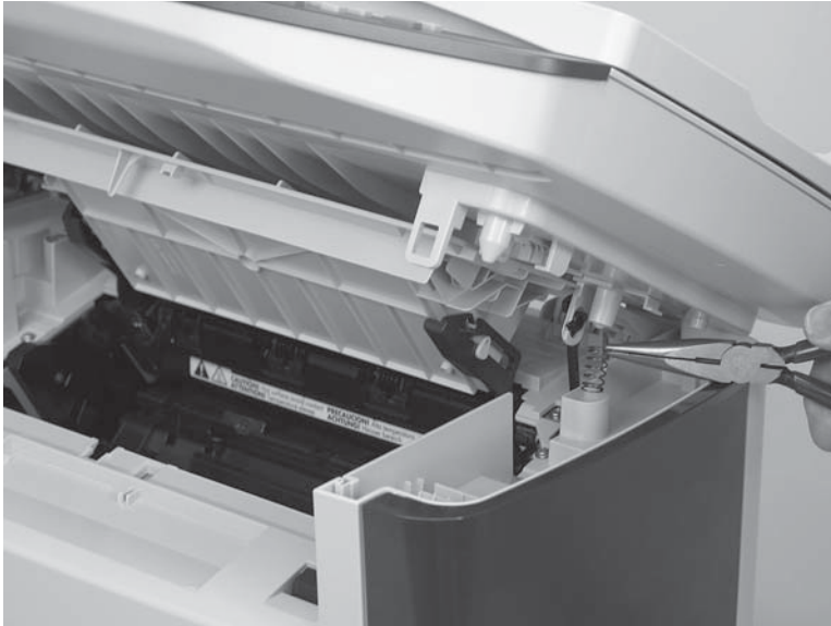
Figure 5-14 Remove the link assemblies and scanner support-frame springs (4 of 4)
