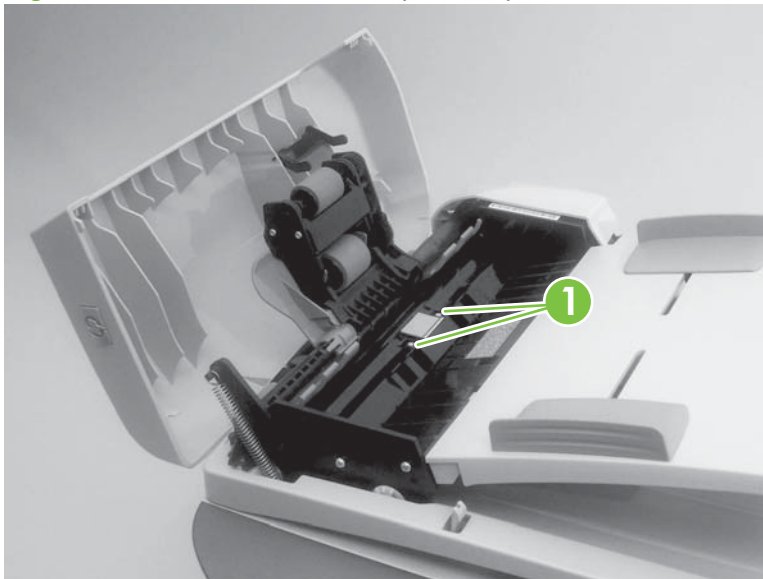
Figure 5-18 Remove the ADF separation pad
