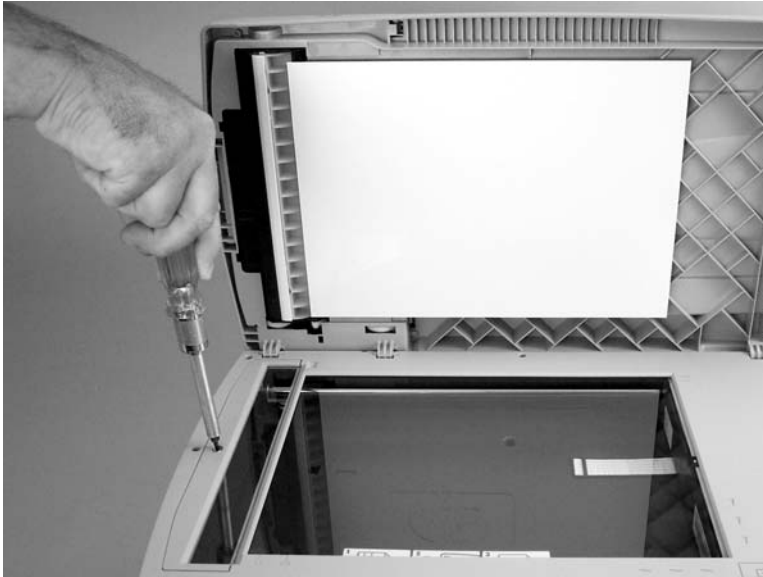
Figure 5-26 Remove the ADF scanner glass (1 of 3)
