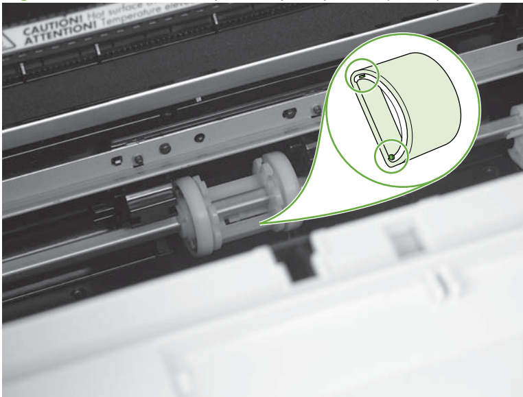
Figure 5-46 Remove the product pickup roller (4 of 5)
