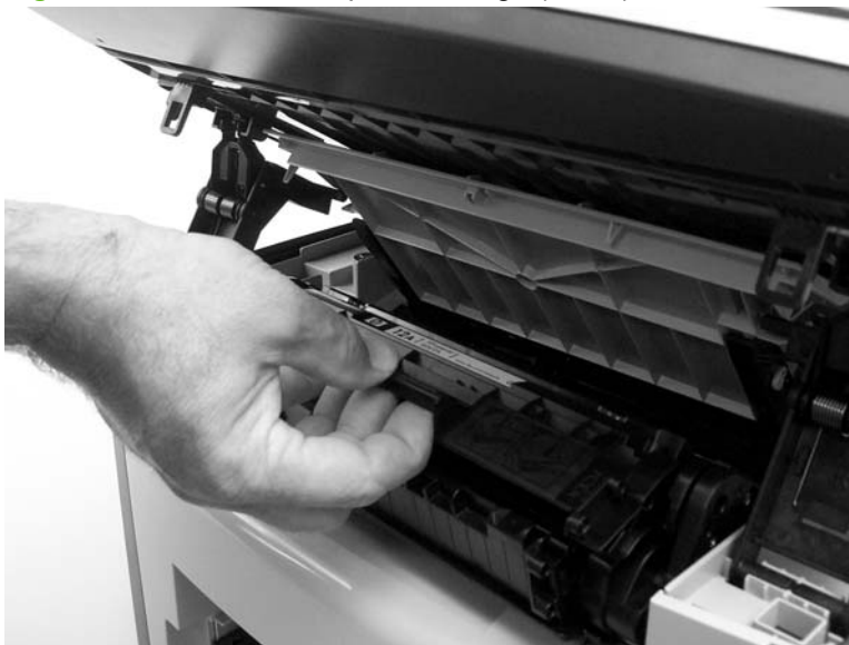
Figure 5-40 Remove the print cartridge (2 of 2)
