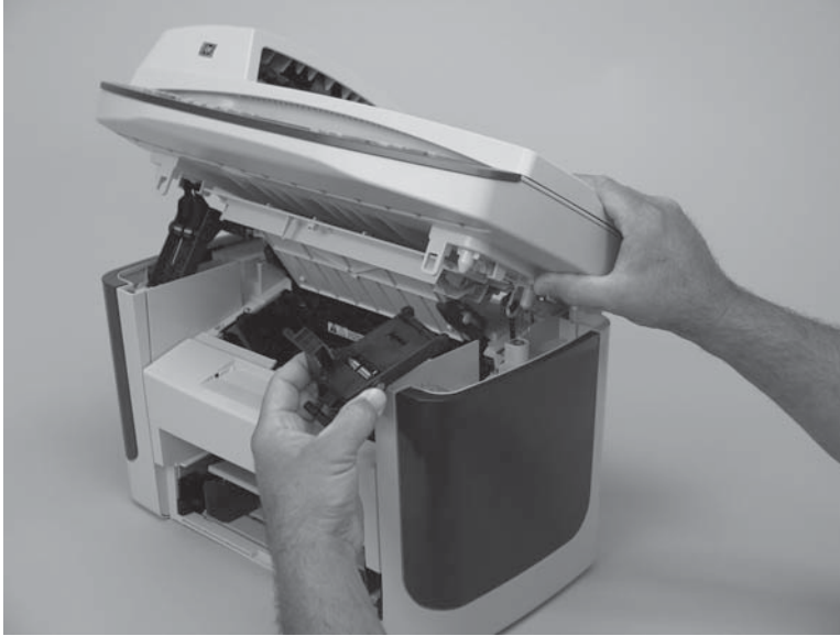
Figure 5-13 Remove the link assemblies and scanner support-frame springs (3 of 4)
