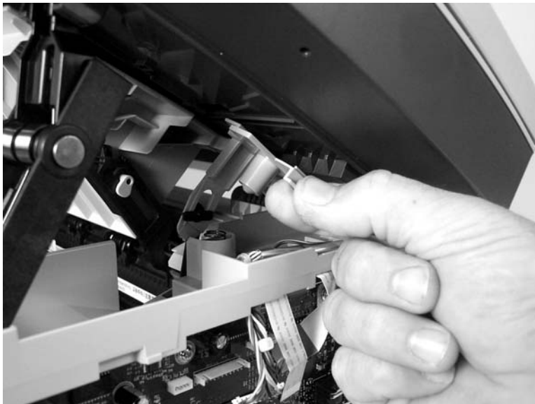
Figure 5-36 Remove the scanner assembly (8 of 10)
