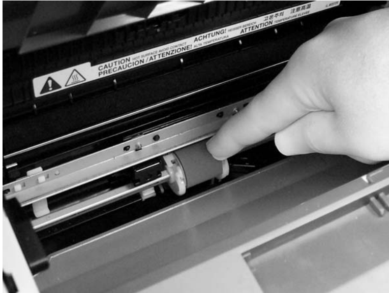
Figure 5-47 Remove the product pickup roller (5 of 5)
