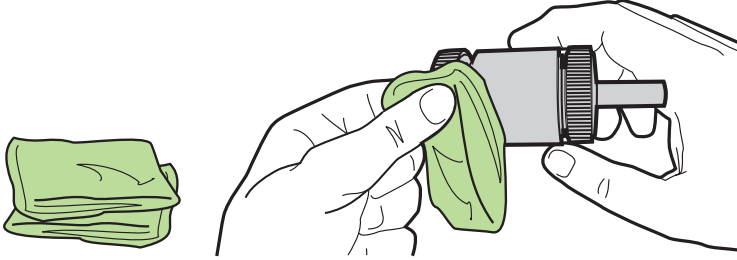
Figure 3-17 Clean the tray 2 pickup roller (1 of 6)
