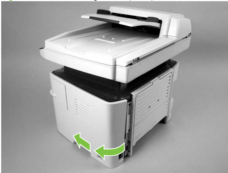
Figure 5-8 Remove the right cover (4 of 4)
