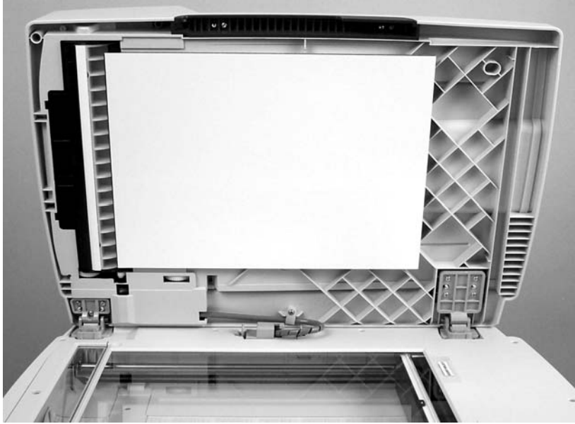
Figure 5-31 Remove the ADF assembly (1 of 3)
