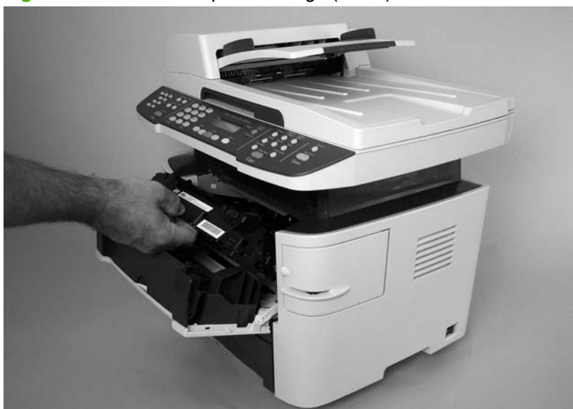
Figure 5-4 Remove the print cartridge (2 of 2)
