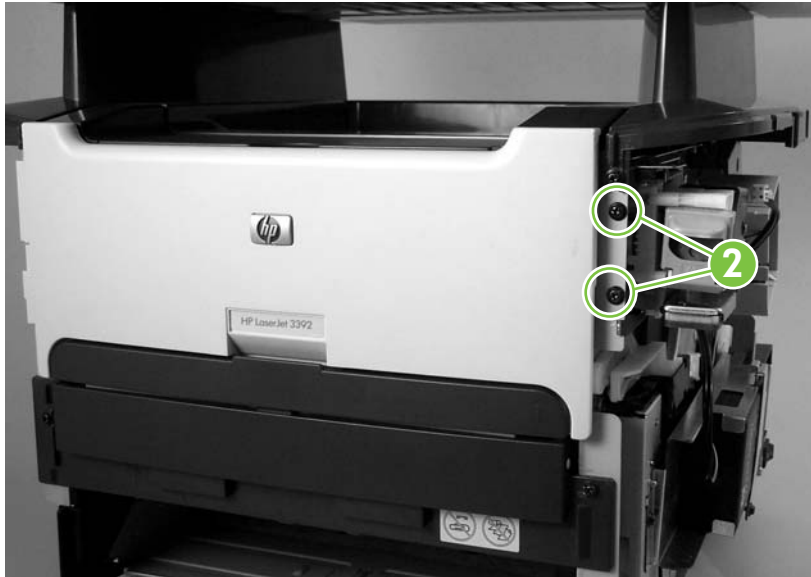
Figure 5-43 Remove the convenience-stapler assembly (2 of 2)
