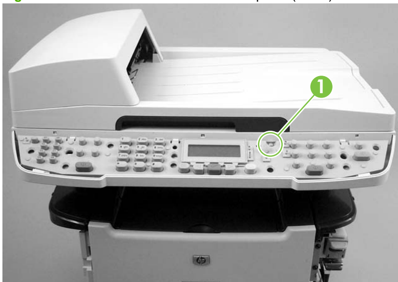
Figure 5-39 Remove the bezel and control panel (2 of 4)
