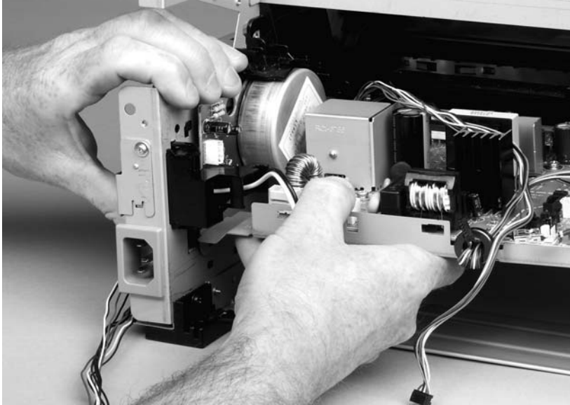
Figure 5-84 Remove the ECU (5 of 8)
