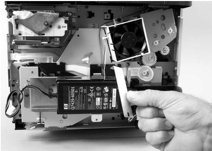
Figure 5-45 Remove the convenience-stapler power assembly (2 of 3)
