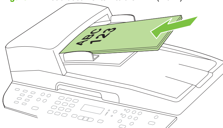
Figure 2-7 Load documents into the ADF (1 of 2)
