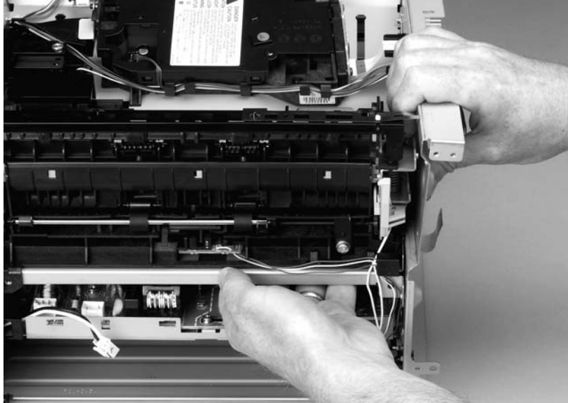
Figure 5-77 Remove the fuser (8 of 9)
