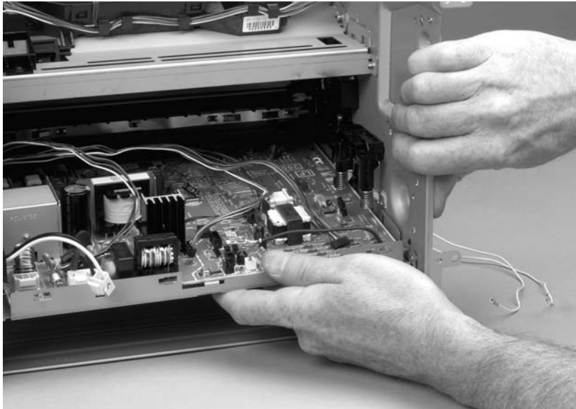
Figure 5-85 Remove the ECU (6 of 7)
