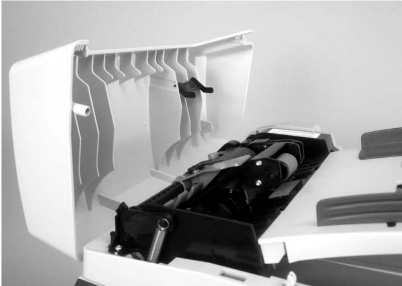
Figure 5-22 Replace the ADF pickup-roller assembly (1 of 6)
