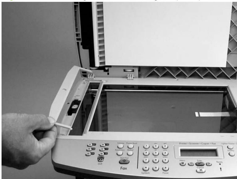
Figure 5-29 Removing the ADF scanner glass (2 of 3)
