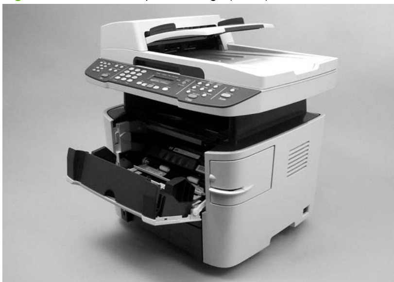
Figure 5-3 Remove the print cartridge (1 of 2)
