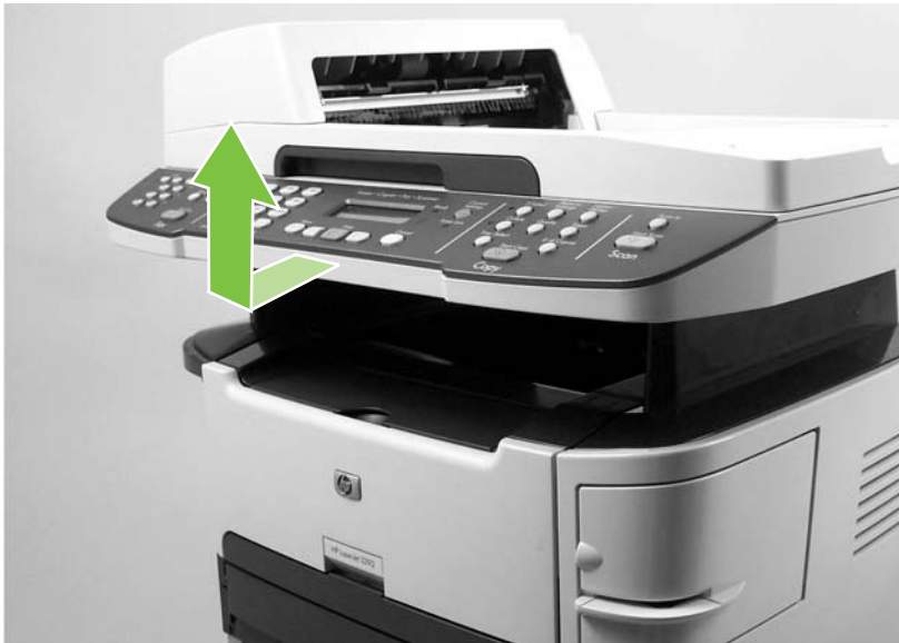
Figure 5-37 Remove the scanner/ADF assembly (4 of 4)
