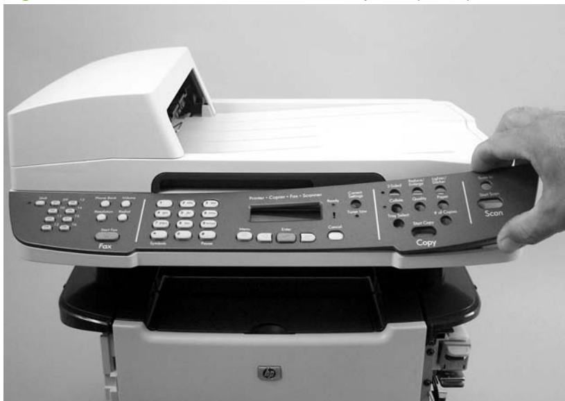
Figure 5-38 Remove the bezel and control panel (1 of 4)
