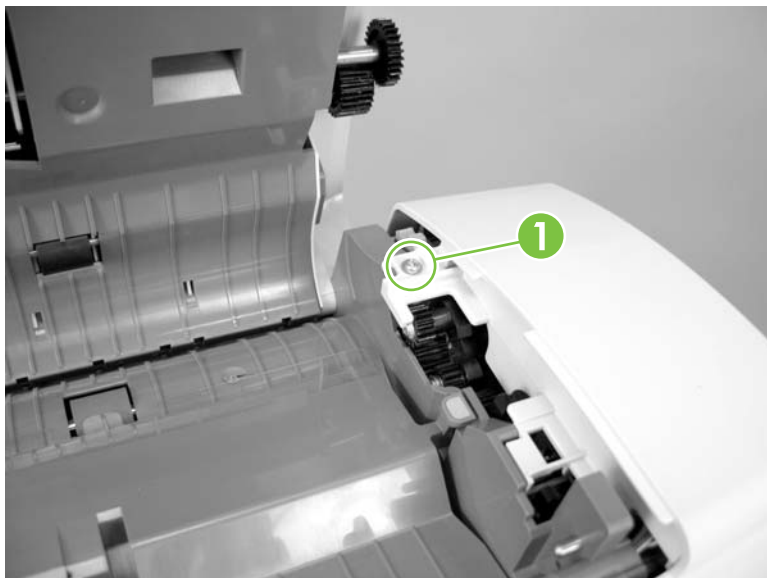
Figure 5-67 Remove the ADF rear end cover (1 of 5)
