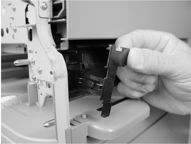
Figure 5-224 Remove the print cartridge door (10 of 12)
