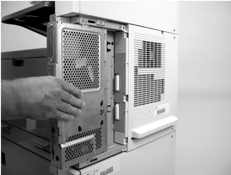
Figure 5-32 Remove the formatter cover and cage (3 of 3)
