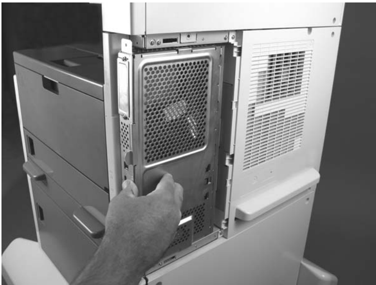
Figure 5-33 Reinstall the formatter cage
