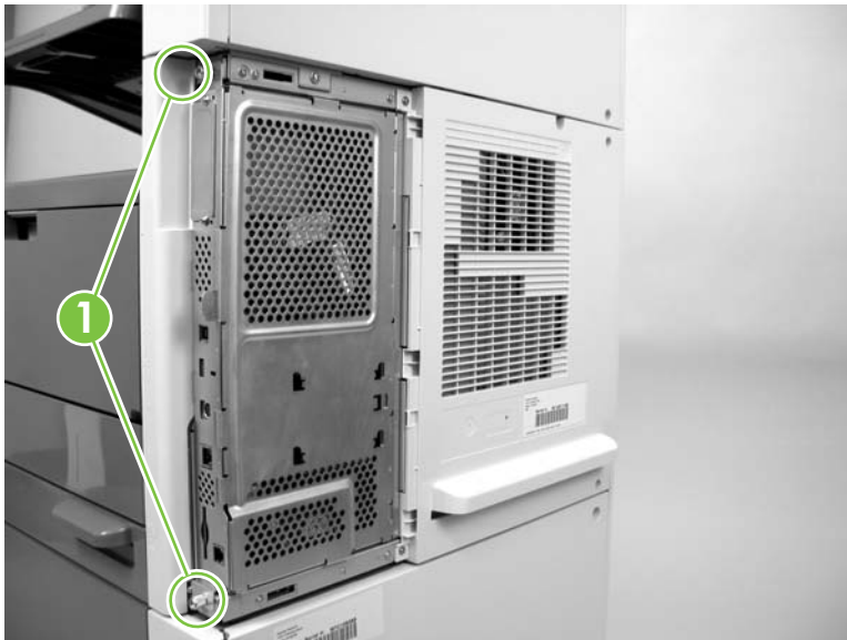
Figure 5-31 Remove the formatter cover and cage (2 of 3)
