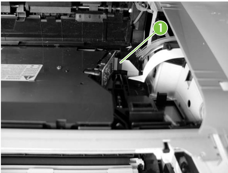
Figure 5-249 Remove the laser/scanner (1 of 3)
