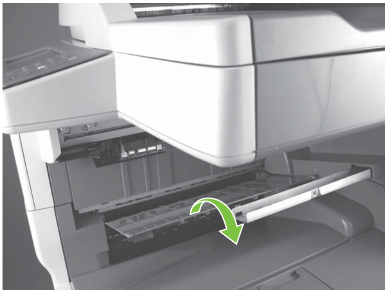
Figure 5-131 Remove the duplex cover
