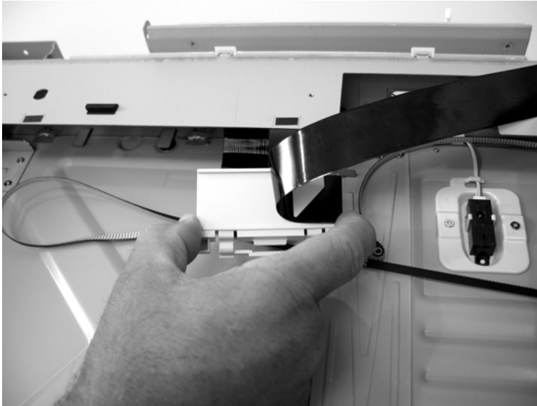
Figure 5-108 Remove the scanner optic assembly (13 of 13)
