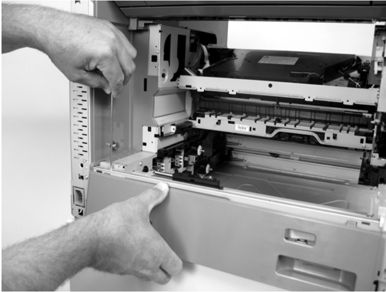
Figure 5-204 Remove the base unit lower left cover (3 of 4)
