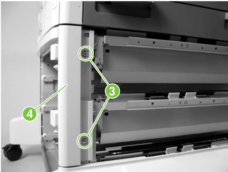
Figure 5-308 Remove the HCI paper pickup assembly (2 of 6)
