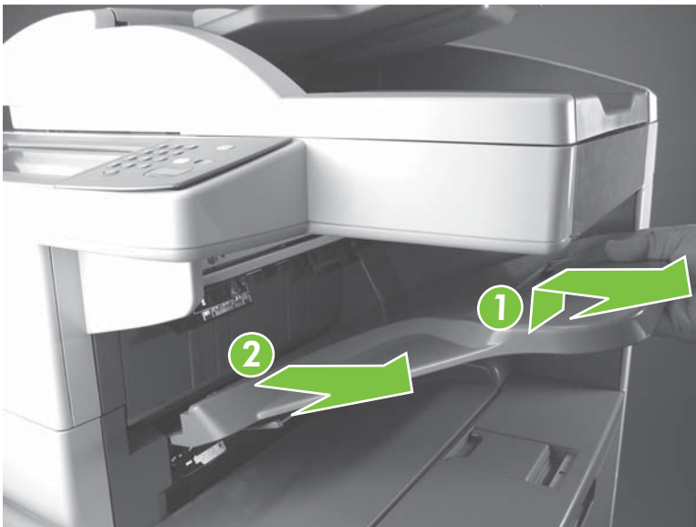
Figure 5-130 Remove the stapler output bin (2 of 2)
