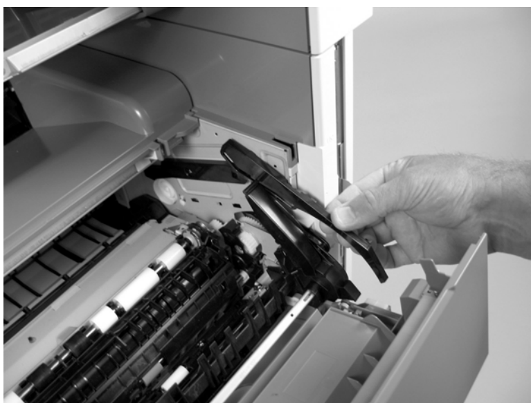
Figure 5-228 Remove the registration assembly (2 of 5)
