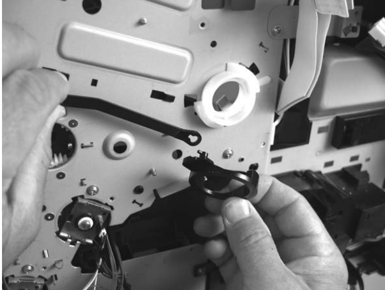
Figure 5-289 Reinstall the print cartridge cam linkage (1 of 2)
