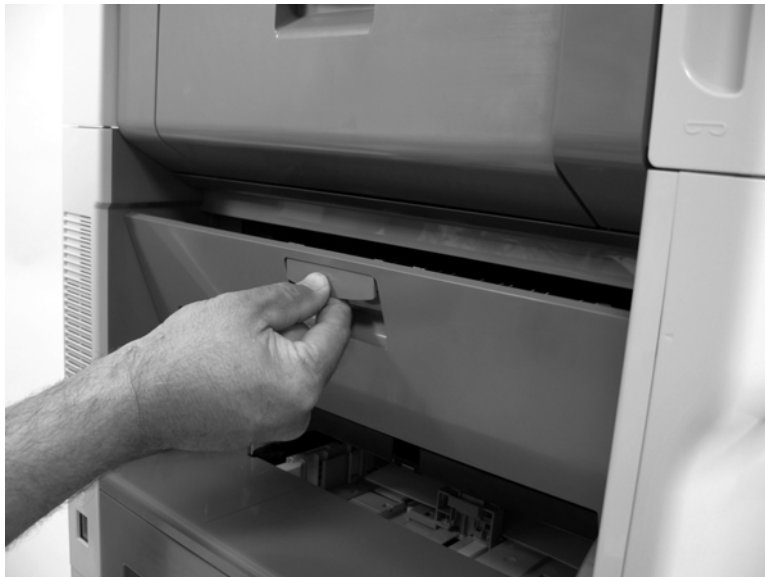
Figure 5-24 Remove the fuser (2 of 6)
