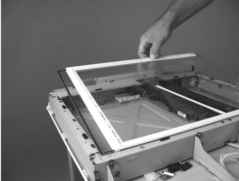
Figure 5-94 Remove the scanner glass assembly and top cover (6 of 7)
