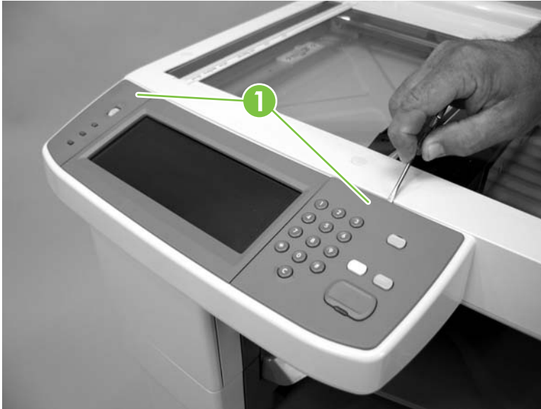
Figure 5-78 Remove the control panel (1 of 3)
