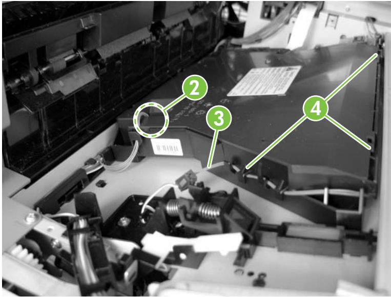
Figure 5-250 Remove the laser/scanner (2 of 3)
