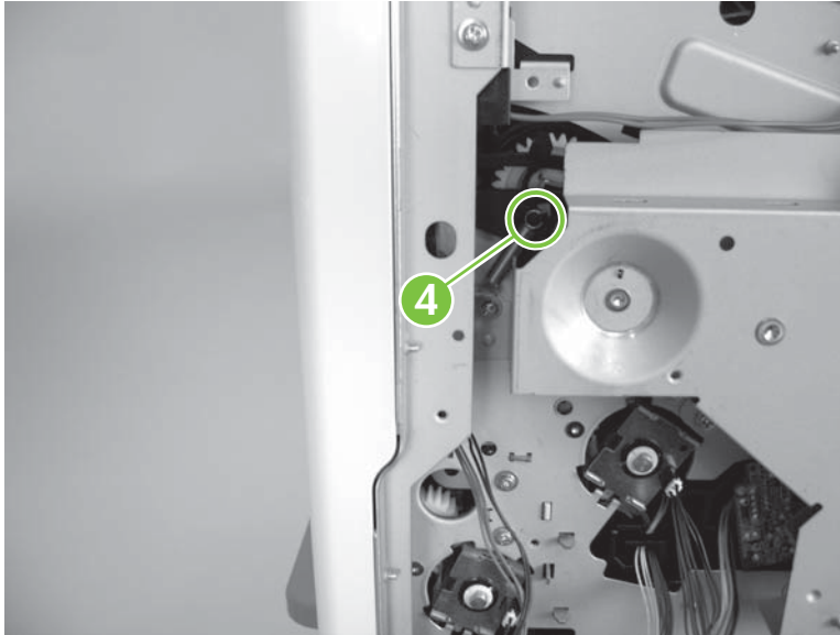
Figure 5-285 Remove the main motor (4 of 7)
