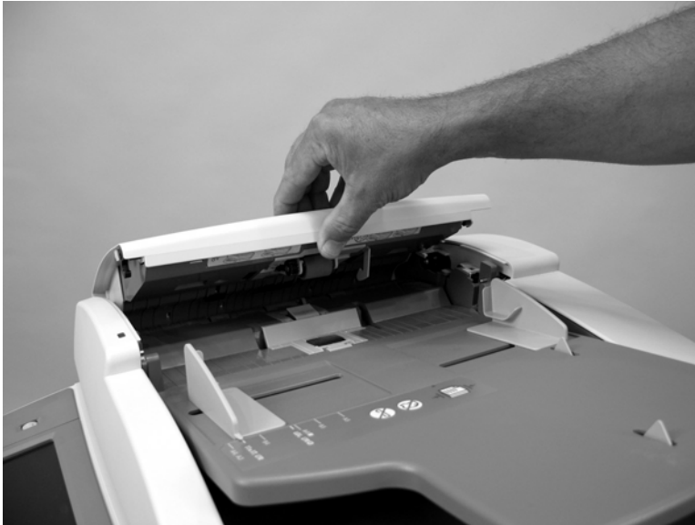
Figure 5-44 Remove the ADF separation floor assembly (1 of 4)
