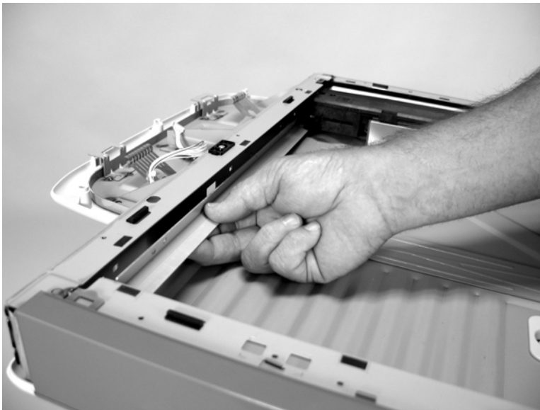
Figure 5-119 Remove the scanner transmission assemblies and slide rail (5 of 5)
