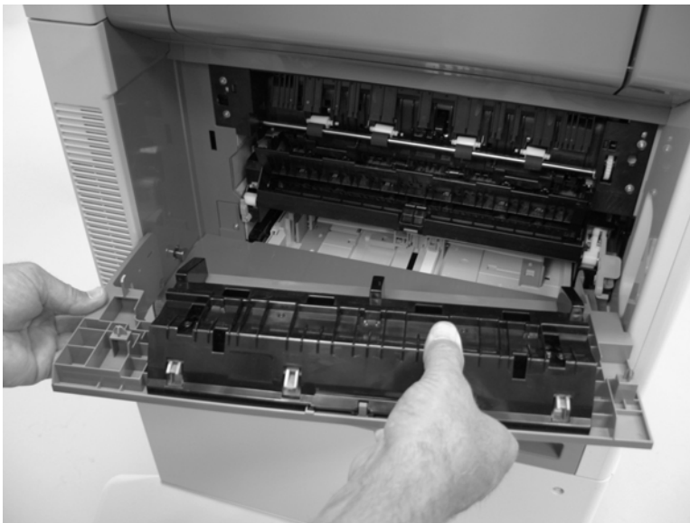
Figure 5-179 Remove the base unit left door (2 of 2)
