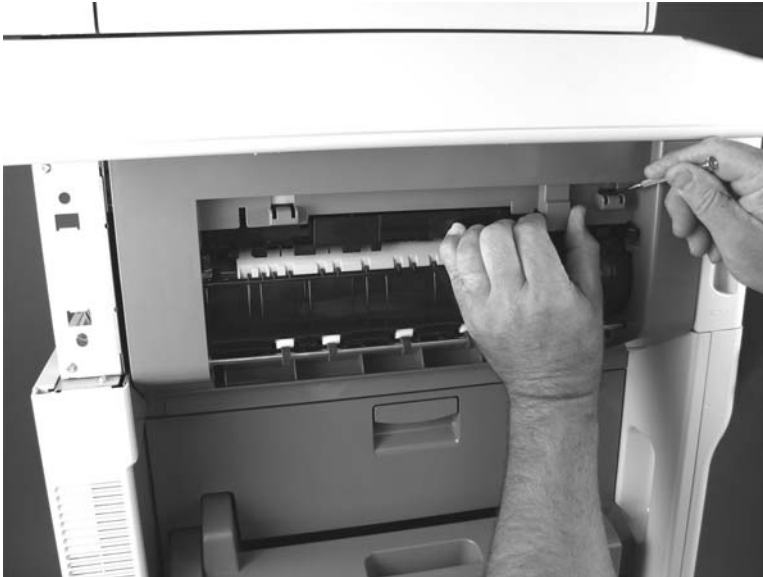
Figure 5-134 Remove the stapler left cover (1 of 3)
