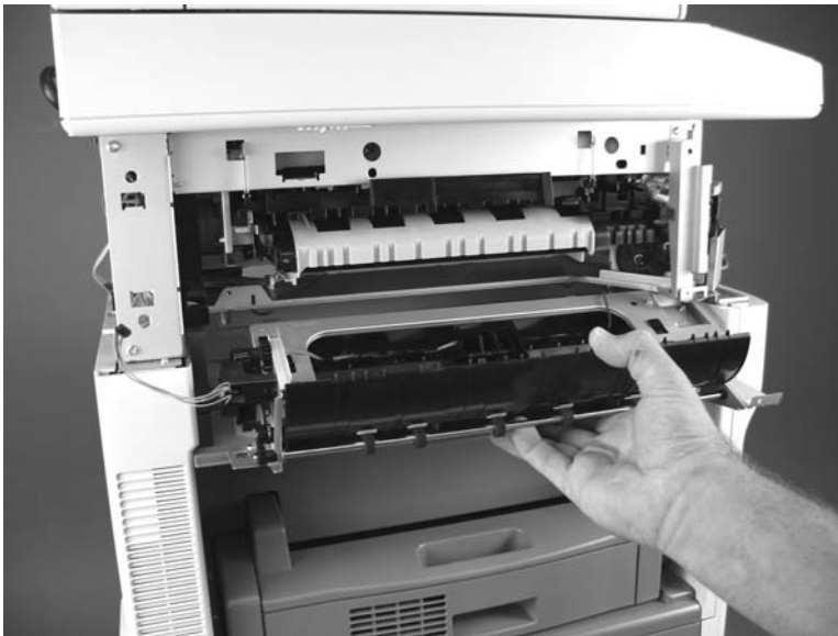
Figure 5-155 Remove the stapler paper feed assembly (3 of 3)
