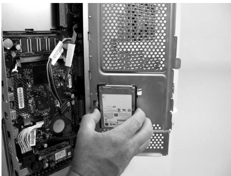
Figure 5-35 Remove the hard drive (2 of 2)
