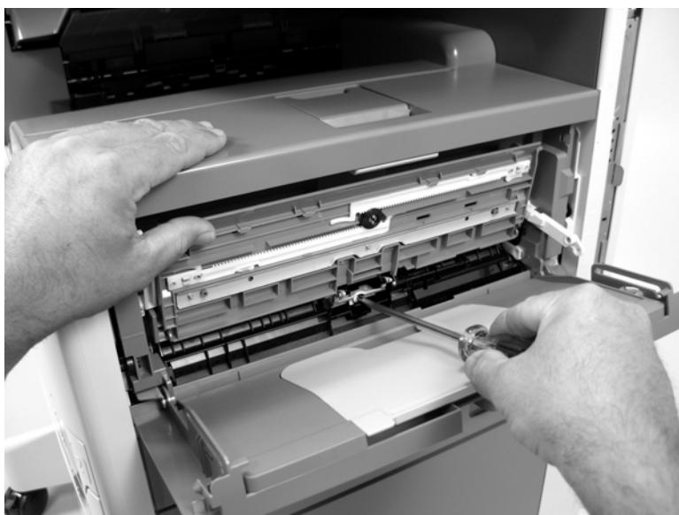
Figure 5-14 Remove the Tray 1 separation pad assembly (2 of 3)
