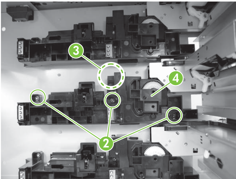
Figure 5-319 Remove the HCI lifter driver assembly (2 of 2)
