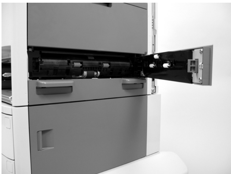
Figure 5-17 Remove the Tray 2 and Tray 3 pickup rollers (2 of 4)
