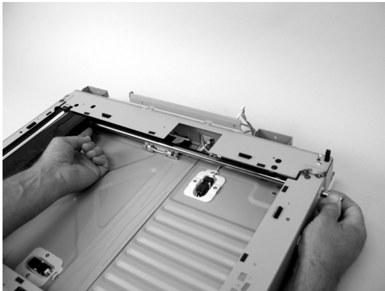
Figure 5-99 Remove the scanner optic assembly (4 of 13)
