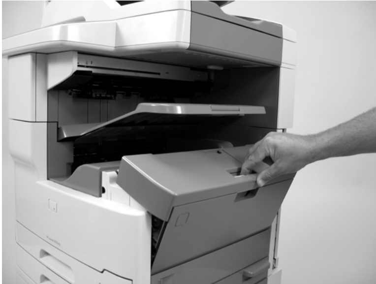
Figure 5-2 Remove the print cartridge (1 of 2)
