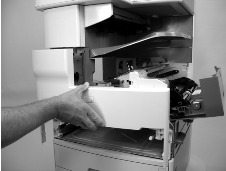
Figure 5-191 Remove the base unit front cover (7 of 7)
