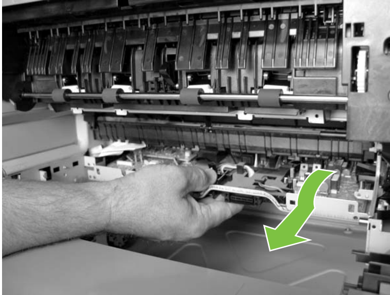
Figure 5-266 Remove the high-voltage power supply assembly (8 of 9)
