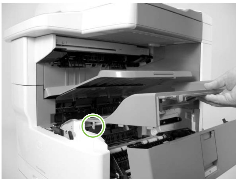
Figure 5-177 Remove the base unit face-down cover (2 of 2)
