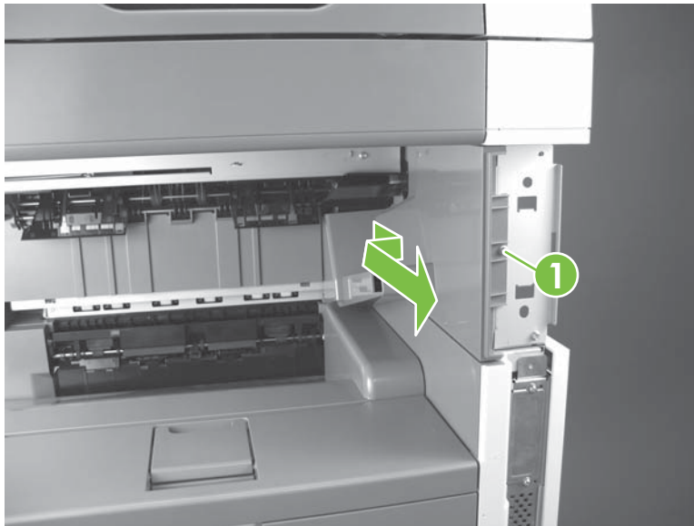
Figure 5-148 Remove the stapler rear inner cover
