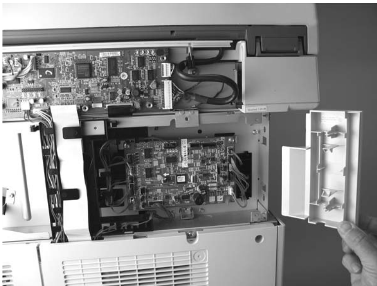
Figure 5-139 Remove the stapler right and left rear covers (4 of 4)
