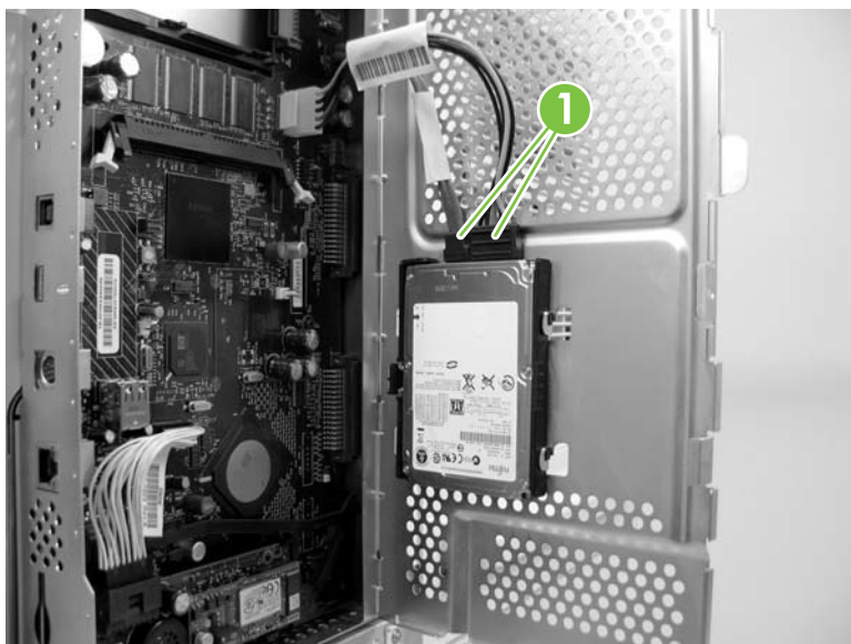
Figure 5-34 Remove the hard drive (1 of 2)
