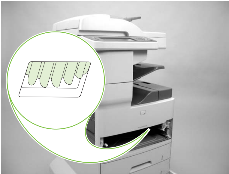
Figure 5-270 Reinstall the high-voltage power supply assembly (3 of 3)
