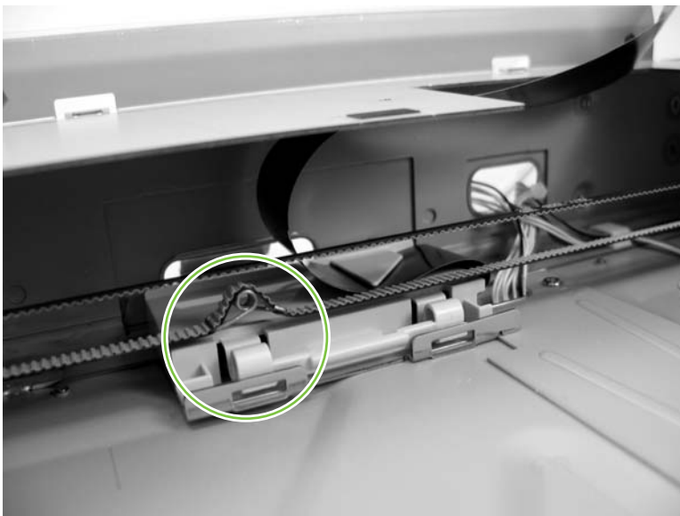
Figure 5-105 Remove the scanner optic assembly (10 of 13)
