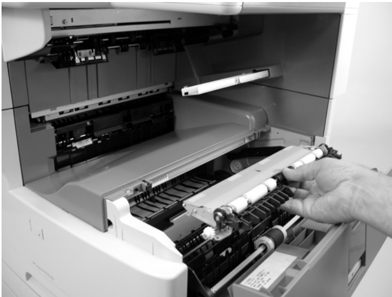
Figure 5-230 Remove the registration assembly (4 of 5)
