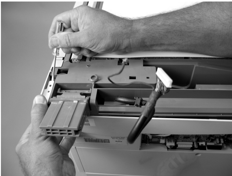
Figure 5-70 Remove the ADF rear end cover (4 of 5)
