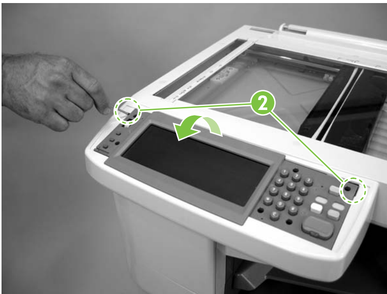
Figure 5-79 Remove the control panel (2 of 3)
