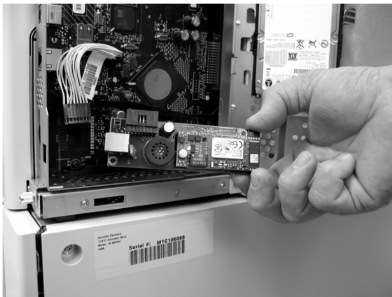
Figure 5-37 Remove the Fax PCA (2 of 2)
