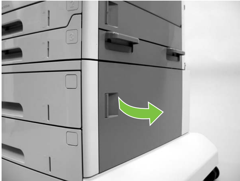
Figure 5-298 Remove the HCI right door (1 of 5)
