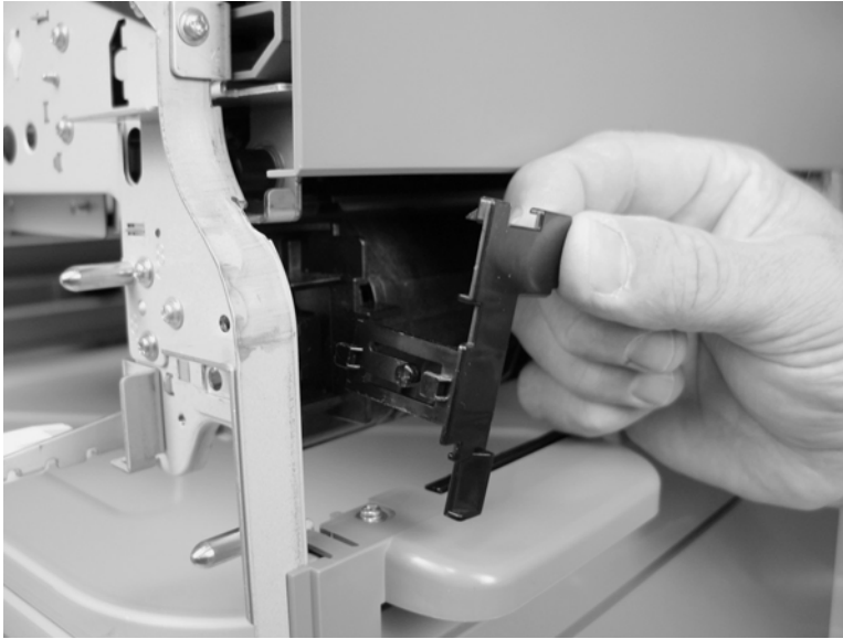
Figure 5-294 Remove the lower cassette pickup assembly (4 of 5)
