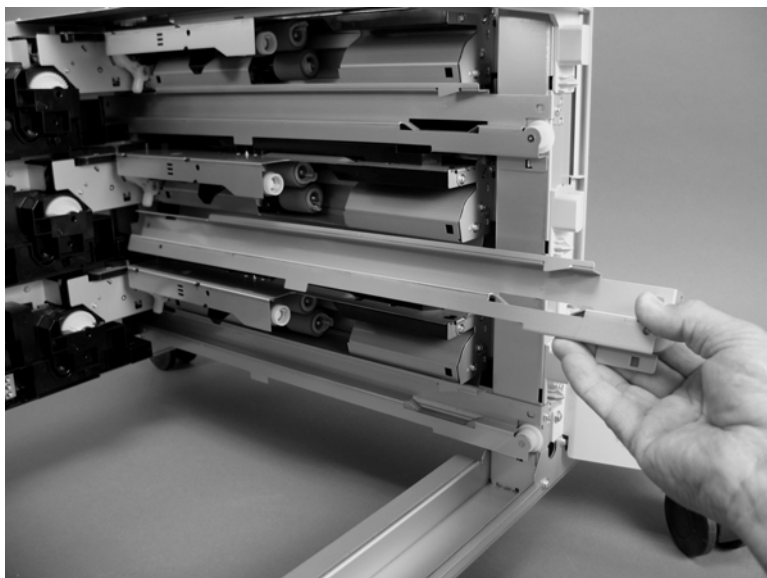
Figure 5-314 Remove the HCI right side tray rail(s) (2 of 2)
