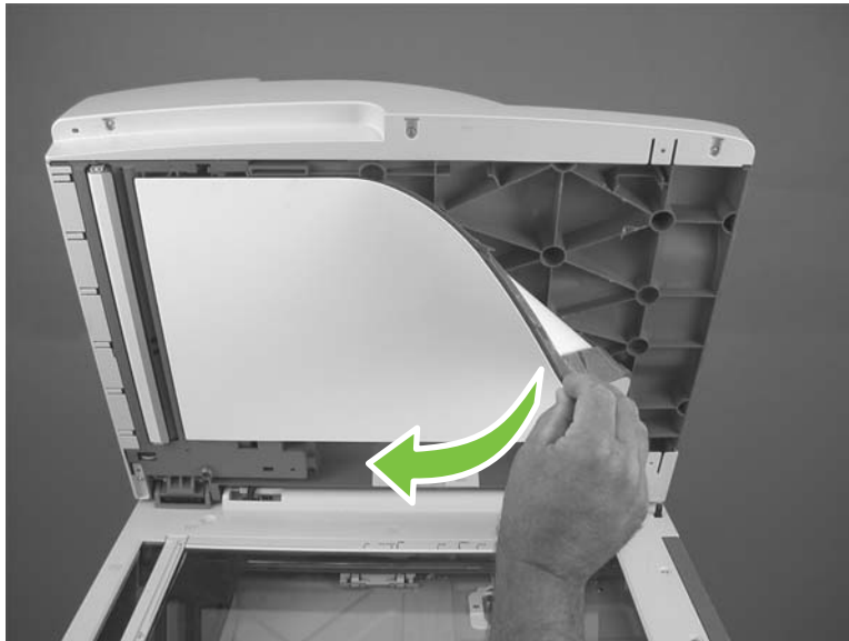
Figure 5-59 Remove the ADF white backing (1 of 4)
