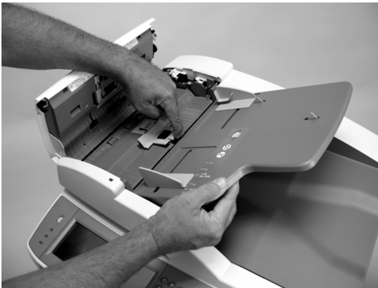
Figure 5-5 Remove the ADF separation pad and pickup and feed roller assemblies (2 of 5)
