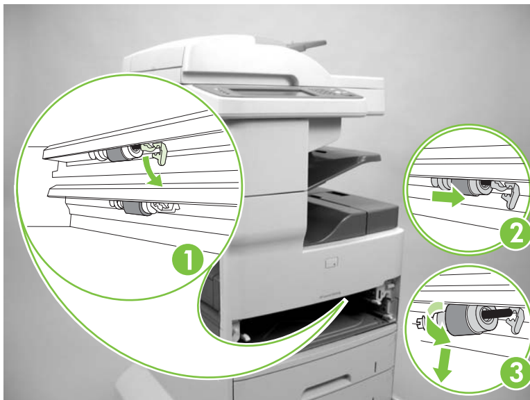
Figure 5-19 Remove the Tray 2 and Tray 3 pickup rollers (4 of 4)
