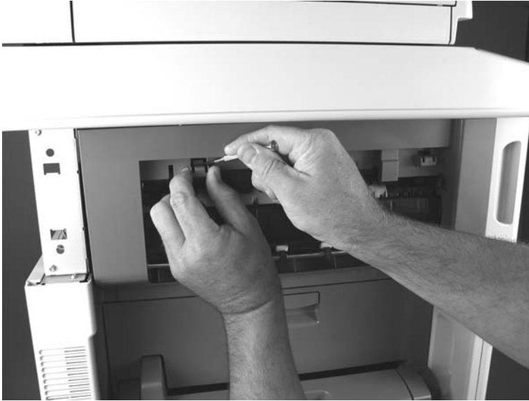
Figure 5-133 Remove the stapler left cover (2 of 3)
