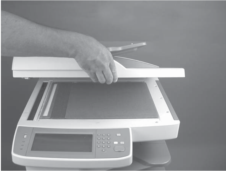
Figure 5-61 Remove the ADF white backing (3 of 4)
