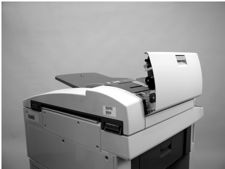
Figure 5-50 Remove the ADF jam cover (1 of 3)
