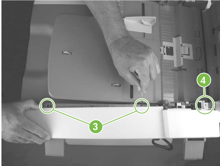
Figure 5-71 Remove the ADF rear end cover (5 of 5)
