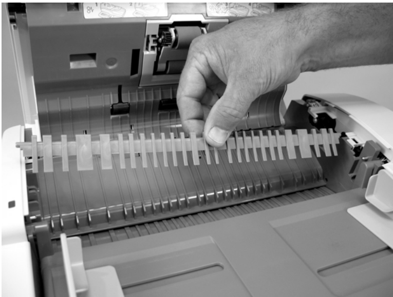
Figure 5-49 Remove the ADF diverter (2 of 2)
