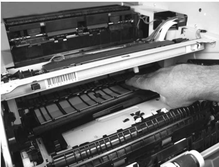
Figure 5-244 Reinstall the paper feed assembly (6 of 8)
