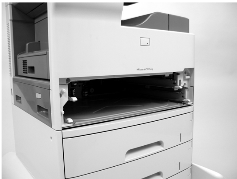
Figure 5-16 Remove the Tray 2 and Tray 3 pickup rollers (1 of 4)
