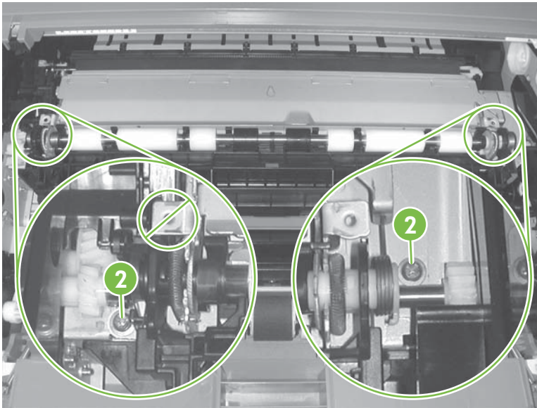
Figure 5-229 Remove the registration assembly (3 of 5)
