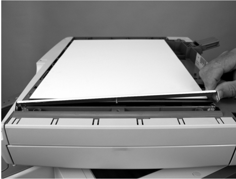
Figure 5-56 Remove the ADF float assembly (3 of 5)
