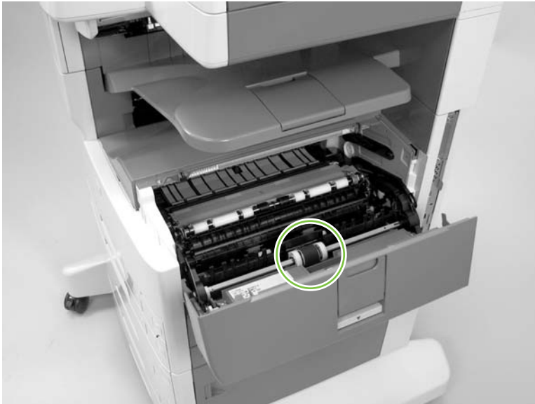
Figure 5-11 Remove the Tray 1 pickup roller (1 of 2)
