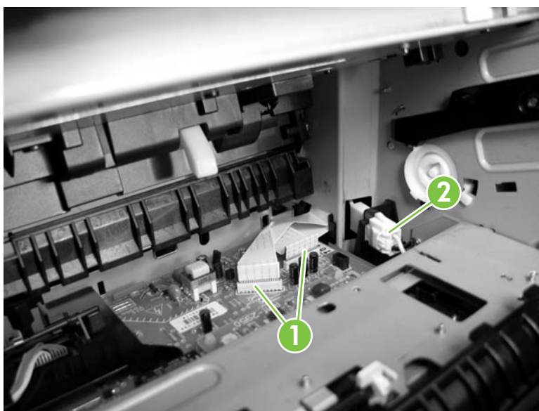
Figure 5-259 Remove the high-voltage power supply assembly (1 of 9)
