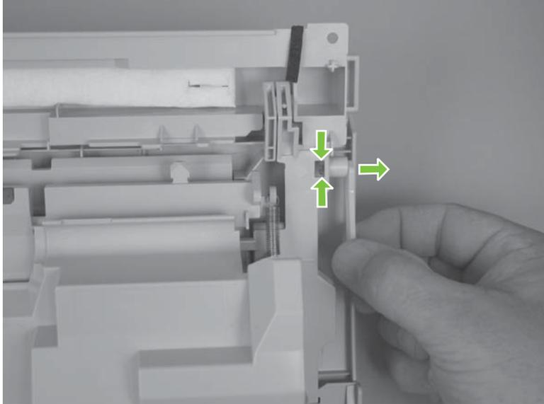
2. Remove the cartridge-door link (callout 2), and then install it on the replacement assembly.
