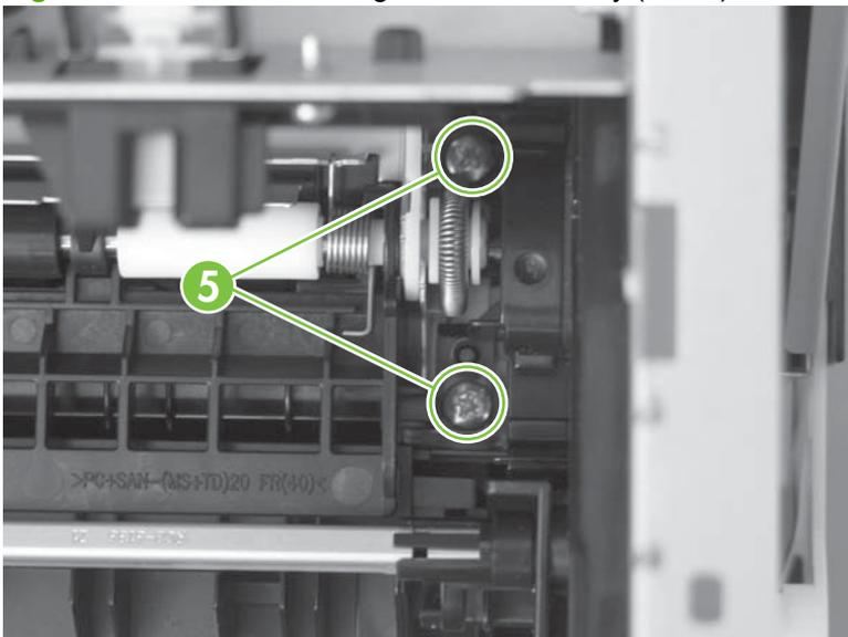
7. Slightly raise the right end of the assembly, and then slide it to the right and lift it up to release it.
