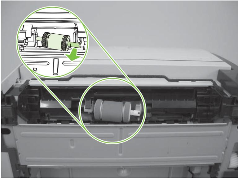
6. Remove the pickup roller.
