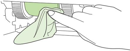
6. Allow the pickup roller to dry completely.
