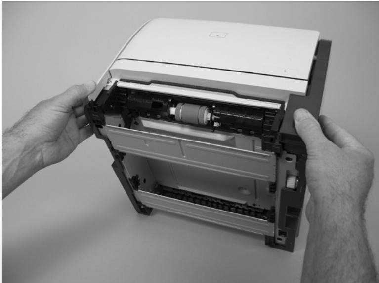
3. Use a small flat blade screwdriver to release one tab (callout 1), and then rotate the locking collar toward the inside of the product.
