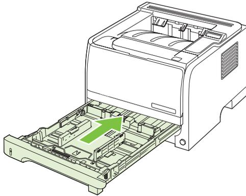
4. If no jammed paper is visible in the tray area, open the print-cartridge door, remove the print cartridge, and pull down the upper media guide. With both hands, grasp the jammed paper and slowly pull it out of the product.
