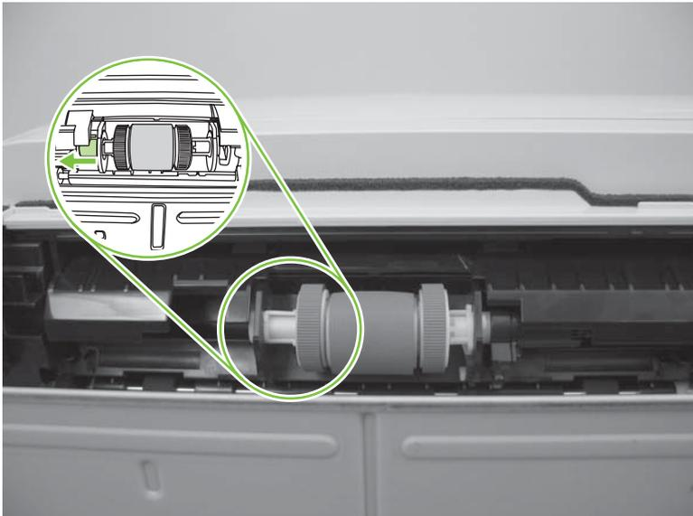
5. Rotate the drive end of the roller assembly out and away from the product.
