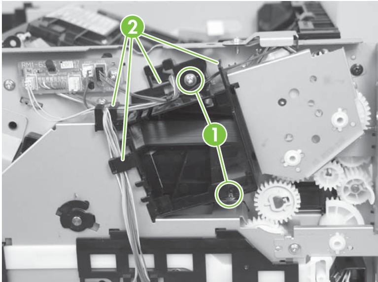
3. Remove the fan duct.
