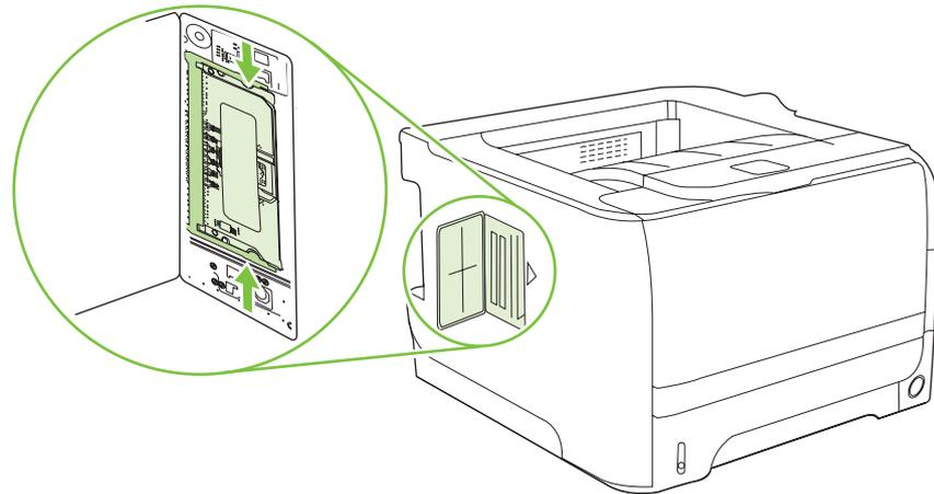
7. Close the access door, and press firmly until it snaps into place.
