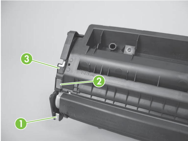
**Figure 7-2** High-voltage contact points (on the product)
