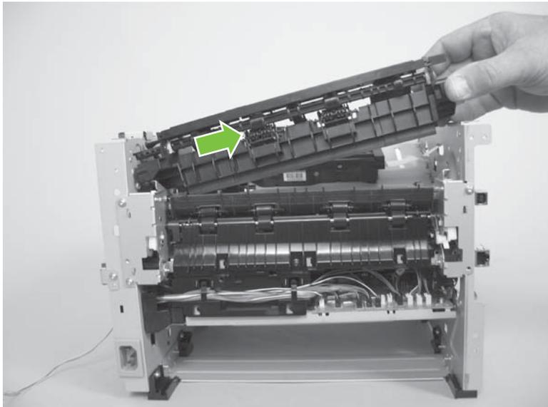
7. Remove the paper-retaining-delivery assembly
