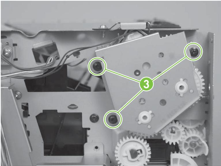
5. Remove the face-down-drive or duplexing-paper-feed assembly.
