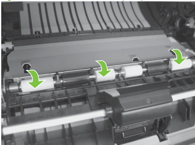
3. Before you proceed, note the location of the two tabs on the transfer-roller right-side locking clip.
