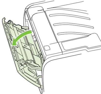
Media guides ensure that the media is correctly fed into the product and that the print is not skewed (crooked on the media). When loading media, adjust the media guides to match the width of the media that you are using.
