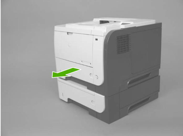
2. Carefully lift up on the tray to release it, and then remove the tray.
