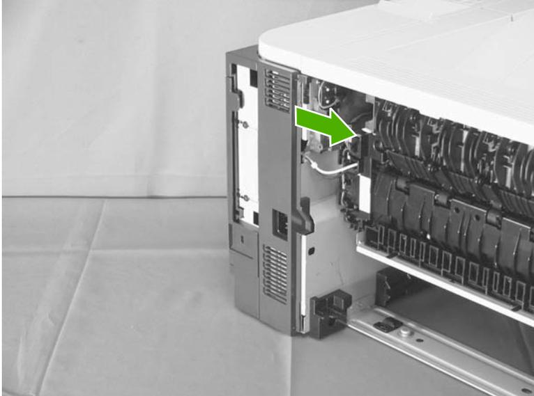
3. Rotate the bottom of the cover away from the product, and then pull down on the cover to remove it.
