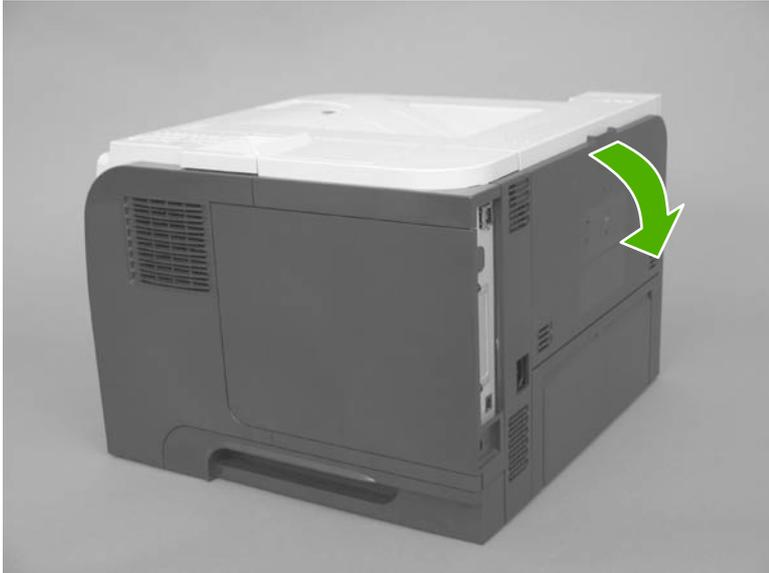
2. Gently pull down on the door and lower the door until it is fully open.
