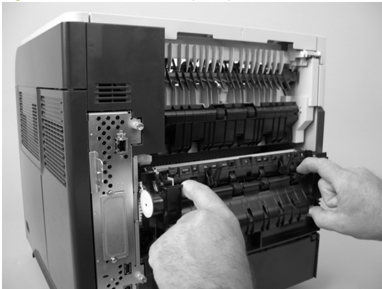
Figure 6-24 Remove the fuser (2 of 2)
