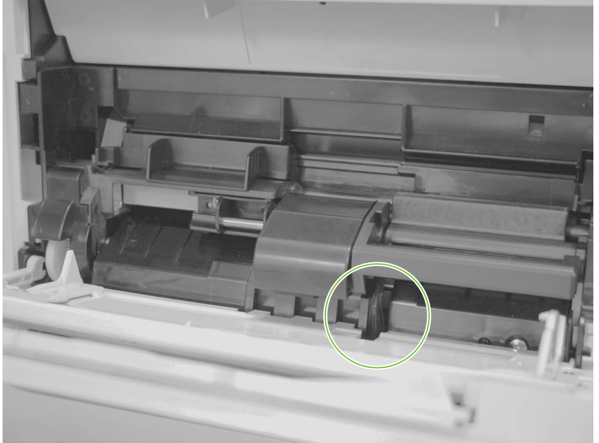
Figure 7-4 Checking the Tray 1 paper present sensor
