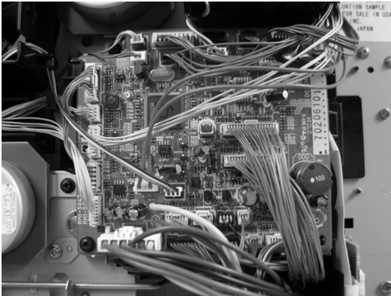
Figure 6-76 Remove the DC controller PCA (1 of 4)
