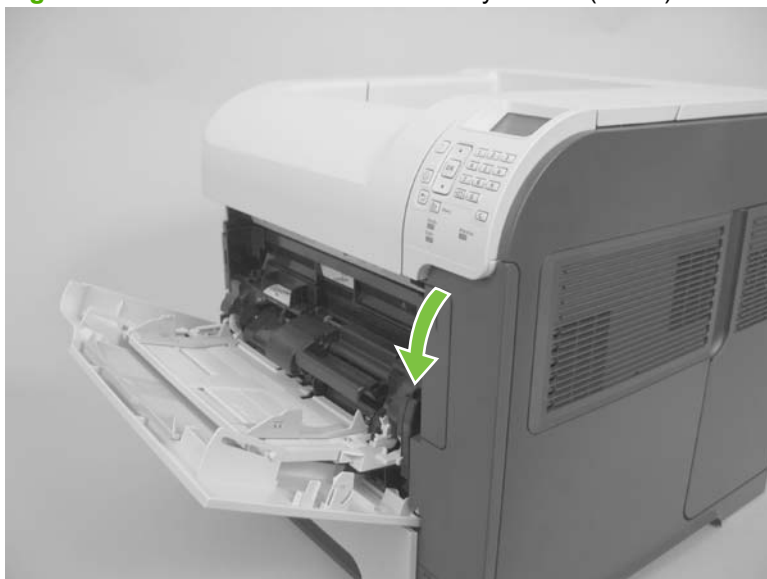
Figure 6-16 Remove the front accessory covers (2 of 2)
