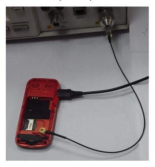
(4) Select proper com port and press "Reconnect" and then press handset's power key.
