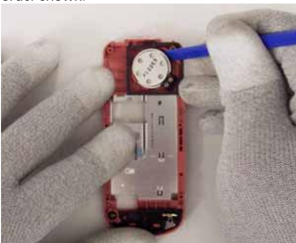
9) Carefully insert the SS-93 at the edge of the tab and lift.
