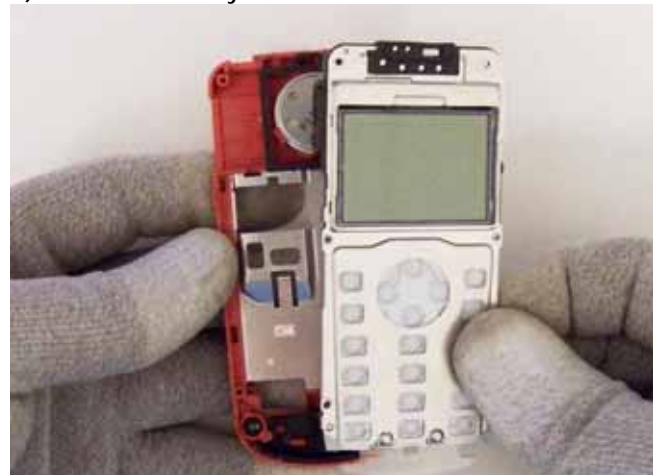
8) Separate the engine module from the D-cover.
