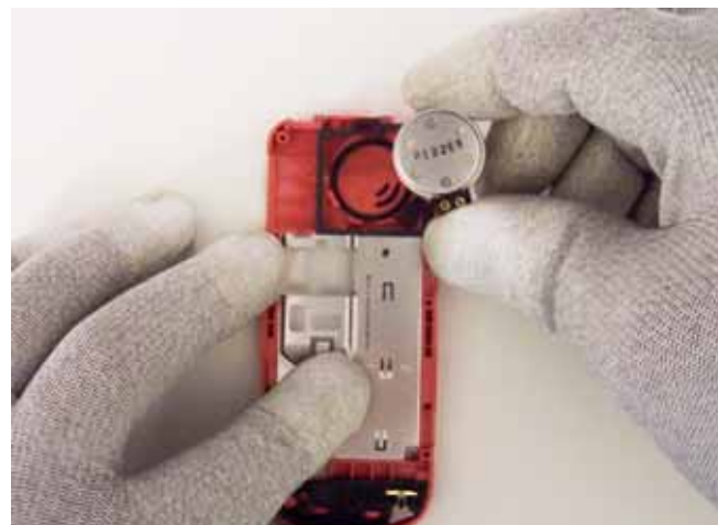
10) Remove the speaker/vibra/earpiece.
