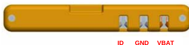
Figure 8 Battery pin order
