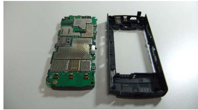
50. The PWB and B-COVER ASSY can now be separated.
