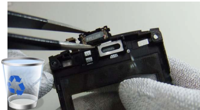
45. Remove the EARPIECE with the tweezers. Discard it. Do not use it again.
