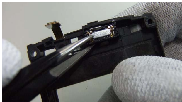
17. Remove the protective tape of the EARPIECE adhesive and assemble it to the A-COVER ASSY as shown.
