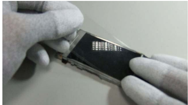
38. Protect the LCM with a protective tape.
