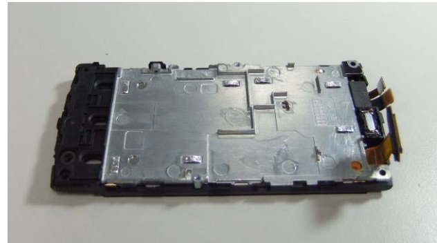
26. The upper module assembly is now complete.
