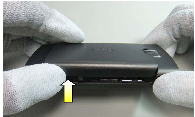
4. Use the opening notch to release the BATTERY COVER.
