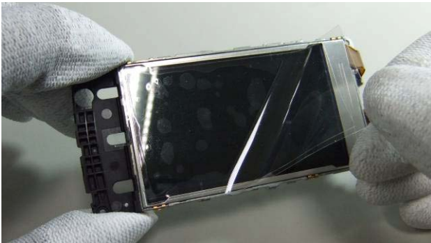
23. Remove the protective tape on LCM and then remove the protective tape on A-COVER ASSY as well.
