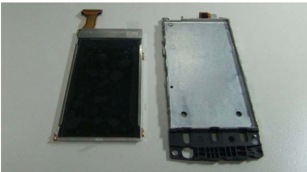
41. The LCM and LCM METAL FRAME can now be separated.
