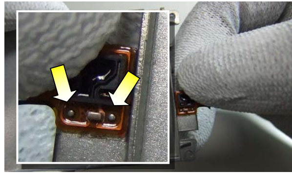
20. Remove the protective tape of the FPC PROXIMITY and fix it on LCM METAL FRAME as shown. Note the two positioning pins on LCM METAL FRAME.
