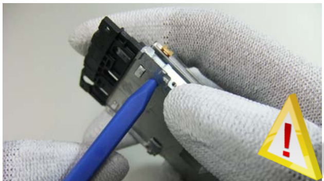
40. Lever out the LCM with SS-93 as shown. Be careful not to bend the LCM.
