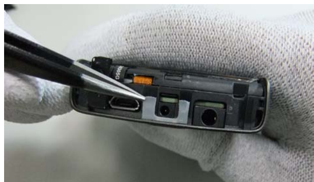
36. Fix the adhesive onto the B-COVER ASSY as shown and remove the protective tape.
