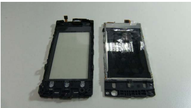
39. The A-COVER ASSY can now be separated.
