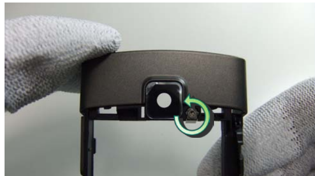
54. Unscrew the TORX+ size 5 screw on B-COVER ASSY as shown. Remove it with the tweezers.
