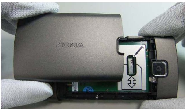
5. Remove the BATTERY COVER. If there is a battery inserted, remove it as well.
