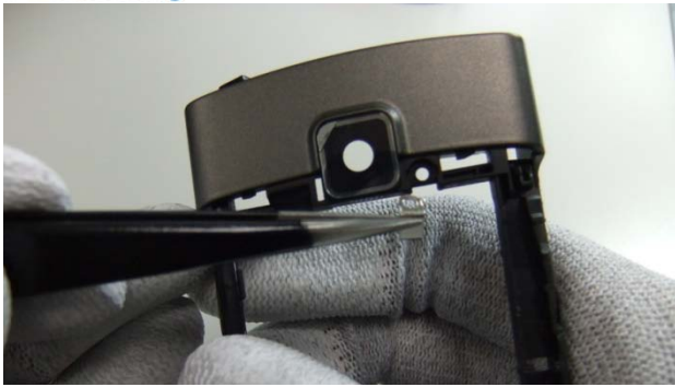
55. Remove the GROUNDING CLIP with tweezers as shown.
