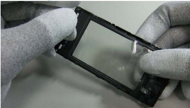
37. Protect the inner side of the lens of A-COVER ASSY with a protective tape.
