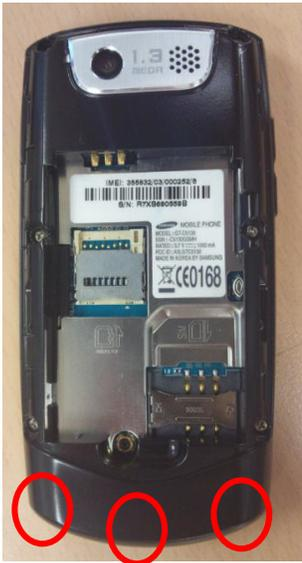
1) Assemble REAR by pressing 3 points from the bottom.
