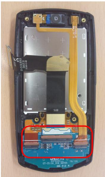
1) Open FPCB connector and disassemble Slide FPCB.
