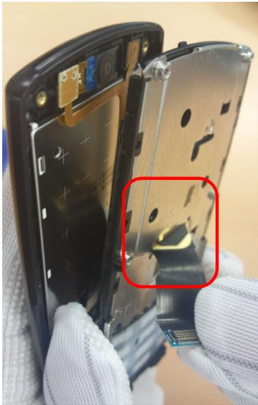
1) Pull the LOWER by lifting it from bottom to top.
