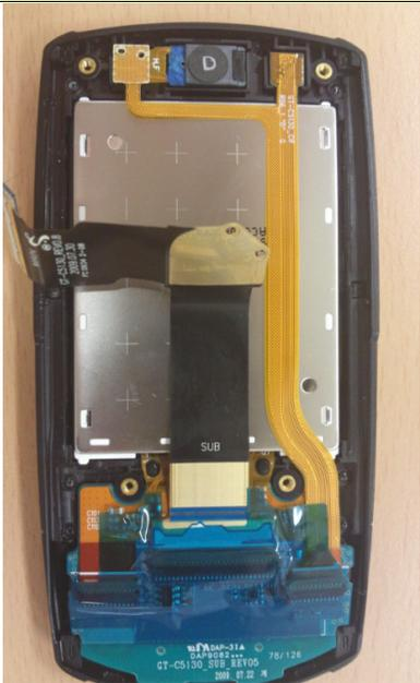
1) Remove green tape and then you can disassemble
