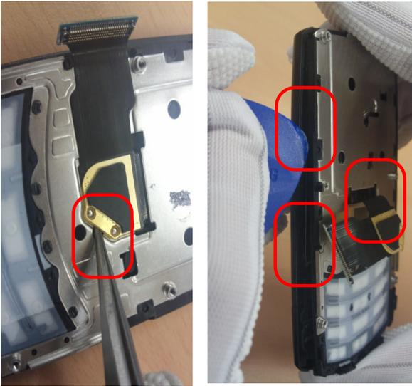
1) Disassemble side of Front locking partl. (2 points)
