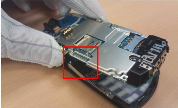
1) Dettach Slide FPCB and Pull PBA by lifting it from bottom to top.
