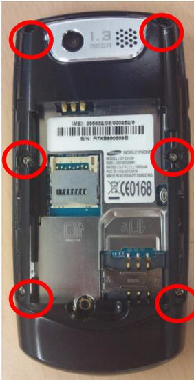
1) Drive Screws at 6 points with torque 1.3 +/- 0.1 Kg/cm<sup>2</sup>.
