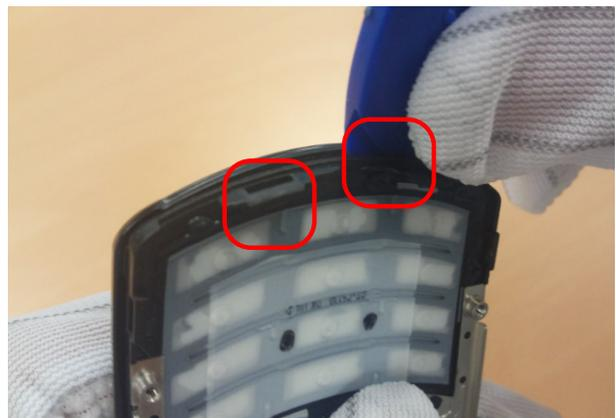
1) Slide up and Disassemble bottom of Front locking part.
