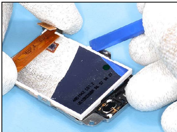
17. Carefully lever out the LCD from the UI SHIELD.
