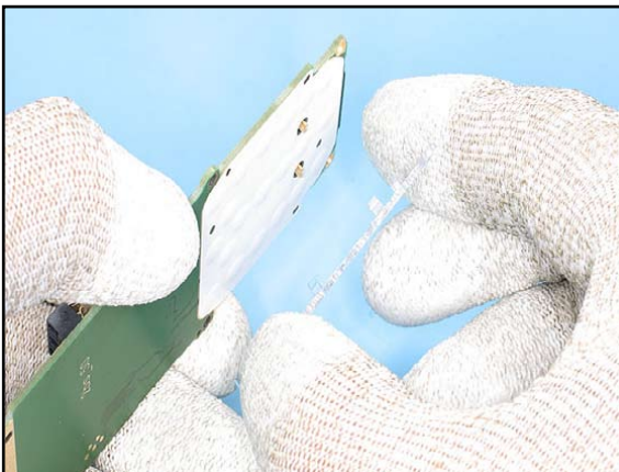
16. If both sides are clearly unlocked, the KEYMAT LIGHT GUIDE ASSY can be removed easily.
