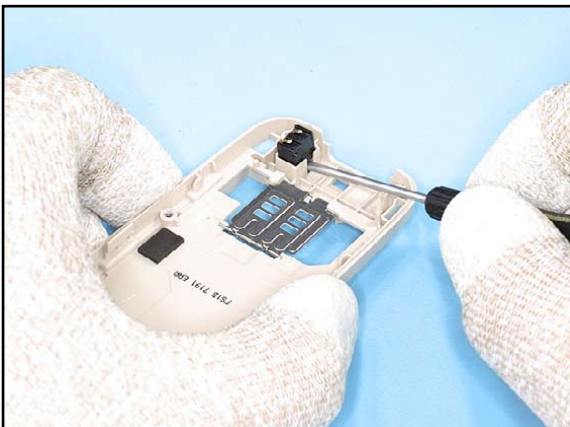
11. Partly ease out the MICROPHONE with the straight bladed screwdriver first, then remove it. Prevent bending the spring contacts and mind the correct placement, if this component should be assembled again.
