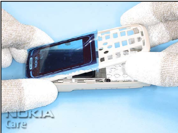
7. Lift up the A-COVER now, beginning from the bottom side.
