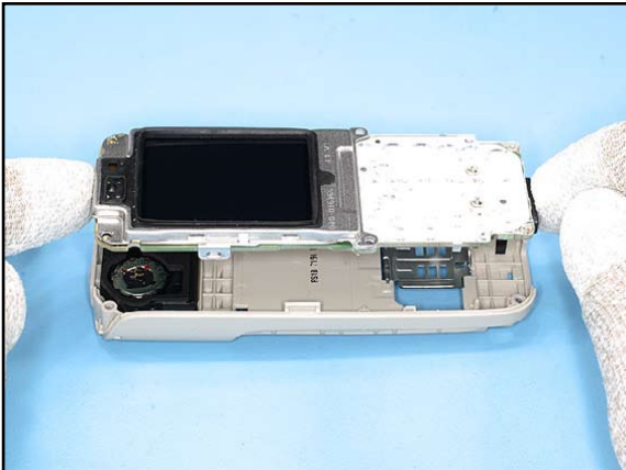
9. Vertically lift out the LIGHT SWAP PWB from the D-COVER ASSY.
