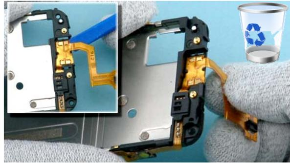
32) Bend the UPPER FLEX ASSY as shown and then use the SS-93 to detach the flex from the deck. The UPPER FLEX ASSY cannot be reused.
