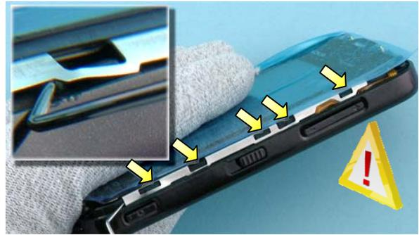
8) Use the dental tool to carefully release the clips holding the TOUCH WINDOW ASSEMBLY.
