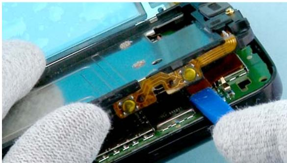
3) Place the UI DECK over the engine board and connect the UPPER FLEX.
