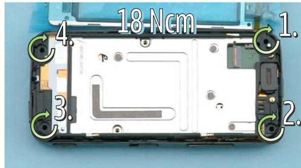
4) Tighten the four TORX + size 6 screws to the torque of 18 Ncm in the order shown.
