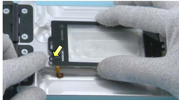
3) Then place the top side of the TOUCH WINDOW ASSEMBLY using the guide of the SS-214.
