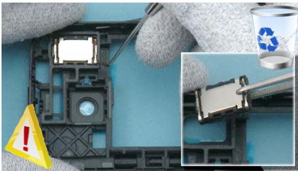
27) Use the dental tool to release the IHF SPEAKER and remove it with the tweezers. Be careful not to damage the IHF gasket! The speaker and the speaker adhesive cannot be reused.
