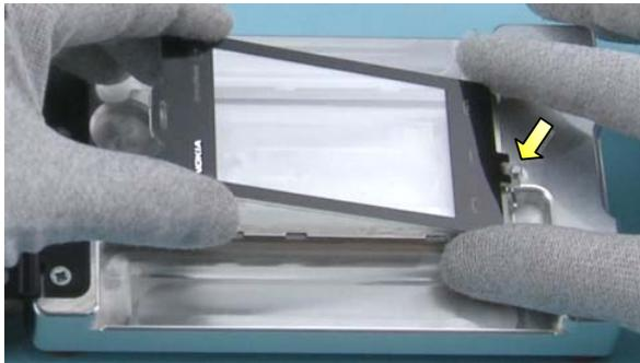
2) Remove protective film from the TOUCH WINDOW ASSEMBLY before placing the assembly. Use the guiding on bottom side to position the assembly correctly.
