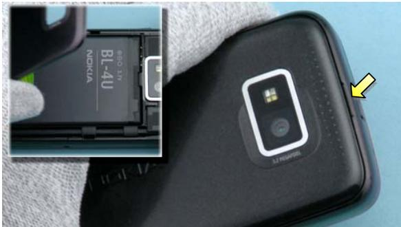
3) To remove the BATTERY COVER, use the finger groove to release the cover. If there is a battery inserted, remove it also.
