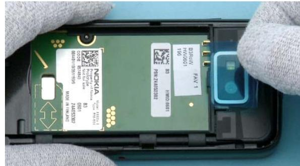
4) Protect the camera lens with protective film.
