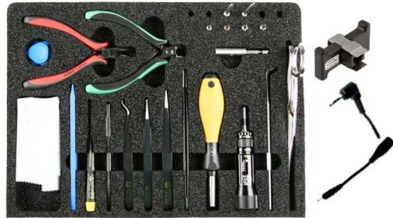
2) You must use the Nokia Standard Toolkit version 2. You will also need the SS-210 camera removal tool, AV plug and the 2 mm charger plug.
