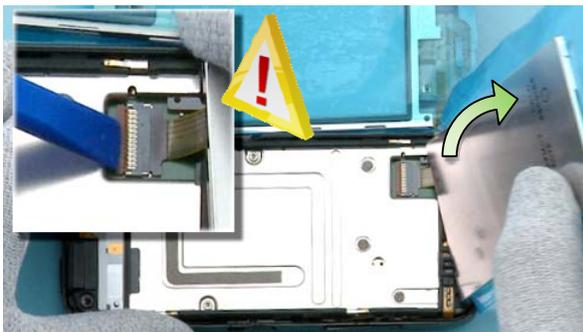
11) Turn the LCD over to gain access to the LCD connector. Then use the SS-93 to unlock the locking mechanism of the LCD connector. While opening the connector, be careful to not to damage the connector!
