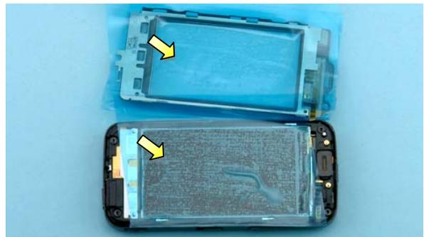
10) Protect the inner side of the TOUCH WINDOW ASSEMBLY and the LCD with protective film.
