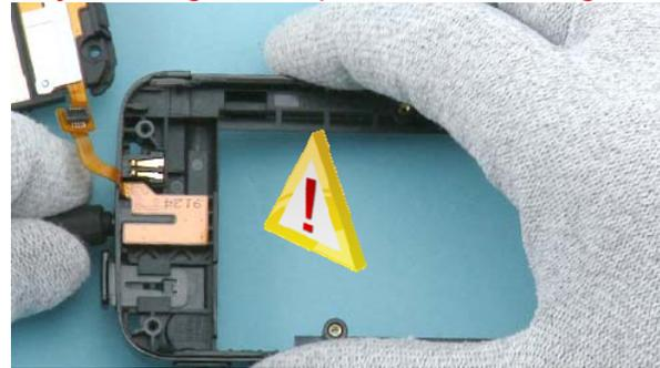
22) Push out the audio connector with the AV plug. Be careful not to damage the audio connector while releasing it - or the flex soldering! Avoid pulling the flex while detaching the AV connector!
