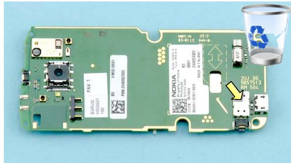
34) Remove also the LNA SHIELD LID from the bottom side of the engine board.
