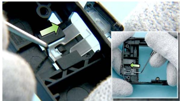
28) Push the end of the USB DOOR with the dental tool as shown.
