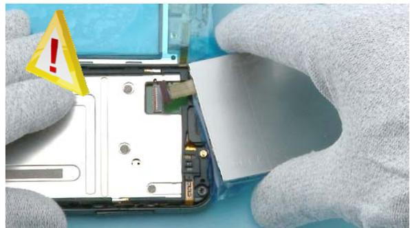
12) Carefully disconnect the LCD connector and remove the LCD.
