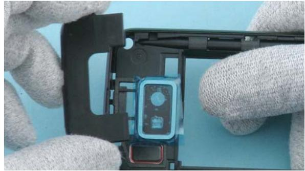
26) Turn the C-COVER over and detach the ANTENNA ASSEMBLY.
