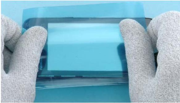
7) Protect the TOUCH WINDOW ASSEMBLY with protective film.
