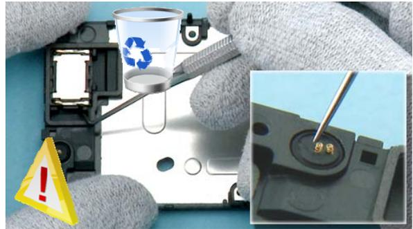
30) Use the dental tool to release the IHF SPEAKER. Be careful not to damage the IHF gasket! The speaker and the speaker adhesive cannot be reused. Also remove the MICROPHONE with the dental tool.
