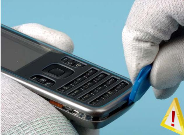
Pull the C-COVER outwards to carefully release the lower side clips.
