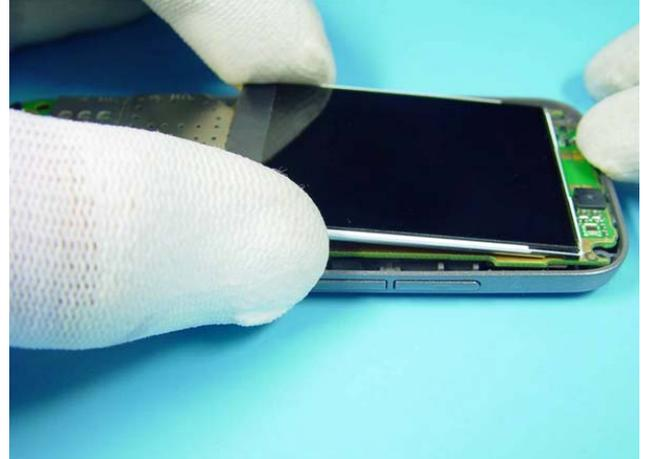
Place the LCD MODULE into the correct position.
