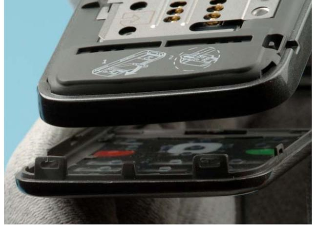
First assemble the lower clips of the A-COVER.
