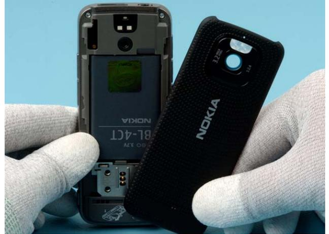
Remove the BATTERY COVER and remove the battery.
