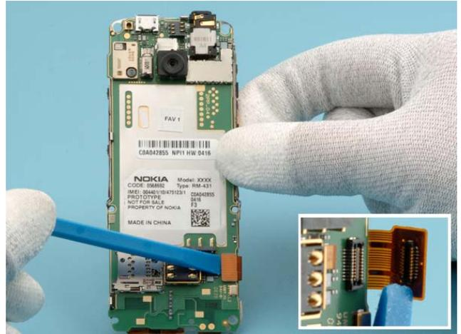
Use the SS-93 tool to release the connector of the UI.
