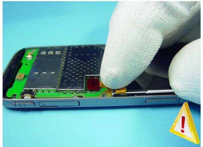
Do not press the LCD FLEX down too hard because it can cause sharp curves and break it.
