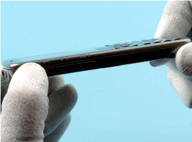
Check that the A-COVER has been closed properly before you tighten the screws.
