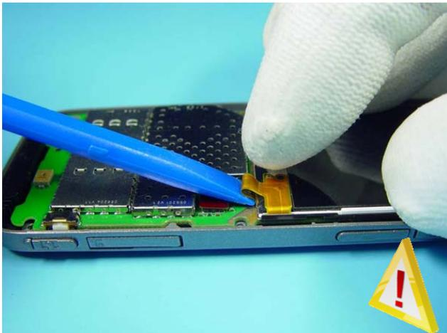
Carefully press the LCD FLEX down.
