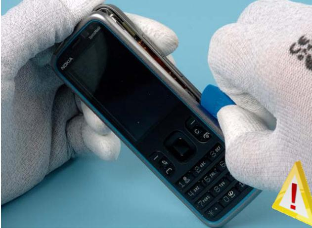
Carefully wedge the SRT-6 tool under the edge of the A-COVER and work carefully around the cover to release the 7 clips. **Note:** Be careful with the clips, they break easily.
