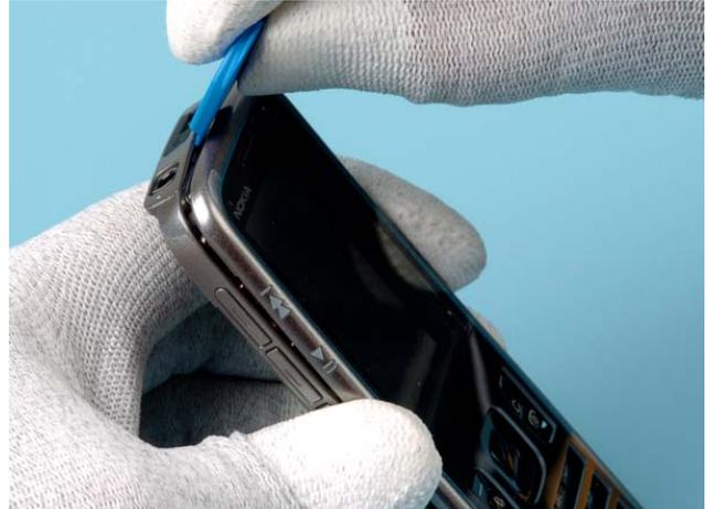
To release the middle clip, first lift the top of the A-COVER.
