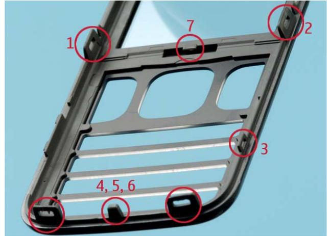
Before removing the A-COVER, make sure that you have released all 7 clips.
