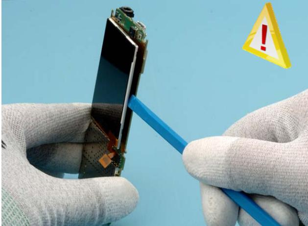
Carefully wedge the SS-93 tool under the LCD MODULE and gently work the tool around the LCD MODULE.
