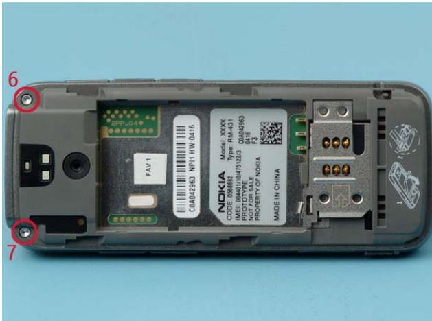
Tighten the two screws to the torque of 13 Ncm in the order shown.
