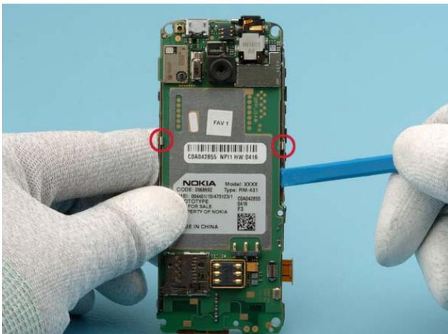
Release the clips on both sides of the PWB.
