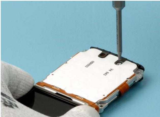
Tighten the screw to the torque of 13 Ncm.
