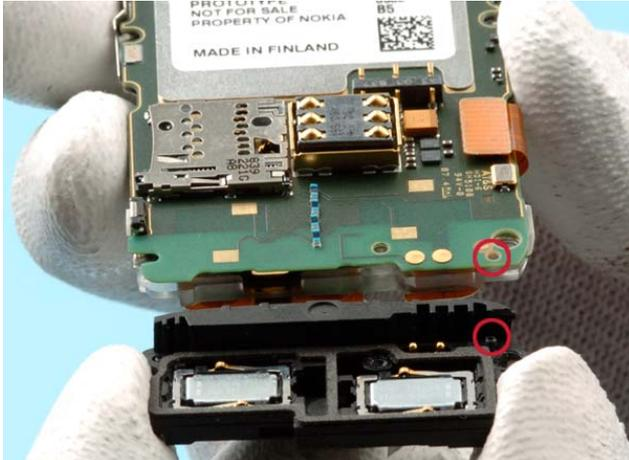
Use the guiding pin in the ANTENNA MODULE and the hole in the PWB when assembling the ANTENNA MODULE.
