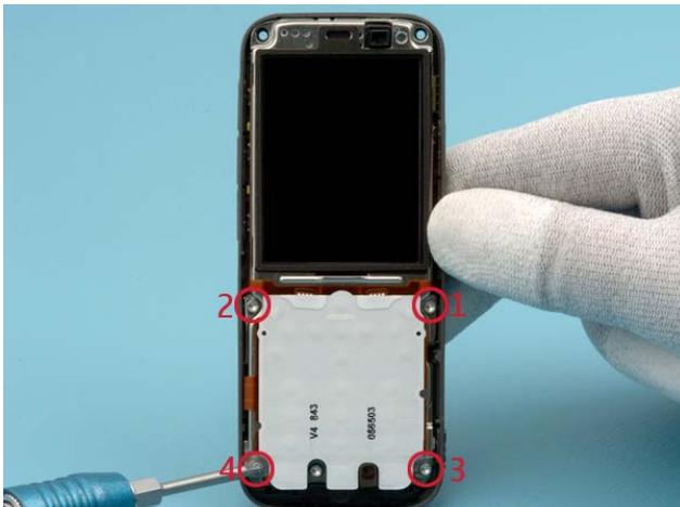
Unscrew the four T6+ screws.
