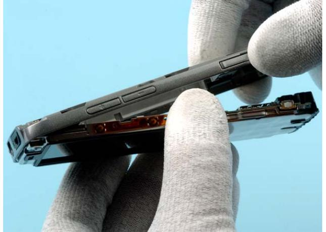
Start assembling the C-COVER from the audio connector.
