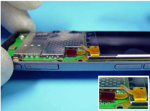
This is the position of the LCD FLEX after the pre-bending procedure. Make sure the connector is secure by pressing it.
