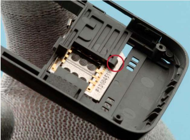
Note that the C-COVER has a clip that you need to press in place from the top of the left speaker.
