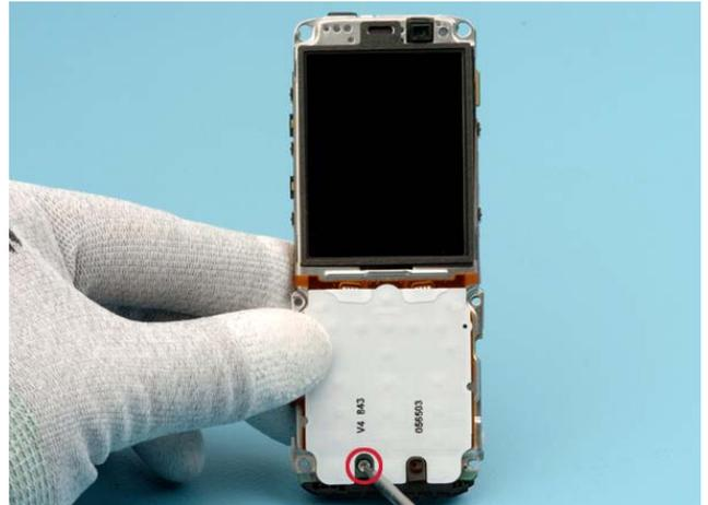
Unscrew the T6+ screw to remove the antenna.
