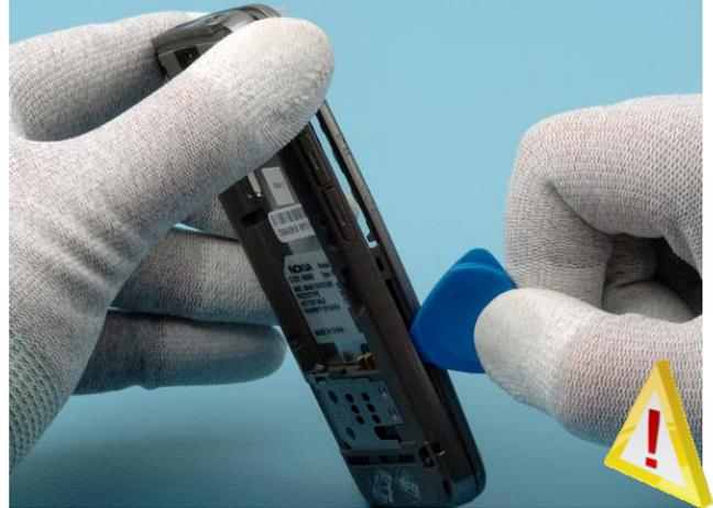
Pull the C-COVER outwards around the cover with the SRT-6 tool when opening the A-COVER.
