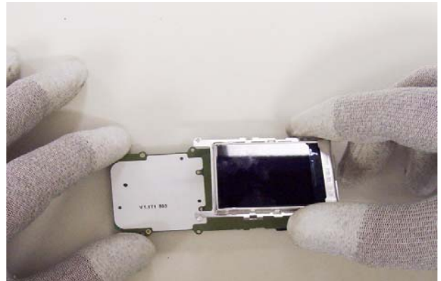
10) Remove UI Shielding and LCD Module.
