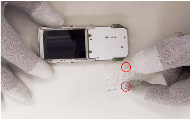
7) Gently release tabs with fingers and remove Keymat Light Guide.
