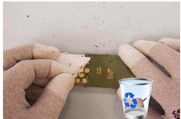
18) Remove the Dome Sheet and discard it.
