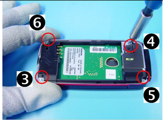
2) Tighten the screws to the torque of 15 Ncm in the order shown.
