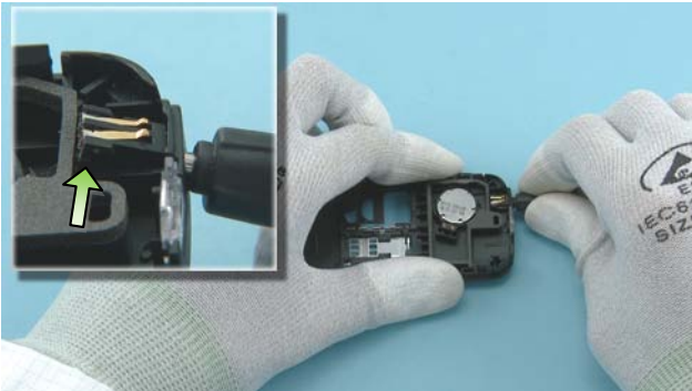
19) Lift up the DC JACK with a DC plug.
