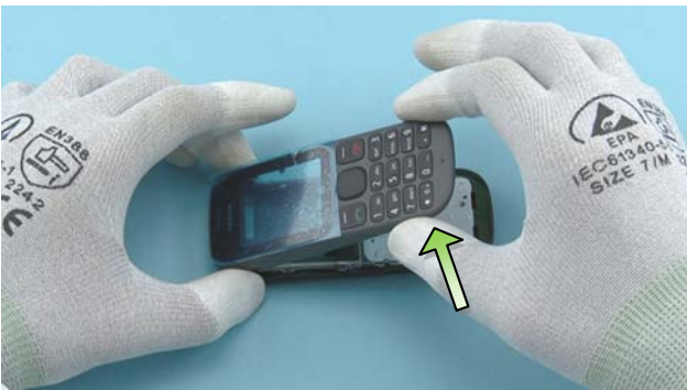
9) Flip the A-COVER open from the bottom side and remove it.
