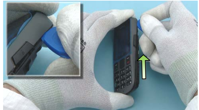
8) Open also the right side of the A-COVER by sliding the SRT-6 to direction shown.
