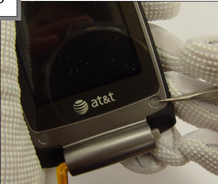
Attach the Screw caps (2 Points)
