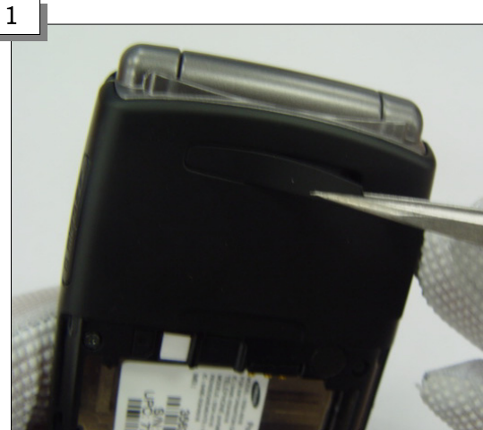
Remove the Rear Screw Deco
