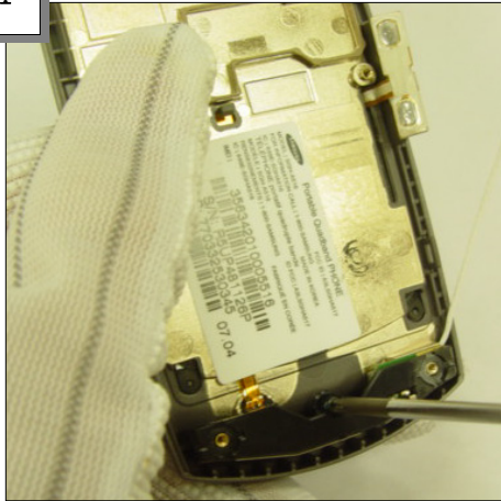
Join the Screw to the Antenna
