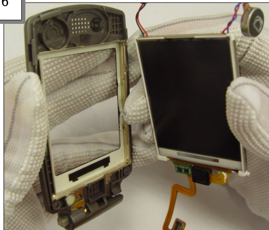
Disjoint the LCD from the Lower
