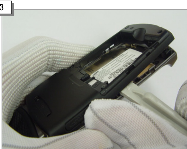
Open the side with a knife (from the bottom)
