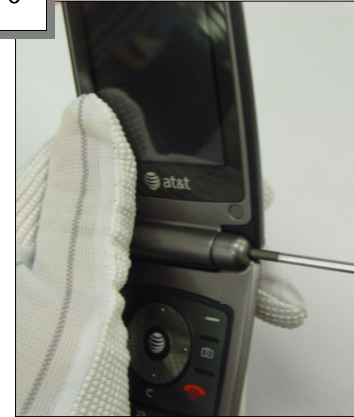
6 Press the Hinge with a lever
