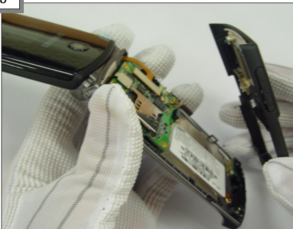
Open the side with a knife (from the bottom)
