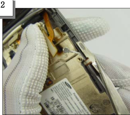
2 Tear the Sidekey Dome off
