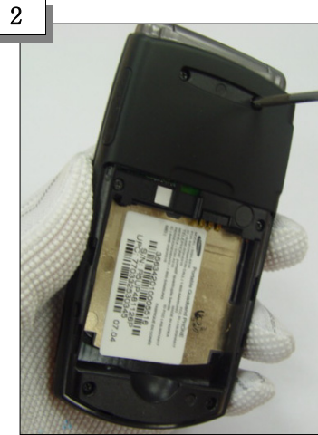
Remove the Screws (6 Points)
