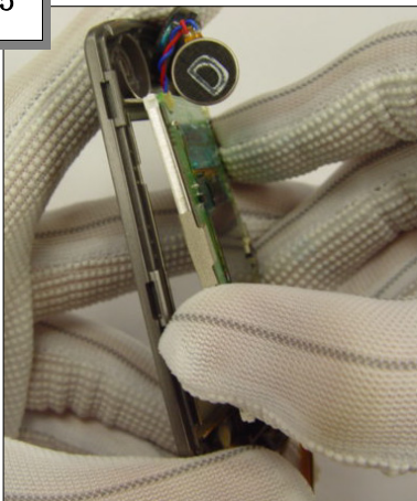
Tear the LCD off
