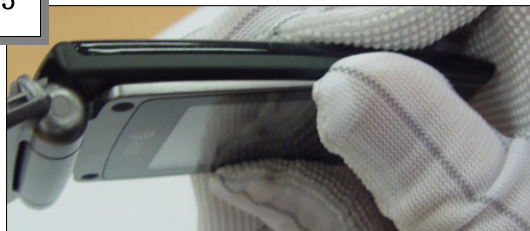
Assemble the middle of the Upper
