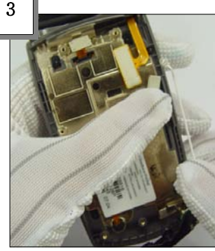
3 Disjoint the Antenna & Wire
