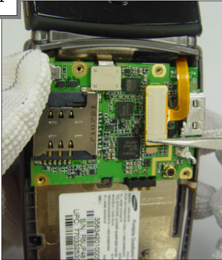
Disjoint the LCD Connector
