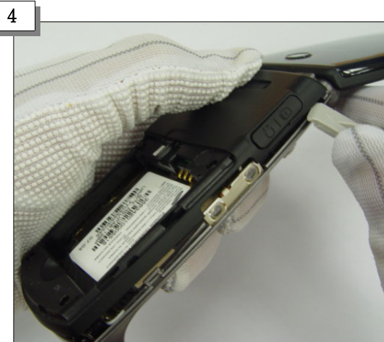
Open the side with a knife (to the top)
