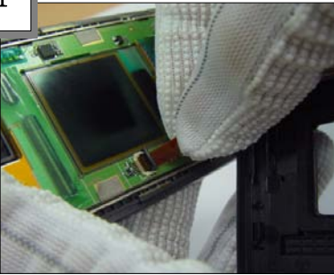
Join the Touch key to the connector
