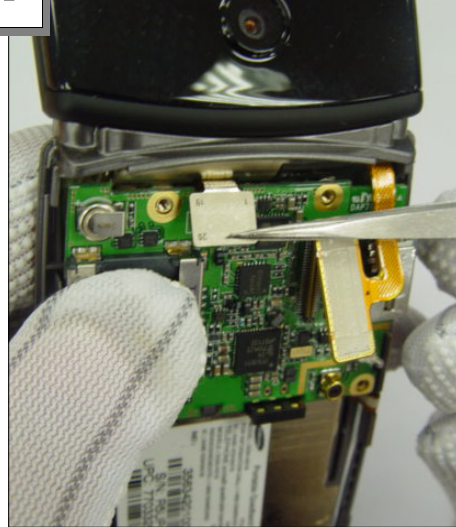
Disjoint the KEY Connector
