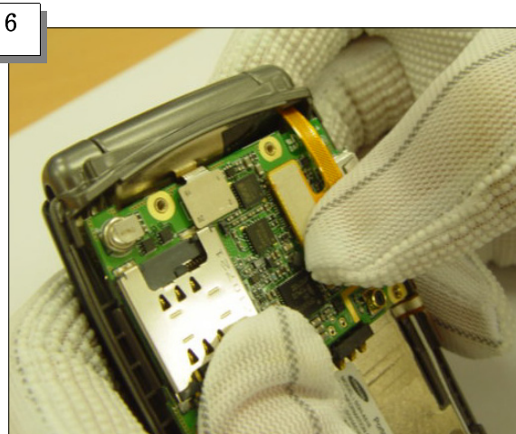
Assemble the LCD Connector
