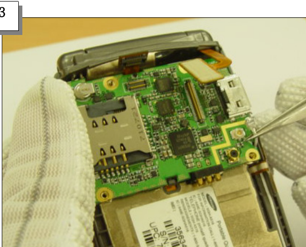
Join the PBA to the Front (Put the Antenna wire in the hole in the PBA)
