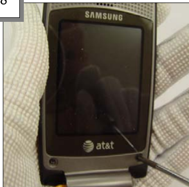
Tighten the Screws (2 Points)
