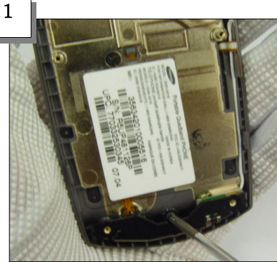
1 Remove the Screw from the Antenna
