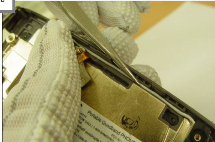
Arrange the Antenna wire in the guide hole
