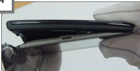
Join the Upper to the bottom of the Lower
