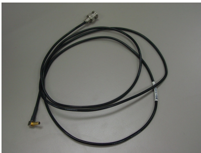
3-3-1. RF Test Cable (GH39-00397A)
