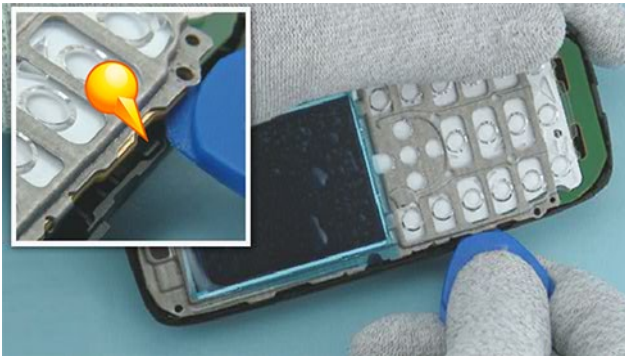
17) Release the clip from the other side of the device and lever out the ENGINE BOARD with the DISPLAY, UI SHIELDING and KEYMAT LIGHT GUIDE.
