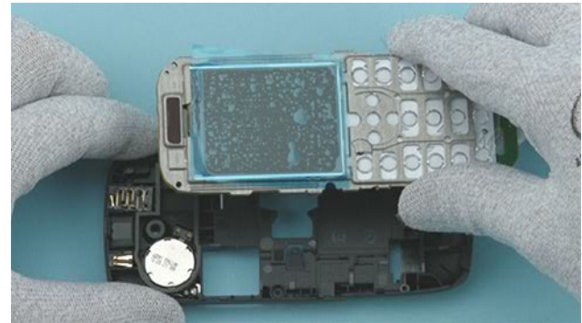
18) Separate the ENGINE BOARD with the DISPLAY, UI SHIELDING and KEYMAT LIGHT GUIDE.
