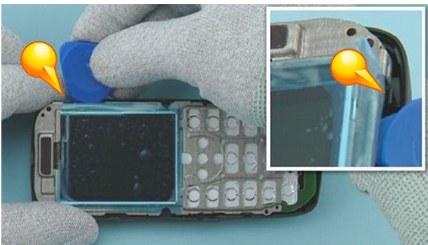
15) Release the shown clip holding the ENGINE BOARD with the SRT-6.
