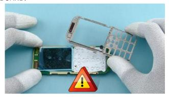
16) Separate the UI SHIELDING. Note that the DISPLAY is attached to the ENGINE BOARD only with the DISPLAY flex. Be careful not to damage the DISPLAY FLEX.
