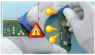
14) Use the SRT-6 to open the three shown clips holding the UI SHIELDING. Be careful not to damage the small components on the ENGINE BOARD.
