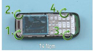
3) Tighten the four TORX+ size 4 screws to the torque of 14 Ncm in the order shown.
