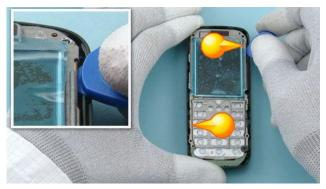
12) Open the two shown clips with the SRT-6 to release the ENGINE BOARD.
