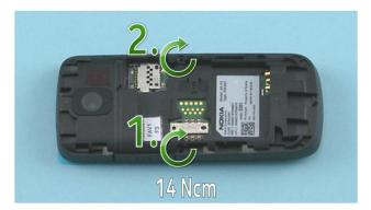
4) Tighten the two TORX+ size 4 screws to the torque of 14 Ncm in the order shown.
