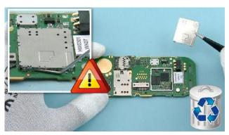
20) Lever out the BB SHIELDING LID with the dental tool and remove it with tweezers. Do not use it again. Discard it.
