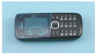
3) Protect the A-COVER window with protective film.
