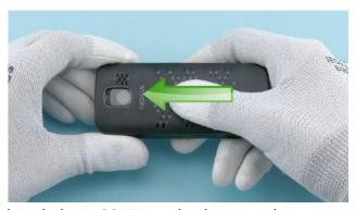
4) Push the B-COVER to the direction shown to release it.
