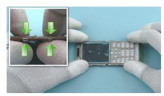
2) Place the UI SHIELDING to the ENGINE BOARD. Press the UI SHIELDING gently until the clips attaching it to the ENGINE BOARD snap.
