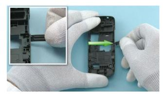
25) Pull out and remove the SIM DOOR.
