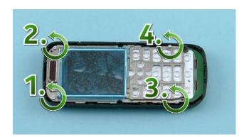
11) Unscrew the four TORX+ size 4 screws in the order shown.
