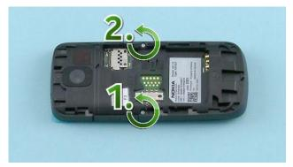
6) Unscrew the two TORX+ size 4 screws in the order shown.
