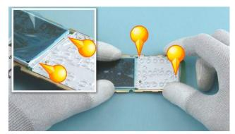
1) Align the KEYMAT LIGHT GUIDE to the ENGINE BOARD using the two shown guiding pins. Before placing the UI SHIELDING check that the DISPLAY is aligned correctly and it is not on top of the KEYMAT LIGHT GUIDE.
