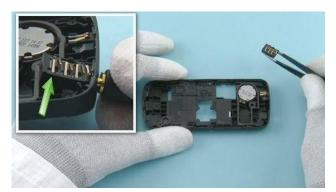
22) Use an AV plug to lift up the AV JACK. Remove the AV JACK with tweezers.
