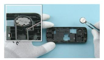
24) Release the MFD BARD with the dental tool and remove it with tweezers.
