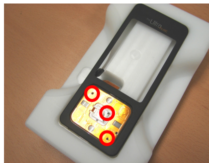
&lt;Attach the key FPCB on MP3 cover&gt;
