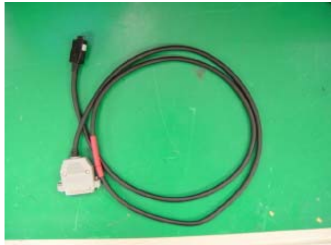
8-6 Test Jig Cable(GH39-00399A)
