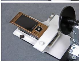
Use the Pressure Tool to press the Keyboard for 10 seconds.
