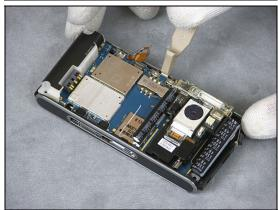
Use a Flex Film Assembly Tool to attach the connector to the Main PBA
