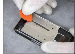
Use a Guitar Pick to peel off the Foil Adhesive 0.048 mm Flex Flip from the PBA Key Flex Flip Complete
