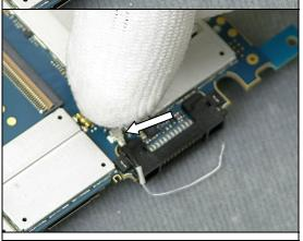
Use a Front Opening Tool to attach the BT/WLAN Antenna
