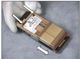
Use a Screwdriver with JCIS Bit to remove the two Screws 2.3x1.4.
