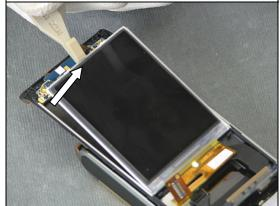
Use a Front Opening Tool to remove the Display 2.41 TFT.
