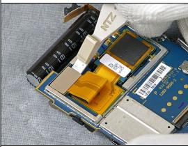
Use a Front Opening Tool to release the five snap hooks
