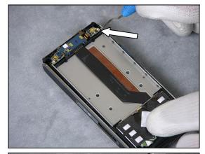
Use a Flex Film Assembly Tool to remove the Foil Adhesive LCD Support, right
