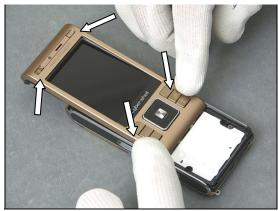
Use your fingers to slide and position the Cover Flip Front to make the two Screw 2.3x1.4 holes visible through the two holes in the Cover Base Rear Assembly.
