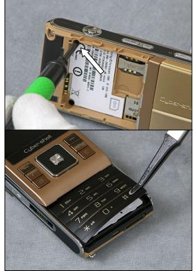
Use a Flex Film Assembly Tool to remove the Keyboard
