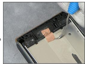
Use a Dentist Hook to remove the Foil Adhesive Double Side GPS Shieldcan
