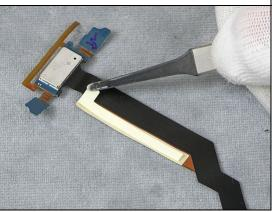
Use a Flex Film Assembly Tool to remove the protection tape from the Foil Adhesive 0.048 mm Flex Flip
