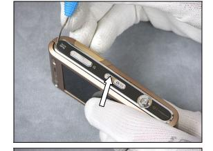
Use a Flex Film Assembly Tool to remove the Right Sidepanel Top
