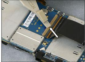
Use a Front Opening Tool to close the connectors lock
