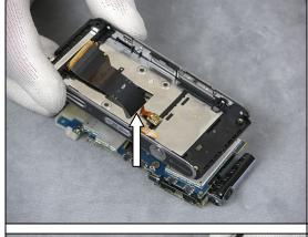
Use A Flex Film Assembly Tool to Loosen the Slider FPC Assy Adhesive from the 100 pin FPC connector
