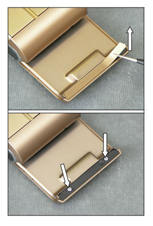
Use a Screwdriver with JCIS Bit to remove the two Screws 4.0x1.4.
