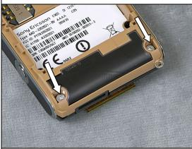
Use a Guitar Pick to loosen the Cover Base Rear Assembly on three sides
