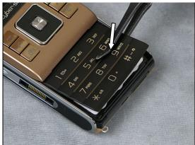
Place the phone on the Keyboard Pressure Tool as the picture shows. Set the Pressure Tool to 50 N.
