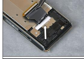
Use a Screwdriver with JCIS Bit to remove the four Flat Head M1.4x1.7
