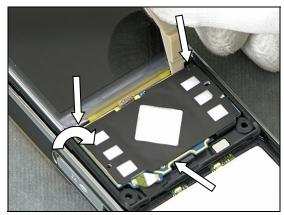
Use a Front Opening Tool to disconnect the LCD FPC Connector
