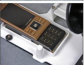
Use the Pressure Tool to attach the Keyboard
