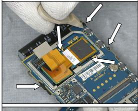
Turn over the Main PBA and use a Front Opening Tool to disconnect the Flash Complete from the Main PBA
