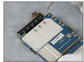
Use a Front Opening Tool to disconnect the Camera Connector from the Main PBA
