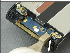
Use a Front Opening Tool to loosen the GPS part of the Board.
