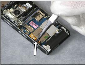
Use a Pair of ESD Tweezers to loosen the BT/WLAN Antenna
