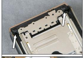
Use a Screwdriver with T6 Bit to remove the two Screws Torx 5.3x1.6.
