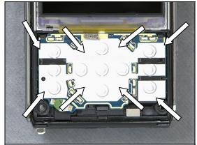
Use a Flex Film Assembly Tool to position the Light GU Navigation
