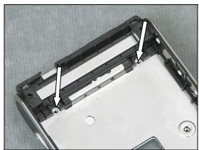
Use a Screwdriver with JCIS Bit (torque 11Ncm) to insert and tighten the four Flat Head M1.4x1.7.
