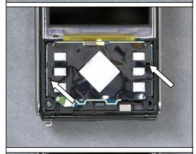
Use your fingers to attach the Light Gu Navigation DO NOT ATTACH THE LIGHT GU NAVIGATION BY PRESSING ON THE BUTTONS!
