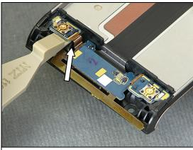
Use a Front Opening Tool to loosen the Key A part of the Board.
