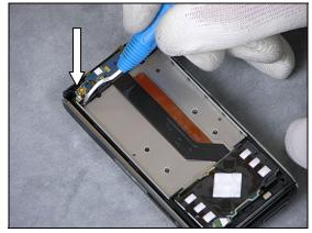
Use a Flex Film Assembly Tool to remove the Foil Adhesive LCD Support, left
