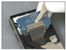
MAKE SURE TO ALIGN THE PBA KEY FLEX FLIP COMPLETE PROPERLY TO THE COVER REAR ASSY!
