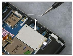
BE VERY CAREFUL NOT TO DAMAGE THE MAIN PBA SWITCHES WHEN LOOSENING THE MAIN PBA!
