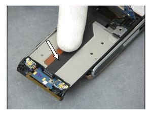
Use a Flex Film Assembly Tool to position the Foil Adhesive Single Side 0.15 mm Flip Tape
