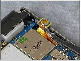
Use a Flex Film Assembly Tool to position the Key Camera Flex in the camera key switch supporter
