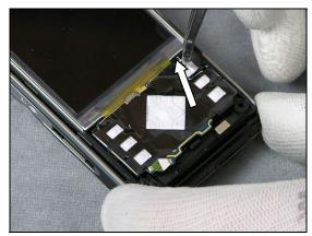
Use a Flex Film Assembly Tool to remove the Dome Foil Flip
