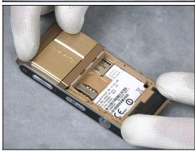
Use a Screwdriver with T6 Bit to assemble the two Screws Torx 5.3x1.6 (torque 11Ncm).
