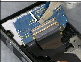
Use a Flex Film Assembly Tool to disconnect the Slider FPC Assy from the PBA Key Flex Complete
