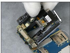
Locate the five snap hooks and use your fingers to snap on the Flash Complete.
