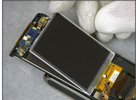
Attach the connector to the PBA Key Flex Flip Complete
