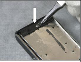
Use a Flex Film Assembly Tool to position the Foil Adhesive Conductive GPS ESD protection tape
