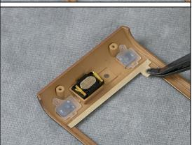
Use a Flex Film Assembly Tool to remove the protection tape from the Foil Adhesive Conductive 0.05 mm protection tape, front
