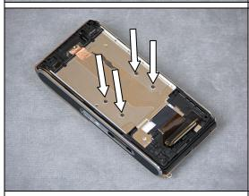
Use a Flex Film Assembly Tool to loosen the Slider PPC Assy from the back of the Cover Rear Assembly
