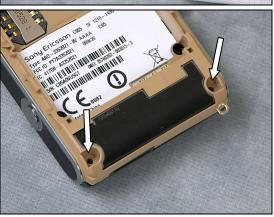
Use a Screwdriver with T5 Bit to assemble the two Screws Torx 5.0x1.6 (torque 11Ncm).
