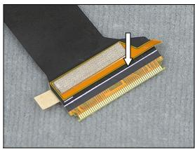
Attach the Slider FPC Assy to the Main PBA..
