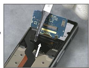
Use a Front Opening Tool to unsnap the PBA Key Flex Flip Complete connector
