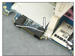
Use a Front Opening Tool to disconnect the BT/WLAN Antenna.
