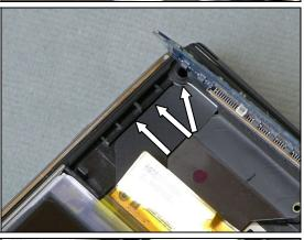
Locate the three snap hooks and use your fingers to flip over and place the PBA Key Flex Flip Complete.
