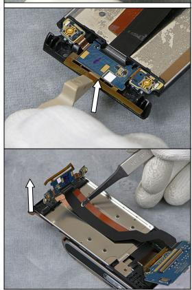
Use a Flex Film Assembly Tool to remove the PBA Key Flex Flip Complete
