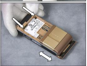
Use a Screwdriver with JCIS Bit (torque 11Ncm) to insert and tighten the two Screw 2.3x1.4.
