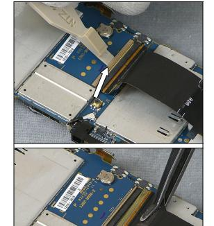
Use a Flex Film Assembly Tool to remove the Slider FPC Assy from the Main PBA
