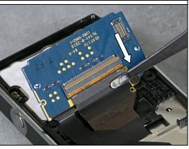
Use a Front Opening Tool to loosen the GPS Antenna.
