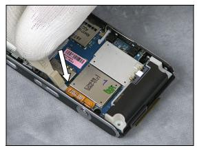
Use a Flex Film Assembly Tool to pull the Numeric Key Foil out of the camera key switch supporter.
