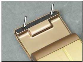
Use a pair of ESD Tweezers to position and attach the Foil Flip Inner.
