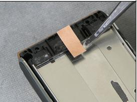
Use a Flex Film Assembly Tool to attach the Foil Adh Conduct GPS ESD protection tape
