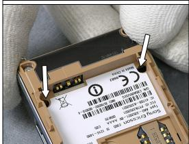
Use a Guitar Pick to loosen the Cover Flip Front on both sides.
