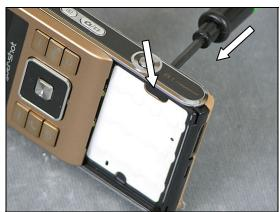
Use Screwdriver to remove the Cap Numeric keyboard on the opposite side.
