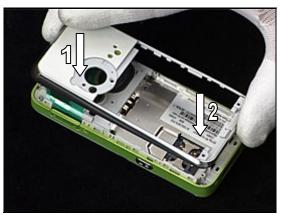
Press down the bottom end of phone to secure snap hooks as shown in picture.
