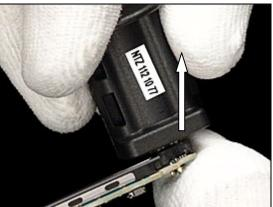
Remove QCIF VGA Camera by using tweezers.
