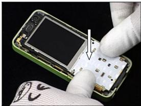
Press down on *PCBA Assy* to secure into the *Main Frame Assembly* at the top end of phone second.
