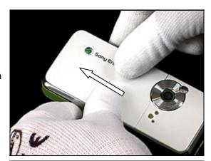
Grip Battery Cover with fingers and lift off Battery Cover.
