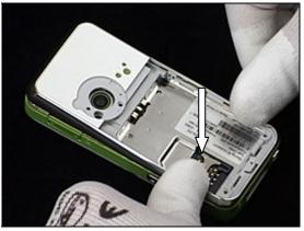
Press down the top end of phone to secure snap hooks as shown in picture.
