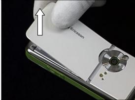
Grip *Battery* as shown in picture and lift up to release the battery.
