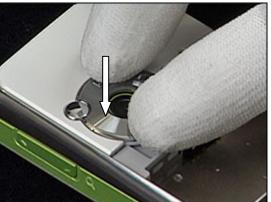
Press down with fingers to secure Camera Ring Assembly.
