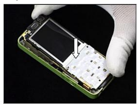
Press down *PCBA Assy* to secure into the *Main Frame Assembly* at bottom end first.
