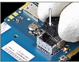
Press down the *Camera 2Mega Pixel* into the camera socket using fingers.
