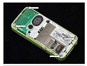
Insert guitar pick tool as shown in picture and unlatch snap hooks along the side of the phone as shown by the arrow.
