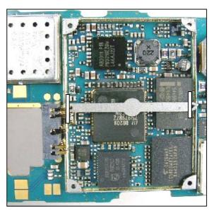
Replace the *quartz crystal* component. Use a soldering iron.
