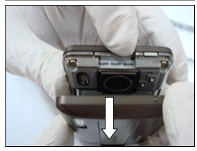
Release the *battery* at the bottom and remove it.
