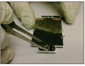
Press the *ear speaker* evenly to be inserted into the speaker hole properly
