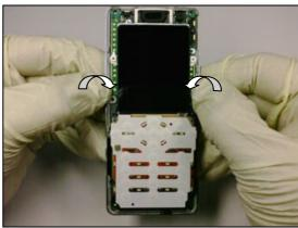
Install two silver screws with torque screwdriver at 11 Ncm with a JCIS.
