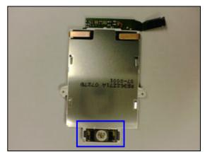
Push the *ear speaker* upward with finger as shown in the picture.
