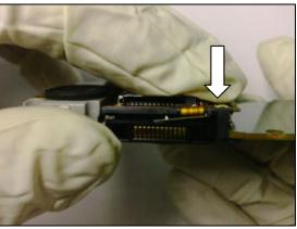
Press the *Keypad support plate* down to make it snap to *M2 SIM assembly.*
