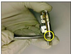
Carefully lift up the LCD module.
