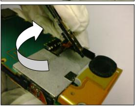
Open the *M2 SIM assembly connector* carefully. Take care not to damage the FPCB.
