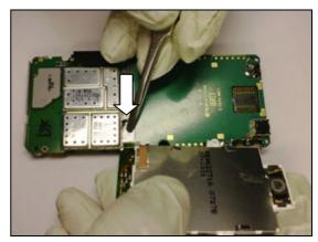
Press the bar on the connector towards the connector by finger evenly to connect completely.
