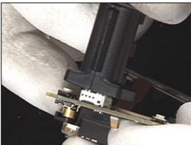
Use tweezers to remove the VGA camera
