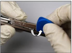
Separate the front cover assembly from the module.
