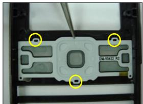
Carefully press to attach the *keypad assembly Navi* to the *front cover*.
