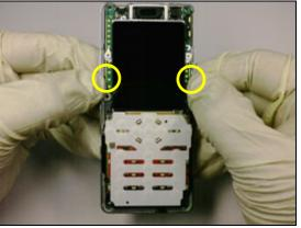
Grab the *frame assembly* by one hand and carefully push the *PCBA unit* up by the other hand as the picture.
