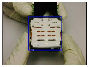
Release the snap between *Keypad support plate* and *M2 SIM assembly* with Opening tool or Blunt pair of tweezers.
