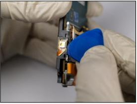
Carefully open the *Key support plate connector* with blunt pair of tweezers and avoid damaging the FPCB.
