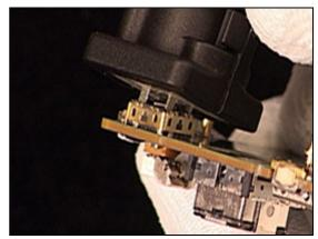
Push the VGA camera tool to bottom and wiggle the tool side to side before lifting the tool up.
