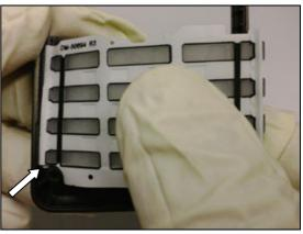
Band the *Keypad assembly Numeric* and insert it to the other side as shown in the picture.
