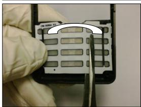
Carefully press to attach the *keypad assembly Numeric* to the *front cover*
