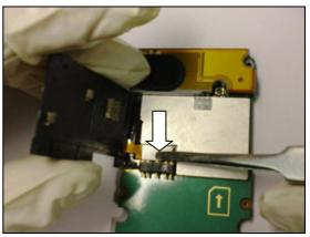
Press the *M2 SIM assembly* down onto the *PCBA unit* to snap together.
