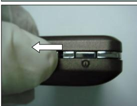
Lift the *battery cover assy* down and release it from the *frame assembly*.
