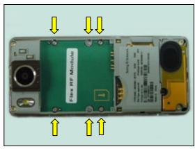
Install four golden screws (*marked with a red arrow*) with torque screwdriver at 17 Ncm with a T6 bit.
