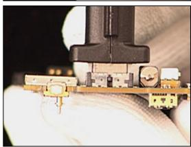
Use tweezers to remove the 3Mpixel camera
