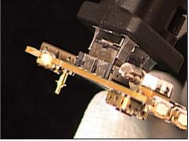
Push the 3Mpixel camera tool to bottom and wiggle the tool side to side before lifting the tool up.
