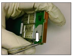
Use your finger to remove the Antenna box from PCBA unit.
