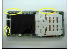
Assemble the *Front cover* and *PCBA unit* using the order shown.
