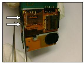
M2 SIM assembly is attached with snaps to the PCBA unit and Keypad support plate respectively. Release the snaps with blunt pair of tweezers.
