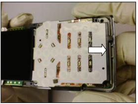
Press the PCBA unit to snap to the Flame assembly.
