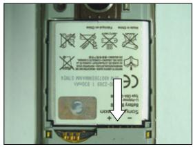
Align the bottom of the *Battery cover assembly* with the guide line of the *Flame assembly*.
