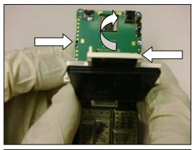
Lock the LCD module's snap to PCBA unit.
