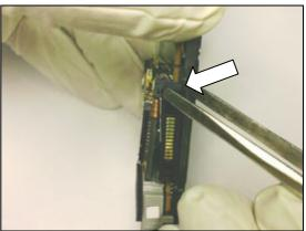
Lift the M2 SIM assembly from PCBA unit carefully.
