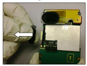
Use the tweezers to remove the system connector gasket.
