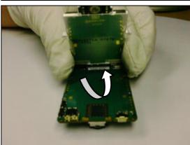
Use the flex film opening tool to remove the flex film.
