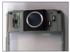
Use the blunt pair of tweezers to remove *Camera cap* from the *Frame assembly*.
