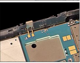
Place the Bluetooth Antenna underneath the plastic clip on the Inner Frame using a dental hook.
