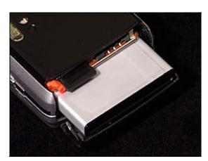
Remove the two screws (Torx T4). You might have to slide the orange battery clip to the side to be able to access the left screw.
