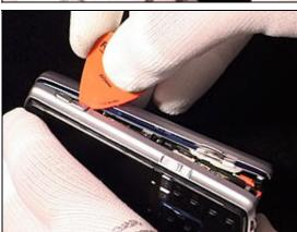
Once all snap hooks on both sides have been released, carefully lift the rear cover in the direction of the arrow and remove it.
