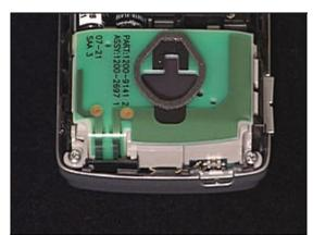
Carefully release the first Antenna snap hook using the guitar pick.
