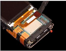
**BE CAREFUL NOT TO DAMAGE OR SCRATCH THE LCD**Carefully insert the guitar pick under the white LCD carrier and loosen the LCD. Remove the LCD.
