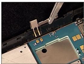
Press the Bluetooth Antenna into position in the Inner Frame.
