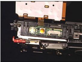
Release the Keyboard Flex BtB Connector using the Nylon pointer.
