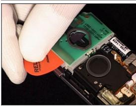
Carefully release the second Antenna snap hook on the other side. Mind the angle of the guitar pick as shown in picture.
