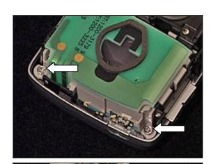
Position the Back Cover Assembly as shown in picture.
