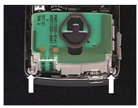
Carefully release the Front Cover snap hooks using the guitar pick.
