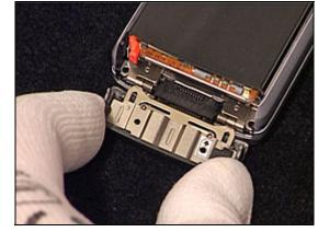
Insert and tighten the two screws (Torx T4 15Ncm).
