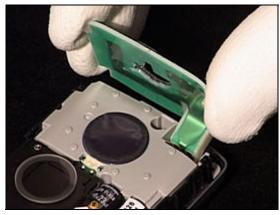
BE CAREFUL NOT TO DAMAGE OR SCRATCH THE PLASTICS AND THE CAMERA SWITCH!
