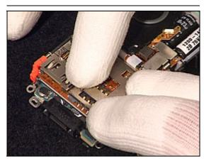
Insert the Flex Film under the plastic clip on the Inner Frame.
