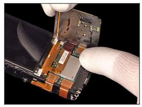
Put the Key FPC in place and gently press it until it snaps into position underneath the three snap hooks of the Inner Frame.
