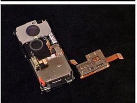
**BE CAREFUL NOT TO DAMAGE THE SIM/COMBO READER**Remove the SIM/COMBO Reader using the guitar pick.
