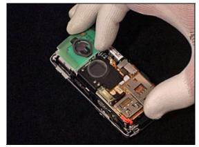
Once the core unit has been positioned inside the Front Cover Assembly, carefully press all four sides of the core unit at the same time. Make sure it has snapped into position into all 4 snap hooks of the Inner Frame.
