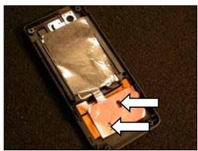
Insert one side of the LCD into its cavity in the new back cover as shown.
