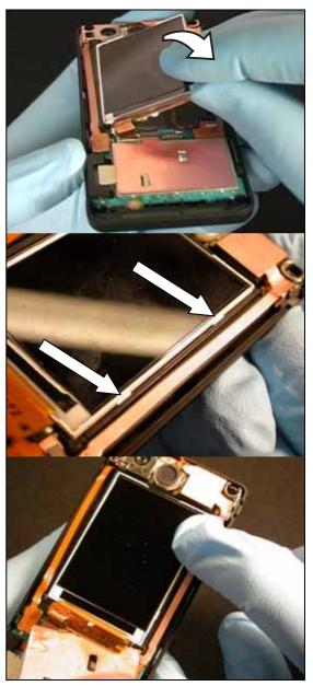
Make sure the LCD is fully seated and that there are no gaps along either side.
