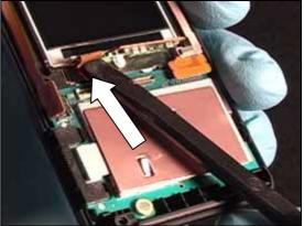
Insert one of the corners of the plectrum into the seam along one side of the LCD in the location shown.
