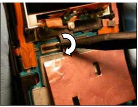
The LCD's flex connection is completely seated in the ZIF connector when the two tabs on the flex are against the ZIF connector.
