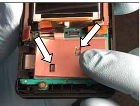
Connect the two camera flex assembly connections to the circuit board.
