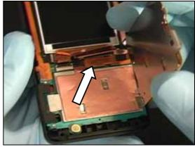
Insert the camera switch portion of the dome foil assembly into place between the circuit board and camera key.
