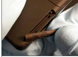
Locate the hole where the tab portion of the memory stick cover inserts through back cover.
