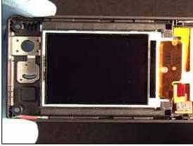
On the old back cover, slide the flat portion of a pry tool between the antenna and the back cover near the screw hole indicated.
