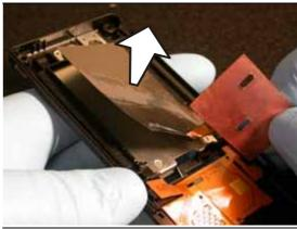
Remove the heat spreader from the old back cover.
