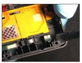
Lift the end of the antenna the pry tool is under.
