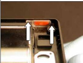
Using style 2A tweezers pull the camera key from its opening in the old back cover.
