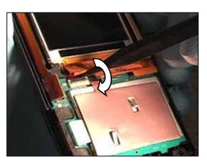
Use the nylon pointer to push the LCD flex film out of its connector toward the LCD.
