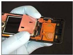
Insert the circuit board into the back cover as shown so that the battery connector inserts into its opening in the back cover first.
