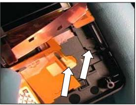
Lay the rest of the SIM flex film down in the back cover so that the SIM connector and memory stick socket are positioned within their alignment features.
