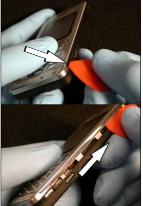
Slide the plectrum down the seam of the phone until the latches along that side are released.
