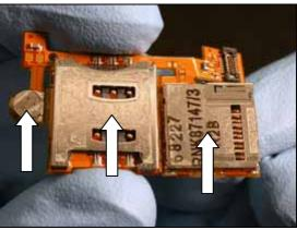
Position the backup battery portion of the SIM flex within its alignment features on the back cover.
