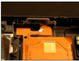
Verify the camera key's two alignment tabs are positioned in the back cover as shown.
