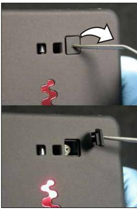
Obtain a new RF port plug and insert it into its opening in the back cover as shown.
