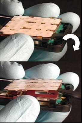
Rotate the dome foil assembly away from the system connector.
