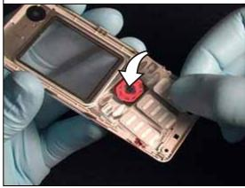
Press the keypad down around each of its four placement pins.
