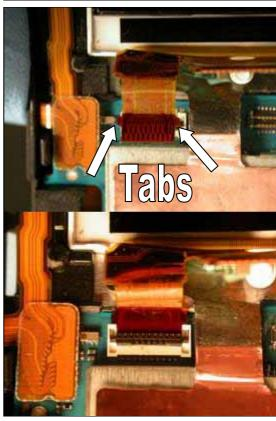
Insert the LCD flex film into its corresponding ZIF connector on the circuit board.
