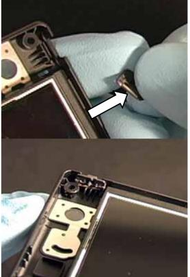
If the volume key fell out, make sure its spring is still attached. Then place it back into its slot in the back cover with the spring facing downward into the back cover.
