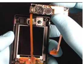
Insert the Walkman key end of the camera flex assembly first.
