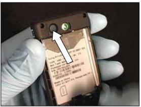
Press on the window for 10 seconds to make sure it bonds to the back cover.
