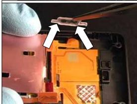
Work the camera key into its opening in the back cover.
