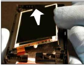
Lift the LCD out of the old back cover.
