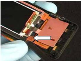
Insert the tip of a pair of tweezers in the hole in the camera flex assembly indicated.
