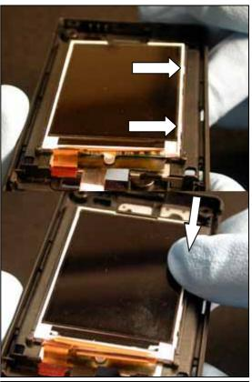
Make sure the LCD is fully seated and that there are no gaps along either side.
