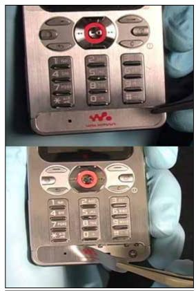
Clean off any remaining adhesive residue with alcohol and a lint free cloth.
