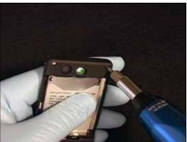
Slide one side of a pair of Style 2A tweezers under the cobrand label in the location shown and peel the co-brand plate off of the front cover.
