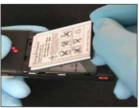
Rotate the battery down into its cavity. Make sure it is fully seated.
