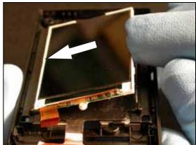
Rotate the LCD down into its cavity.
