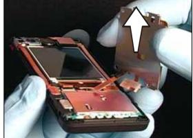
Pull the dome foil assembly straight up out of the phone. Make sure the camera switch portion of the dome foil assembly does not get damaged during this movement.
