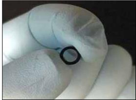
Insert the new camera window into its cavity in the back cover.
