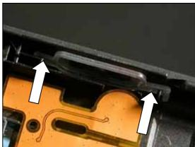
To remove the RF port plug from the old back cover, press on the inside surface of the plug until the plug pops out of its opening.
