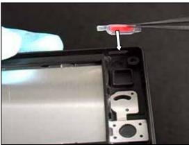
Verify the Walkman key's two alignment tabs are positioned in the back cover as shown.
