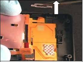
Obtain a new camera key and orient it so that the two curved corners indicated are towards the back cover.
