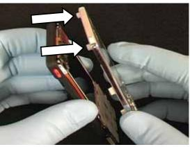
Squeeze the two covers together and inspect the outside seam of the phone. There should be no gaps around the seam.
