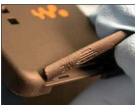
Locate the hole where the tab portion of the memory stick cover inserts through back cover.
