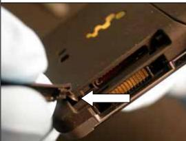
Pull the memory stick cover straight away from hole until the tab holding the cover to the phone comes free.
