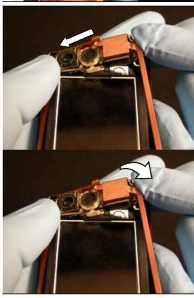
Then rotate the remainder of the camera flex assembly into its cavity in the back cover.
