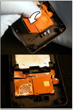
Insert the corner of a plectrum in the seam along one side of the LCD in the location shown.
