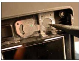
Obtain a new camera window and remove its protective backing.
