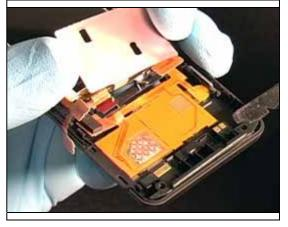
Slide the flat portion of a pry tool between the antenna and the back cover near the screw hole indicated.
