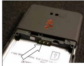
Using style 2A tweezers, place the end of the label that is adjacent to the battery contacts first. Then roll the rest of the label down onto the floor of the battery cavity.
