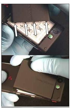
Rotate the battery cover down and snap it into place.
