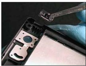
Insert the volume key into its slot in the new back cover with the spring oriented towards the back cover as shown.
