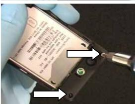
Install two rear screw plugs by inserting them into the rear screw cavities. Press on the rear screw plugs to make sure they seat fully.
