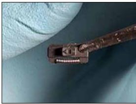
Insert the new volume key into its slot in the back cover with the spring towards the back cover as shown.
