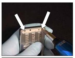
Insert the tip of a plectrum in the seam between the front and back covers in the location shown.
