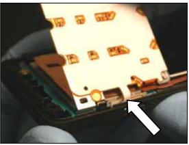
Rotate the dome foil assembly down over the circuit board so that that two alignment pins pass through the two holes at the top of the dome foil assembly as shown.
