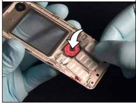
Press the keypad down around each of its four placement pins.
