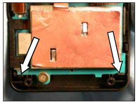
Lift the copper portion of the heat spreader up and fold it toward the LCD.
