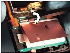
The LCD's flex connection is completely seated in the ZIF connector when the two tabs on the flex are against the ZIF connector.
