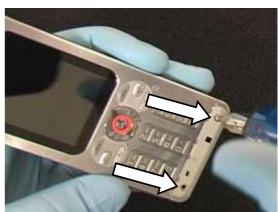
Install two screws in the back cover and tighten with a torque driver set to 20 N\*cm and a T6 bit.
