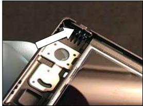
Verify that the Walkman key is in its slot in the back cover with the curved corners towards the frame as shown.
