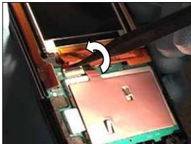
Using a nylon pointer, rotate the black retaining bar on the ZIF connector down over the LCD flex as shown.
