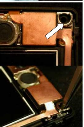
Rotate the tweezers away for the LCD. The camera flex assembly will lift from its cavity in the back cover.
