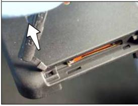
Press the memory stick cover's tab into its hole in the new back cover. Use a nylon pointer if needed.
