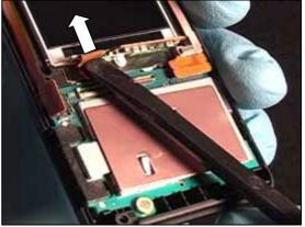
Use a nylon pointer to release the two latches indicated from the bottom edge of the circuit board.
