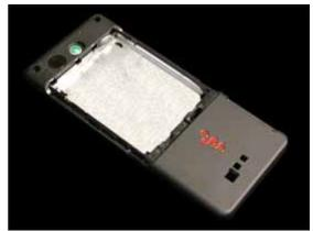
Obtain a new SIM flex film and remove the protective backing from the three areas of the SIM Flex indicated.
