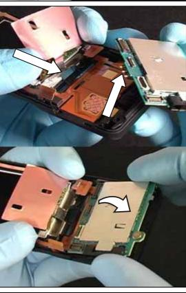
Rotate the circuit board down on the back cover.
