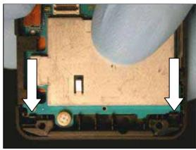
Fold the copper portion of the heat spreader down onto the circuit board's shield can. Make sure the shield can's two prongs go through the heat spreader.
