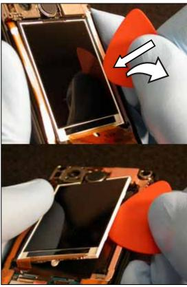
The LCD should pop free of its cavity in the back cover.
