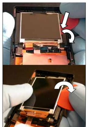
The LCD should pop free of its cavity in the back cover.
