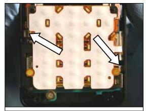
Using a pry tool, pry in the location shown to detach the adhesive holding the dome foil assembly to the circuit board.
