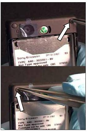
Use a torque driver and a T6 bit, remove the two rear screws.
