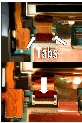
Using style 2A tweezers, insert the LCD flex film into its corresponding ZIF connector on the circuit board.
