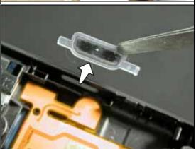
Orient the camera key so that the two curved corners indicated are towards the new back cover.
