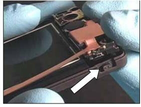
Make sure the new camera flex assembly is fully seated in back cover and that the volume key works properly.
