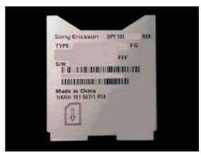
WHEN INSTALLING A NEW LABEL, BE VERY CAREFUL TO AVOID TOUCHING THE CONTACTS OF THE BATTERY CONNECTOR WITH THE ADHESIVE SIDE OF THE LABEL.
