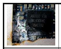
Corrosion components on the PCB.
