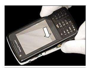
Use a front opening tool to disconnect the BtB connector.
