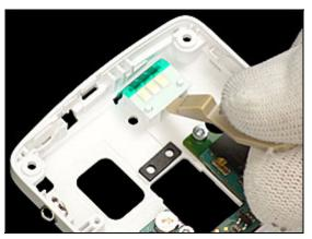
Use a tweezer to push the Antenna Flex through the hole
