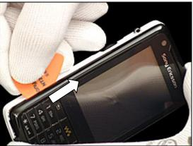
NOTE. Be cautious not to damage the 5 pole pin connector to Touch Panel on right side where the arrow point.
