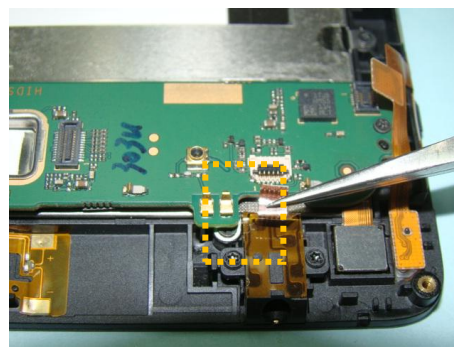
14. Install the FPC for the connector of the headset.
