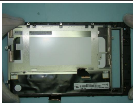
22. Remove the LCD from other cover A assembly.
