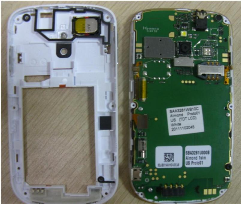
Step 4: Remove main antenna, speaker, T--card gate and side keys from furnished frame.
