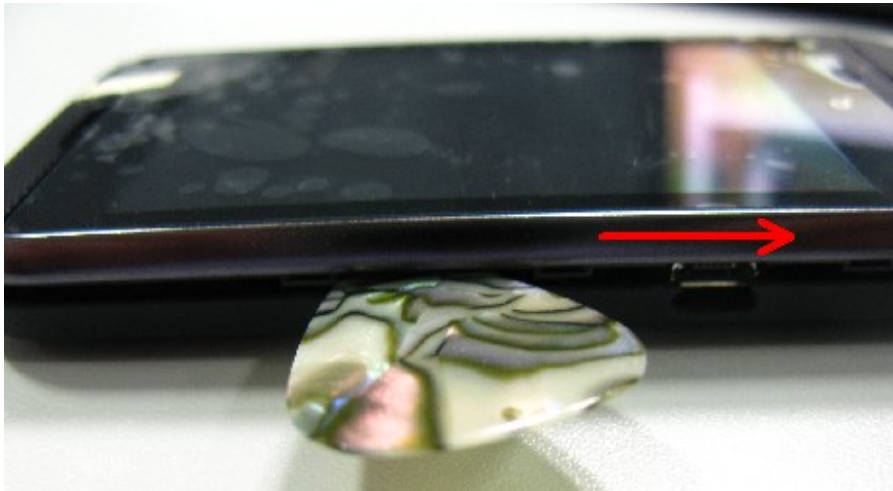
Step 3: Remove Touch Lens and LCD Module FPC connector by Plastic Flake
