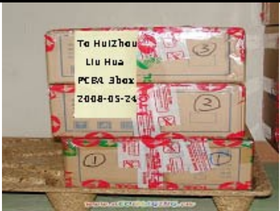
The packing box for PCBA should have marking sticker and well sealed by the tape with TCL logo
