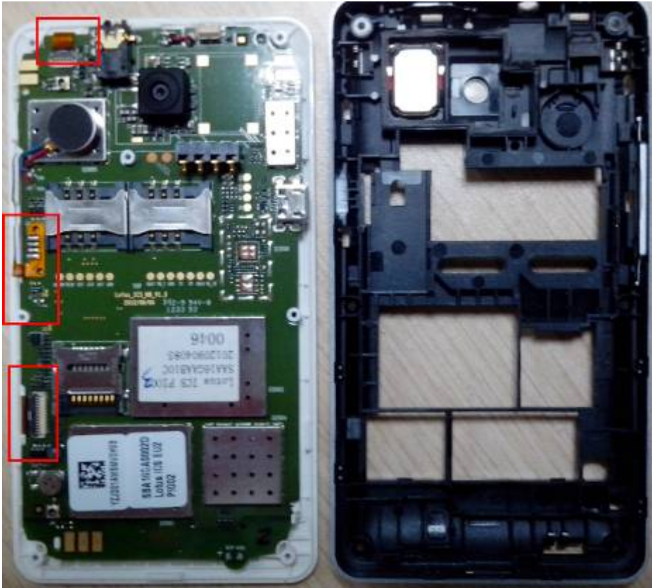
Step 3: Disconnect the connection everywhere as below picture shows
