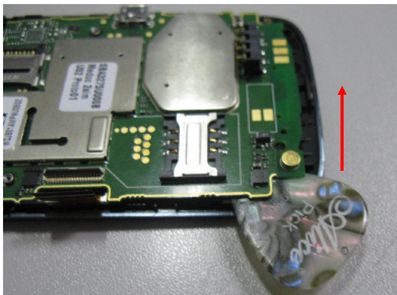
Step 4: Separate the Main PCBA from Furnished front casing
