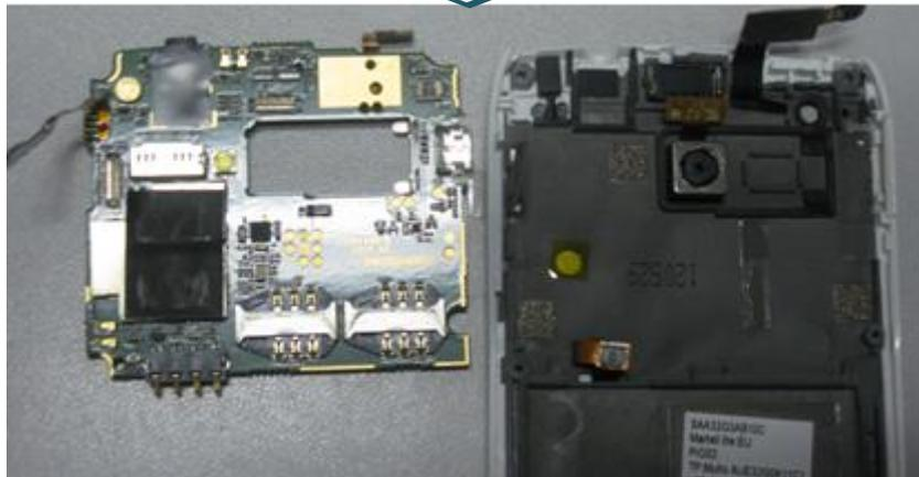
Step 12: Remove sub camera from main PCBA.
