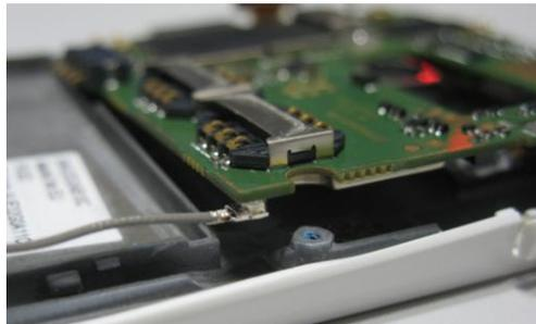
3). Remove the RF cable by using tweezers.
