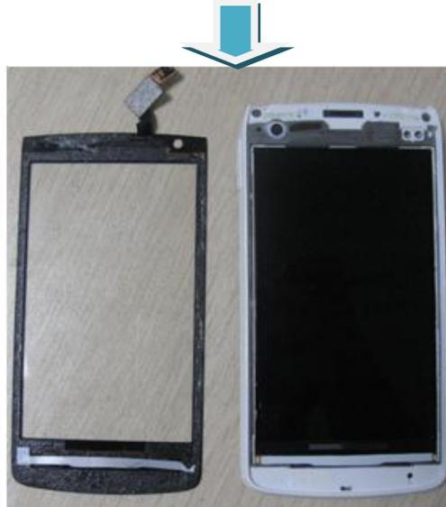
2). Please use hot wind gun to heat up LCD module around the four edges (Temperature: 100°C, Air Level: 3, Height:5-10mm, Time:<60s), and then use plastic flake to push the LCD model through the hole as below.
