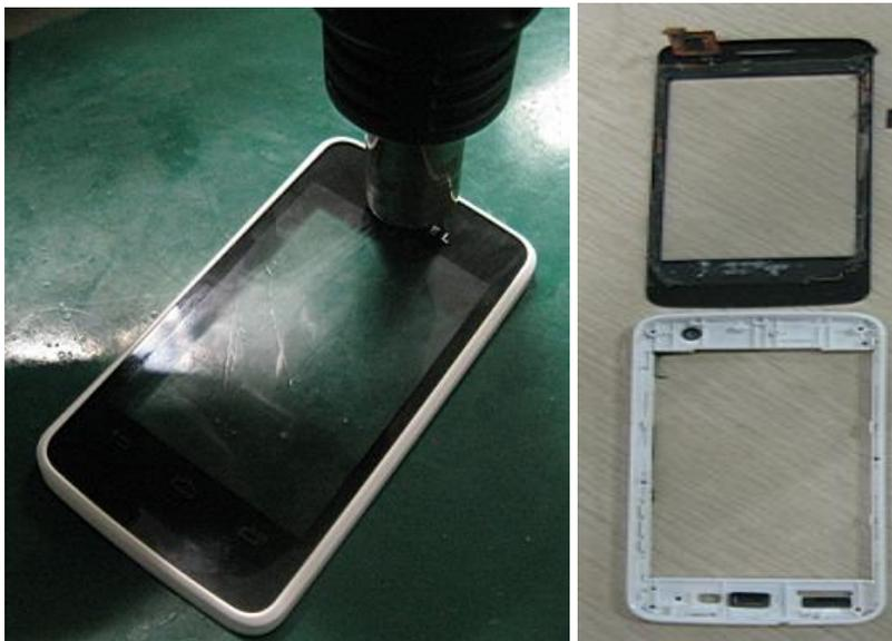
Note: if you repair the touch panel, then TP foam adhesive(below picture item1) and top/bottom adhesive for TP (below picture item2) are needed to be changed.
