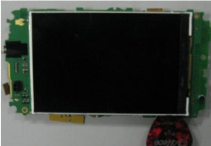
Step 9: Remove power key FPC and volume keypad FPC by using soldering iron (Temperature: Lead-free technology  $330^{\circ}\text{C} \pm 10^{\circ}\text{C}$ , time: 2~3 seconds).
