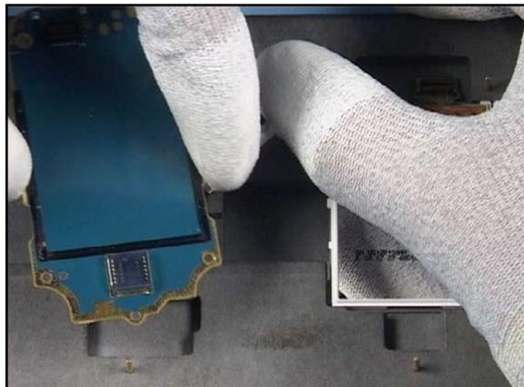
16. Release the lever and remove the PWB.
