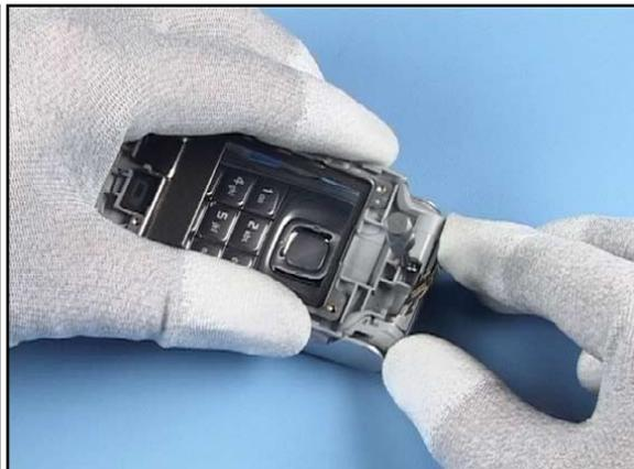
28. Now, the A-COVER UPPER ASSEMBLY can be removed easily. Mind the flex foil. The Hinge can be pulled out after the spring expanding carefully if needed.
