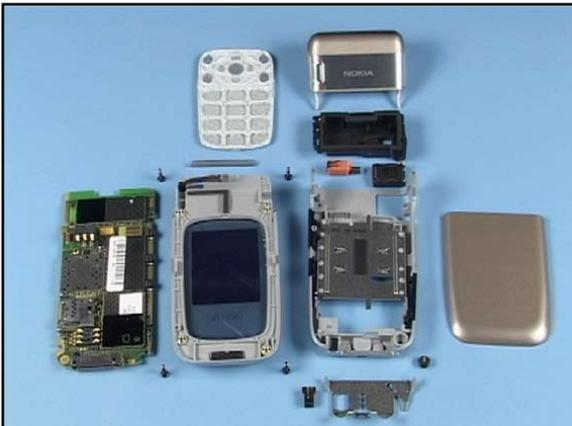
21. The disassembly procedure is now finished.
