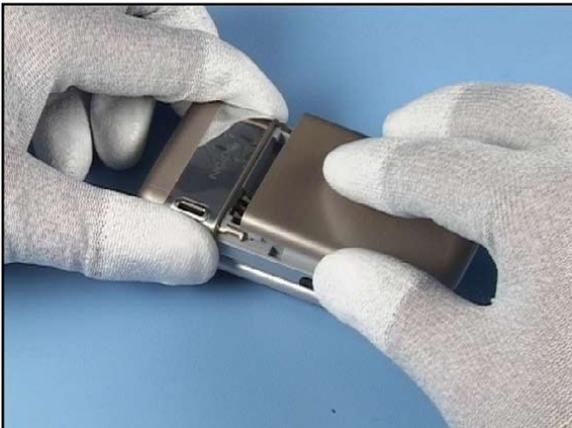
21. Complete the assembly with the BATTERY COVER.
