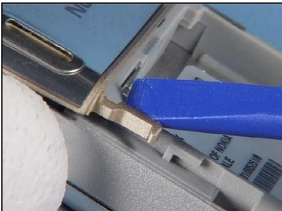
3. Unlock both latches of the ANTENNA CAP.
