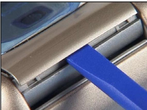
5. Use the SS-93 to pry open the B-COVER UPPER ASSEMBLY, starting at the top.
