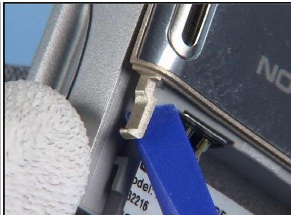
24. Unlock the clips of the ANTENNA CAP.
