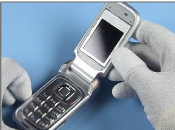
41. Open the unit, check the display and window for cleanness.
