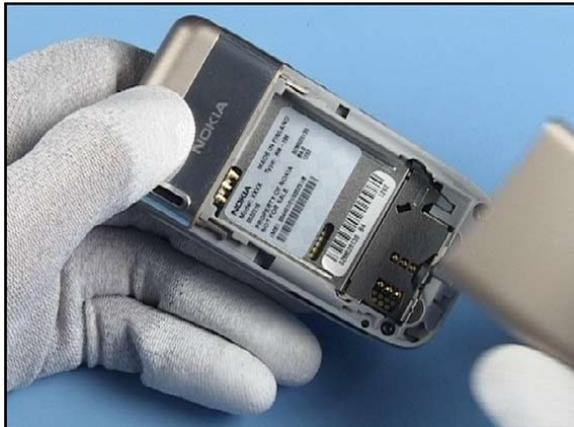
4. Remove the battery if it is still inserted.
