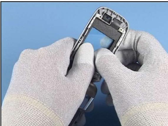
23. Push out the glued in LCD WINDOW.
