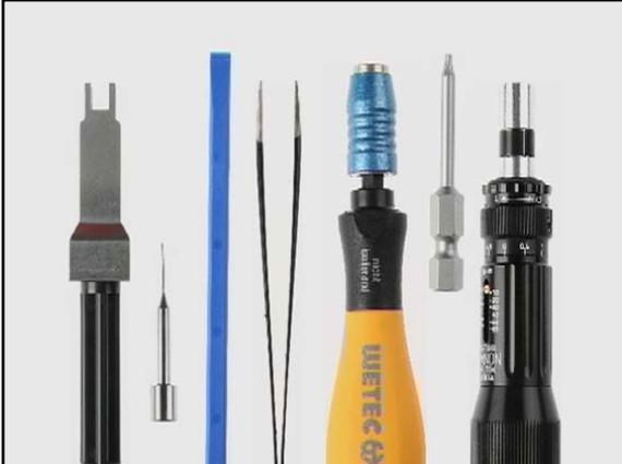
1. Needed tools: SS-88 camera removal tool, the SS-6, the SS-93, metal tweezers, a bit holder with a Torx Plus size 6 bit, a torque driver...
