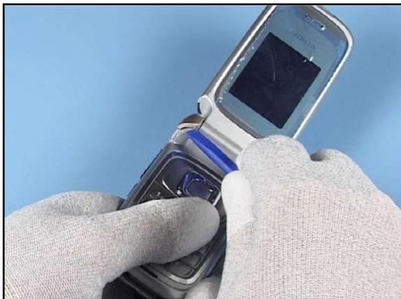
4. Open the assembly, release both upper clips of the ANTENNA CAP.
