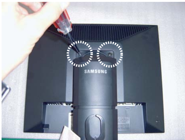
1. Place monitor face down on cushioned table. Remove 2 screws from the stand and remove front cover.
