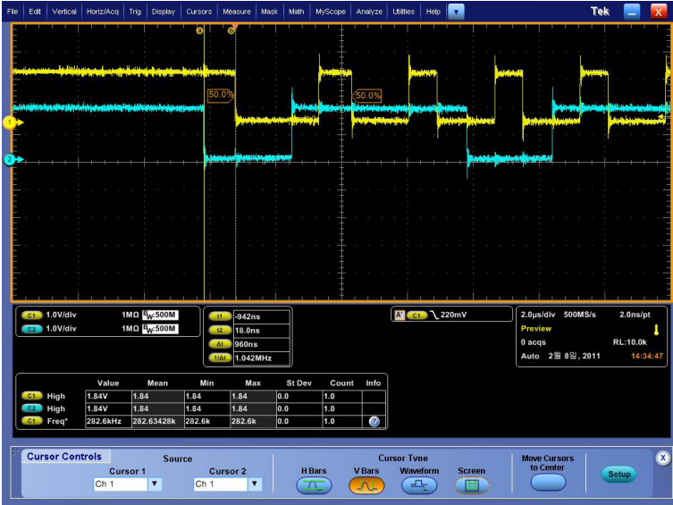
Graph 4.7.4. LCD Backlight Control Signal Waveform
