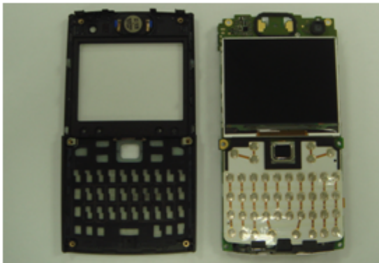
Separate Front Case and PCBA
