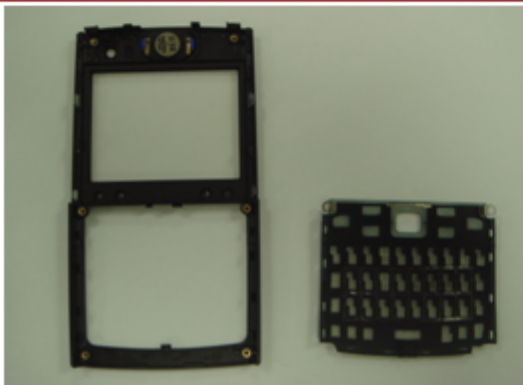
Separate Front Case and Keypad
