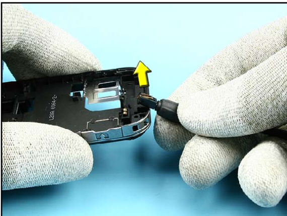
29. Remove the DC-JACK with a DC-plug.
