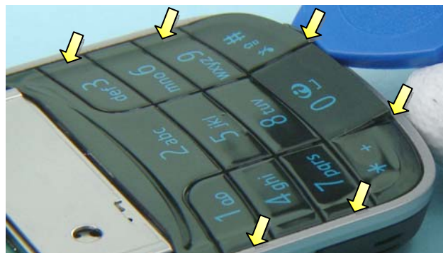
14) Release the six clips on the MAIN KEYMAT with the SRT-6.
