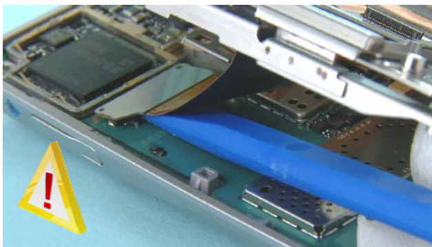
21) Carefully disconnect the MAIN FLEX from the engine board with the SS-93. The SLIDE MODULE can now be removed.
