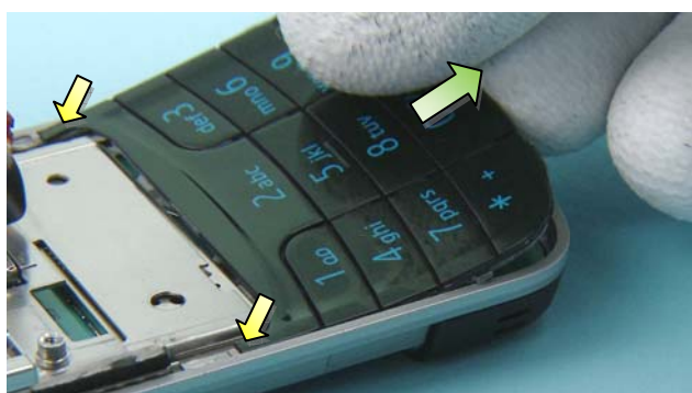
15) To release the two remaining clips, remove the KEYMAT in the direction shown.
