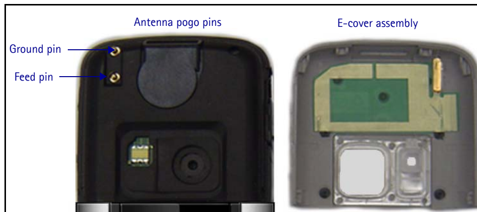
Figure 1: CDMA antenna on the E-cover
