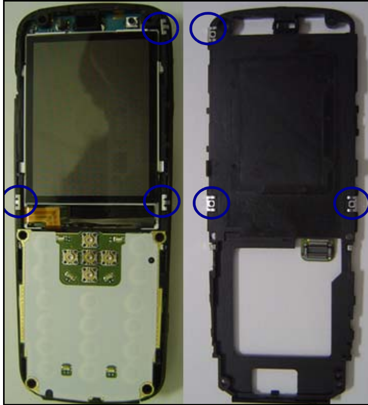
Figure 14: SAR reduction A-cover (left) and C-cover (right) grounding clip locations
