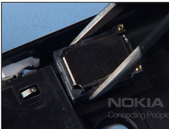
28. The IHF SPEAKER is not glued and can be removed easily.
