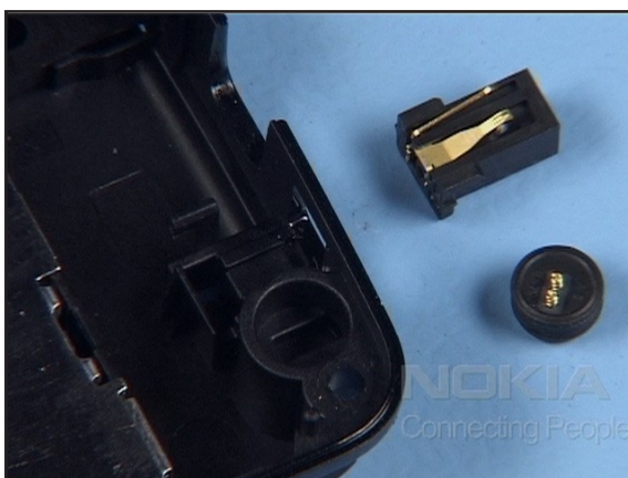
24. Remove the MICROPHONE and the DC JACK.
