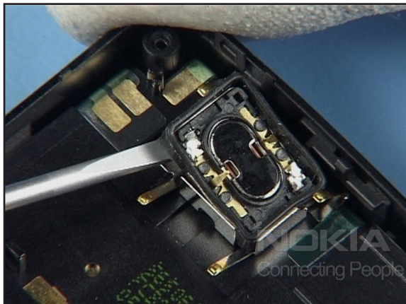
25. Carefully lever out the EARPIECE ASSEMBLY.
