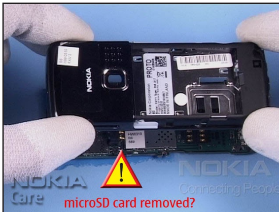
14. Note! Before removing the B-COVER, make sure that the micro SD card has been removed. Turn the assembly, lift up the B-COVER.
