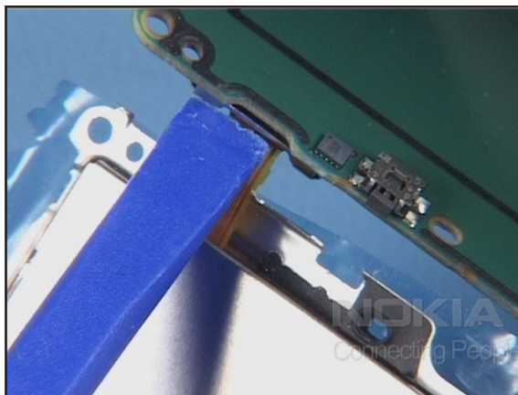
20. Carefully unlock the flex connector of the LCD MODULE.
