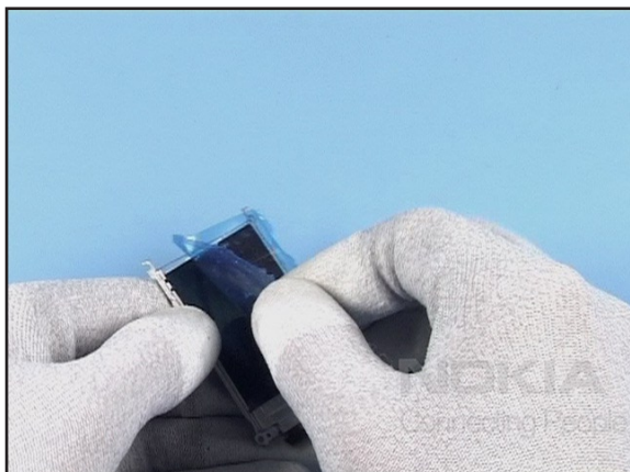
21. Peel up the protective film.
