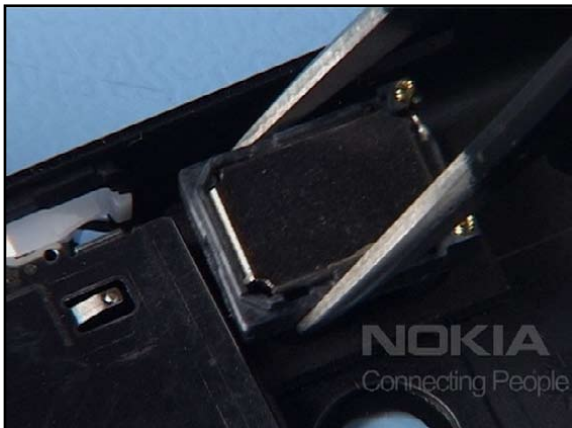
28. The IHF SPEAKER is not glued and can be removed easily.
