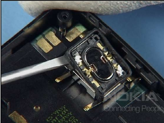
25. Carefully lever out the EARPIECE ASSEMBLY.
