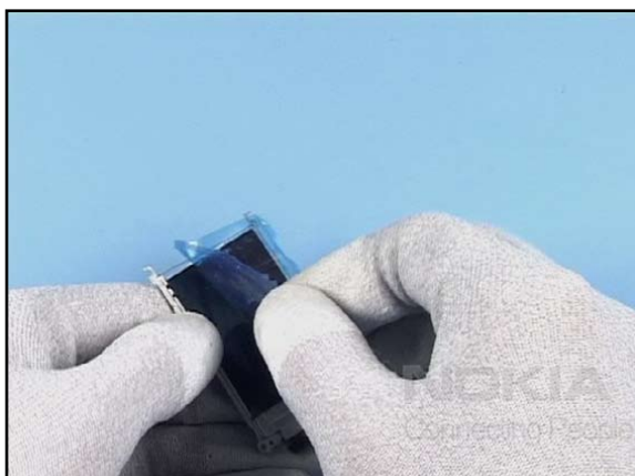
21. Peel up the protective film.
