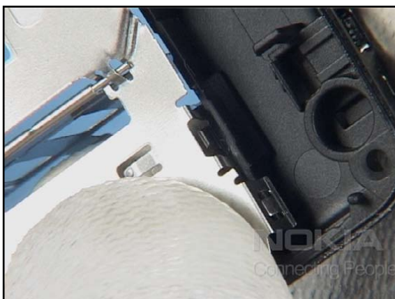
4. Carefully push all latches into their places.
