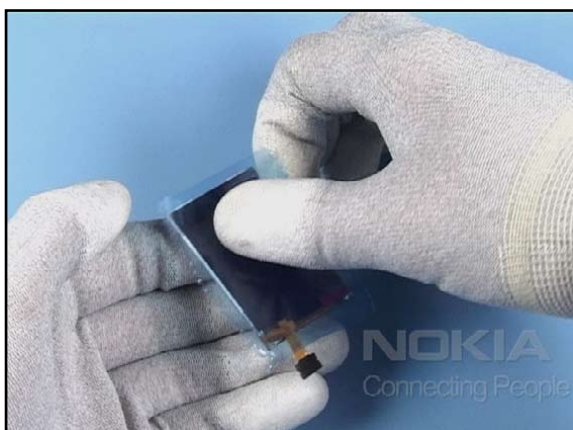
23. Cover the display with a film again.
