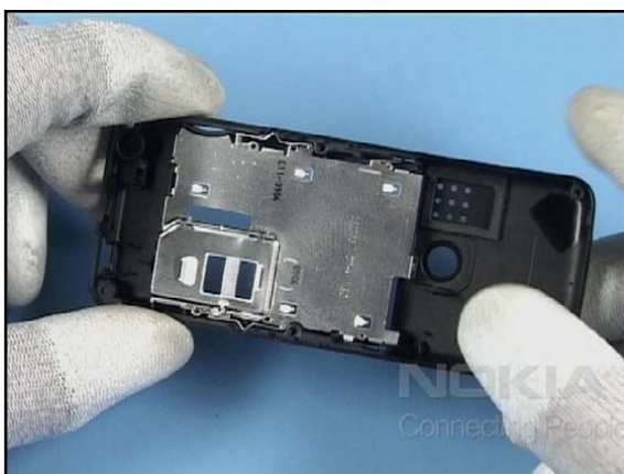
6. Check the correct positioning of all these latches.
