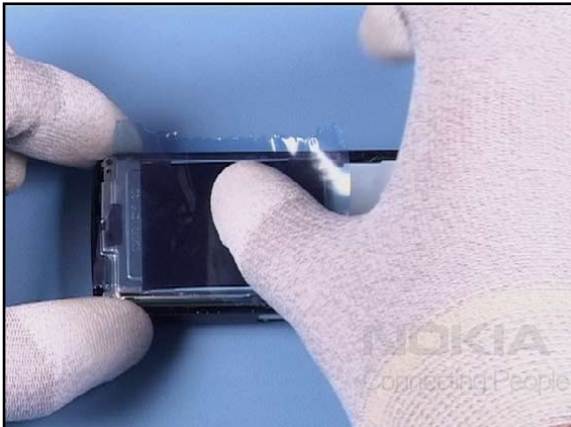
13. Cover the display with a film.
